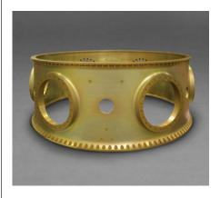
ESPA mounts to the standard NSSL (formerly EELV) interface bolt pattern (Atlas V, Falcon 9, Delta IV, OmegA, Vulcan, New Glenn) and is a drop-in component in the launch stack. Small payloads mount to ESPA ports featuring either a Ø15-inch bolt circle with 24 fasteners or a 4-point mount with pads at each corner of a 15-inch square; both of these interfaces have become small satellite standards.
