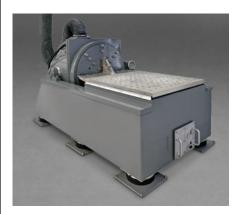
Moog provides end to end vibration test services with a system that is capable of replicating random, swept sine, shock (both classical and SRS) and arbitrary transient waveforms with temperature control and notched drive inputs. The system replicates base vibration levels consistent with environmental testing practices for space flight hardware and MIL Specification 810G. We offer the customer data reporting that
