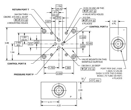
Null Adjust: Flow out of Control Port B will increase with clockwise rotation of null adjust screw (1/8 hex key).
