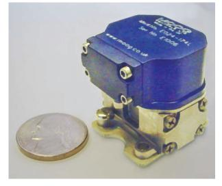
The EO24 servovalve weighs 92 g, is rated for 7.5-Ipm flow at 70 bar, with maximum pressure of 210 bar. On Formula One cars, it handles high-power applications such as shifting gears and actuating clutches.
