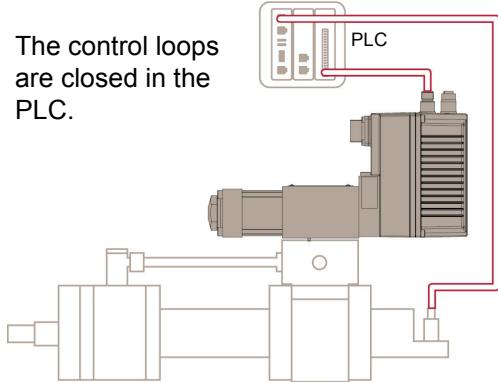
The control loops are closed in the PLC.
