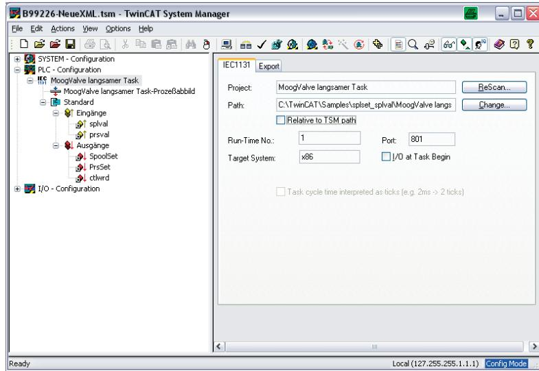
Figure 36: PLC configuration with PLC application parameters
