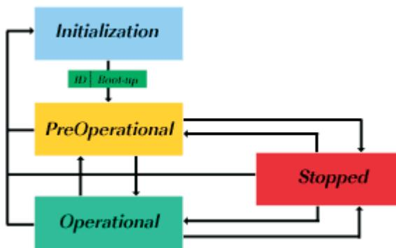
Figure 6: Network State Machine (NMT)
