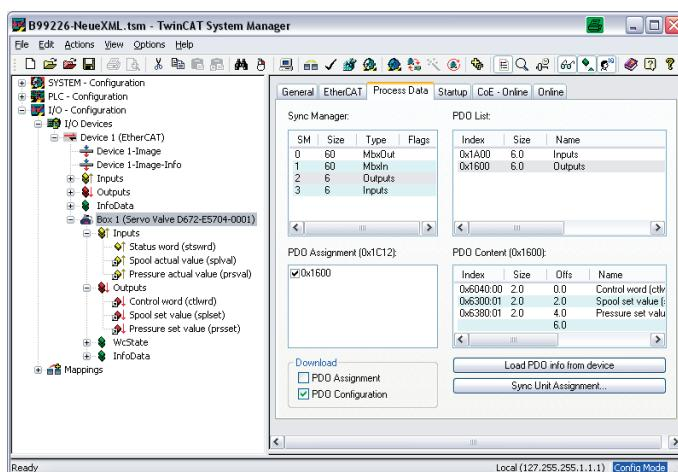
Figure 33: Process Data Objects (PDO) mapping
