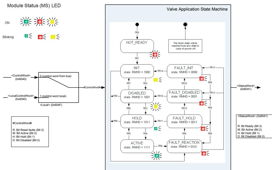
Figure 7: Device State Machine (DSM)
