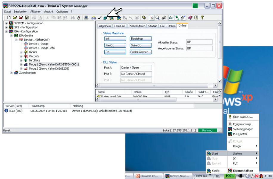
Figure 39: Activating the network configuration
