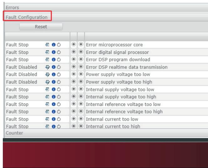
Figure 22: MoVaPuCo fault configuration
