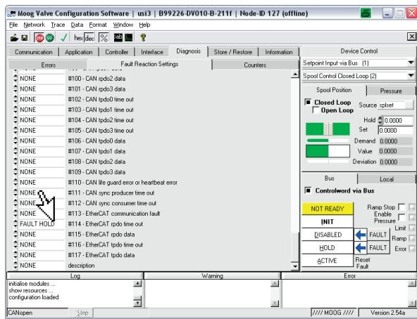
Figure 45: Configuring the fault reaction
