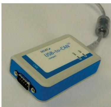
Figure 24: USB to CAN adapter
