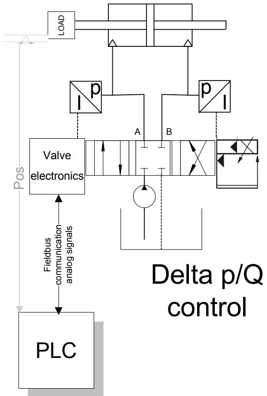
Figure 18:  $\Delta p$  control principle
