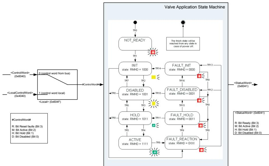
Figure 23: Device State Machine fault states
