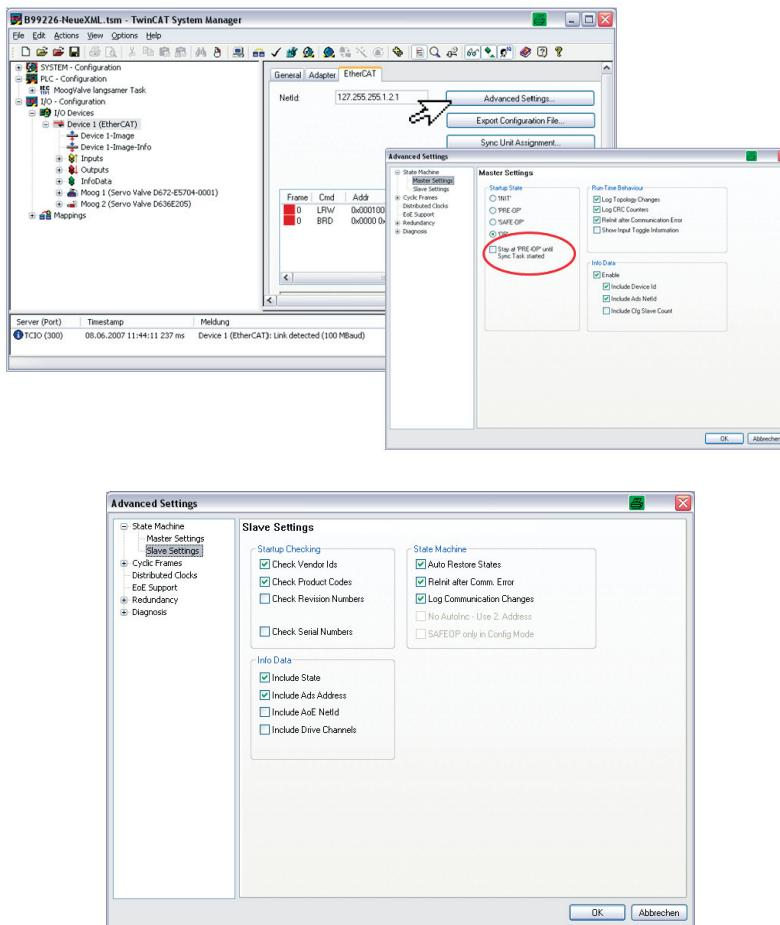
Figure 38: Setting the network startup options
