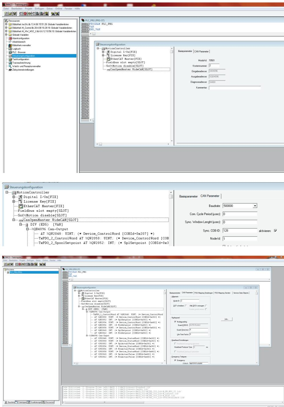
Figure 28: CANopen network with Moog MSC II configuration
