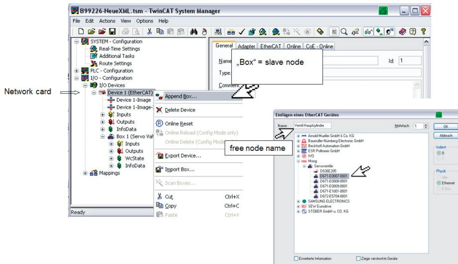
Figure 31: Inserting a network card
