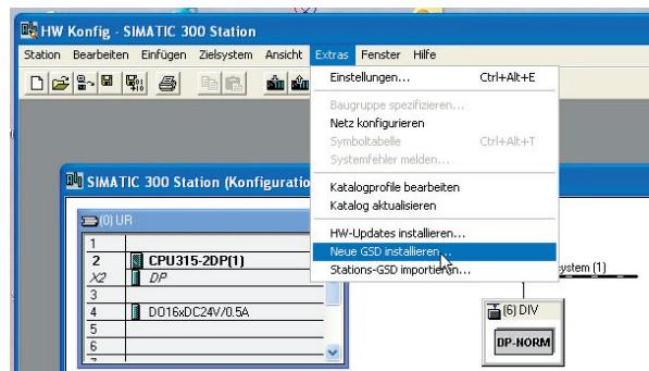
Figure 50: Installing slave interface description file (GSD)
