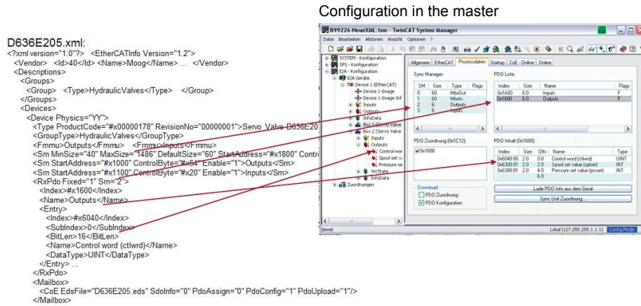
XML file is read during startup of the TwinCAT System Manager
