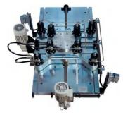
Hydraulic springs and clamps are available to release/tighten the moving plates. Automated control is available with PC and remote control options.
