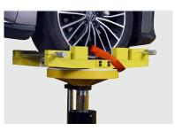
stiffness needed for squeak and rattle applications. Positioning of the restraints (both lateral and longitudinal) is manual and does not interfere with the usable tire contact patch area.
