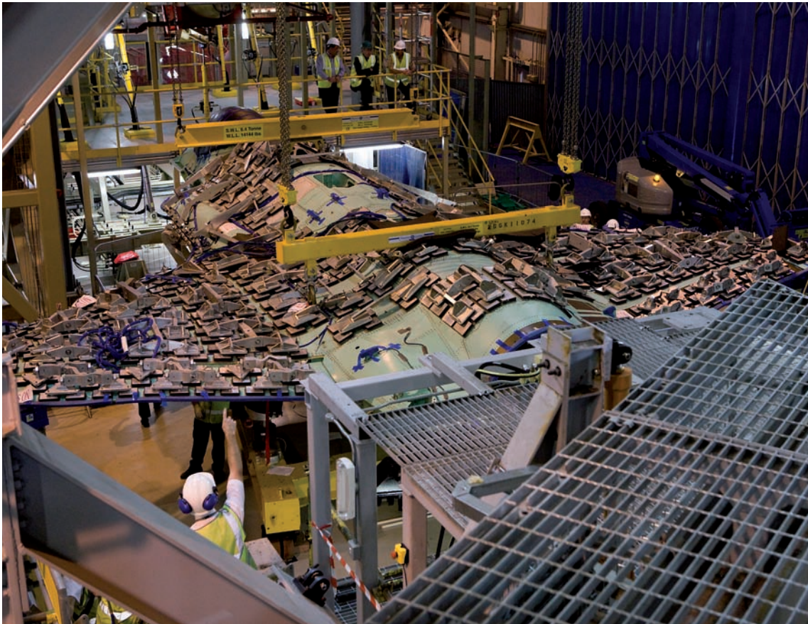
The fully padded airframe AJ-1 ready to be lifted into the test fixture
