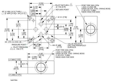
$\triangle$  External pilot supply and return ports shown for reference only. Manifold P/N 22236AM3 Is not provided with ports.
