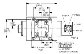
The mounting Manifold must conform to ISO 10372-06-05-0-92.
