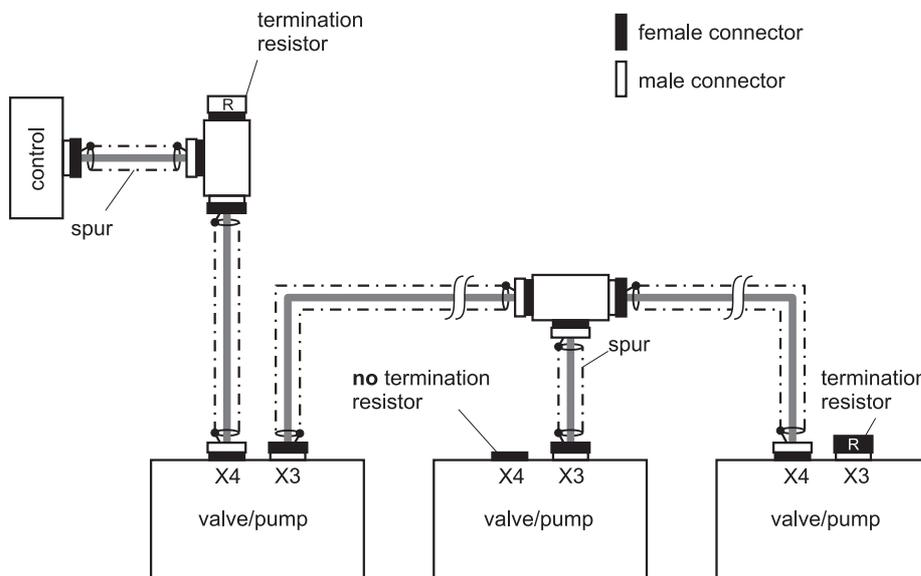
**Wiring diagram of
