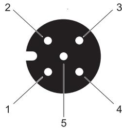
External LVDT connector X8 (M12, 5-pin)
