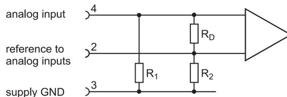
Figure 13: Equivalent circuit diagram of analog input
