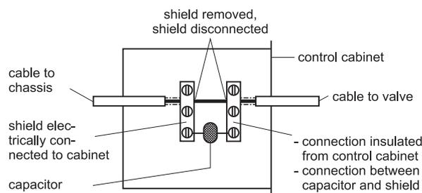
Figure 23: Connecting the insulated shielding to the control cabinet's wall (detail A from Figure 20)
