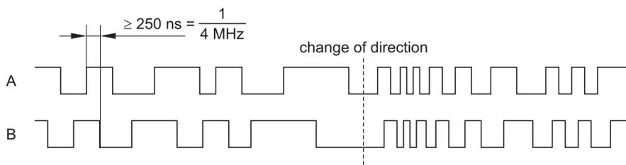
Figure 31: Incremental transducer signals A and B with reversal point and speed variation
