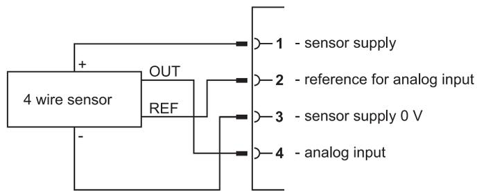
**Wiring the 4-wire transducer**
