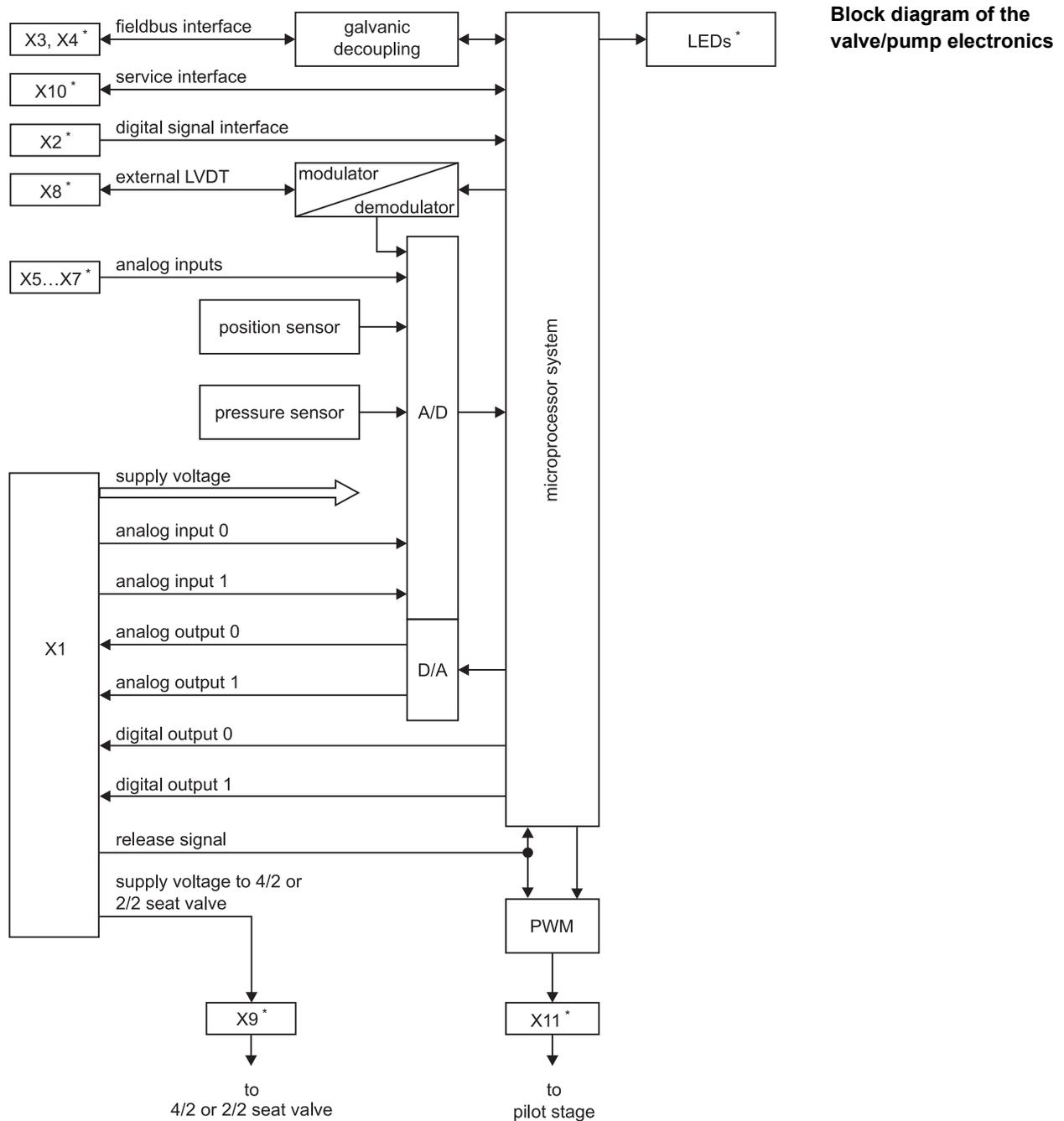
Figure 1: Block diagram of the valve/pump electronics
