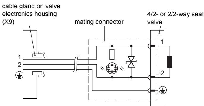
Block diagram of the plug connection of the 4/2- or 2/2-way seat valve (with free-wheeling and light emitting diode)
