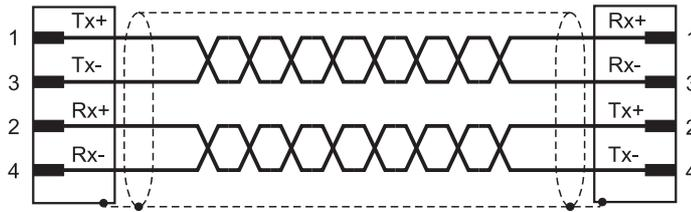
**Pin assignment for the EtherCAT® cable**
