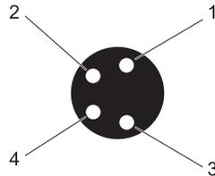
**Analog input connectors X5, X6 and X7 (M8, 4-pin)**
