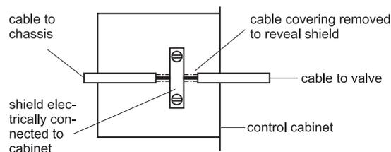
Figure 21: Connecting the shield to the control cabinet's wall (detail A from Figure 20)
