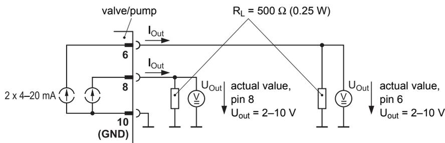
Figure 29: Circuit for converting the actual value output signals  $I_{out}$  (for valves with 11+PE-pin connector X1)
