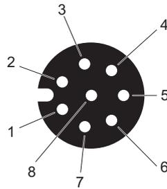
View of SSI transducer connector X2
