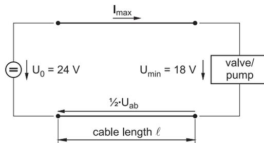
Figure 24: Voltage drop on the supply cable
