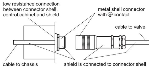
Figure 22: Connecting the cable shield via connector to the control cabinet's wall (detail A from Figure 20)
