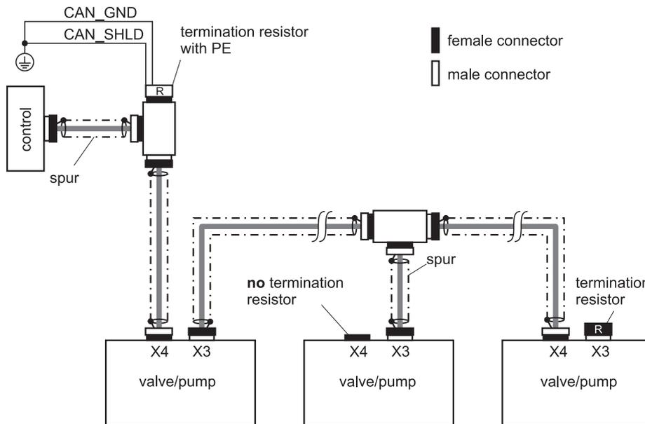
Figure 34: CAN wiring diagram
