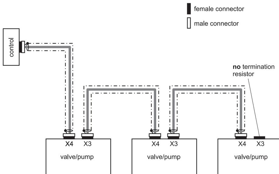
Figure 38: EtherCAT® wiring diagram
