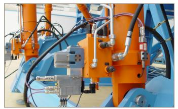
Figure 5: Cylinder with Moog D671 series valve Source: Courtesy of Airbus Bremen
