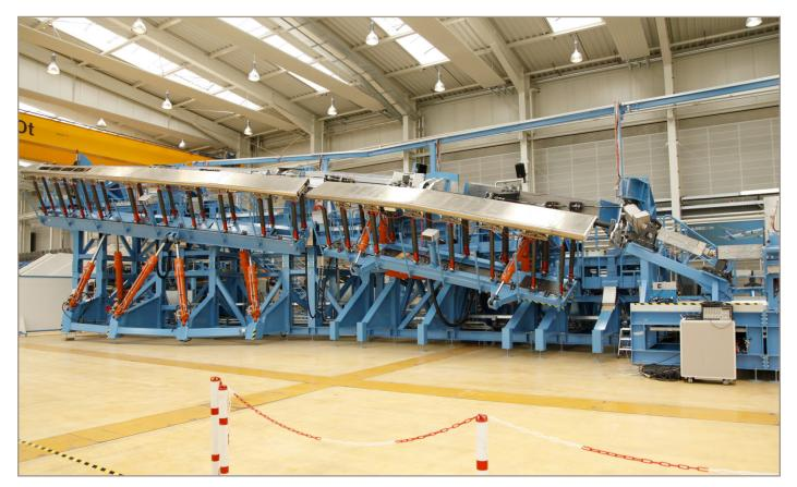
Figure 1: Landing flap test system Source: Courtesy of Airbus Bremen
