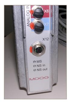
Figure 6: New analog input for sensors with resistive bridges
