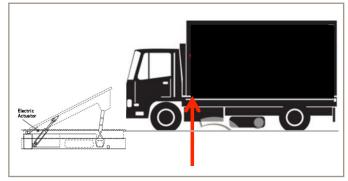
Figure 3: Penetration Measuring Location (P-Rating)
