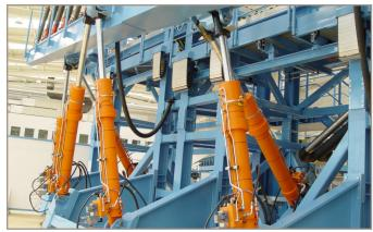
Figure 4: Metal framework with hydraulic cylinders Source: Courtesy of Airbus Bremen
