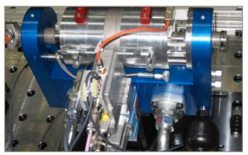
Figure 7: Moog Servo Valve with rotary drive during the test phase
