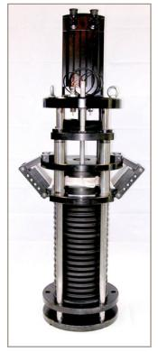
This arrangement uses a conventional fail-safe spring override to power the Anti-Surge Valve to the 'fully open' system in the event of a system problem. However, the novel part of the design is a 'toggle' mechanism which holds the spring in its fully compressed position during normal operation. This toggle is held in position by a mechanical toggle, latched by a lowpower electrical solenoid. In the event of a system failure the solenoid is de-
