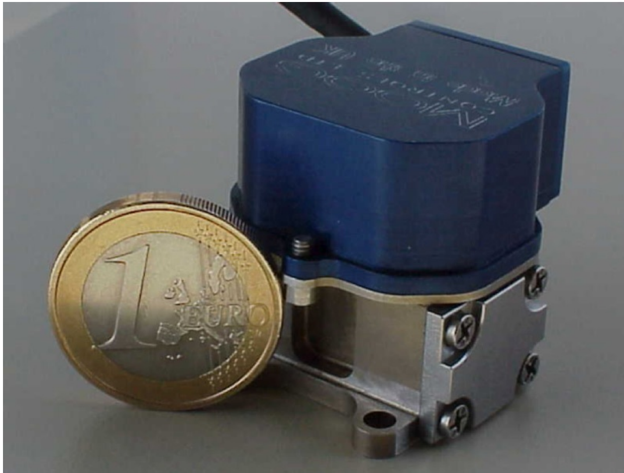
Figure 2: Moog 24 Series Servo Valve illustrates degree of miniaturization required by F1
