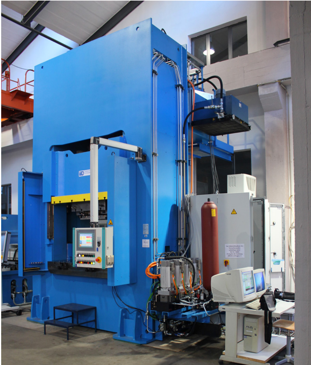
Figure 3: Deep drawing press using EHA for the die cushion axis. Source: Dresden University
