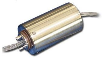
The FO300 is a prism based multichannel fiber-optic rotary ioint (FORJ). It is a passive and bidirectional device which can be used as a standalone device or easily integrated into a rotary assembly, enabling transfer of high data rate optical signals across a rotating interface.
