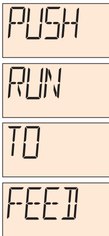
Figure 3-7 PUSH RUN TO FEED Alarm
