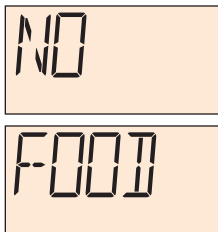
Figure 3-6 NO FOOD Alarm
