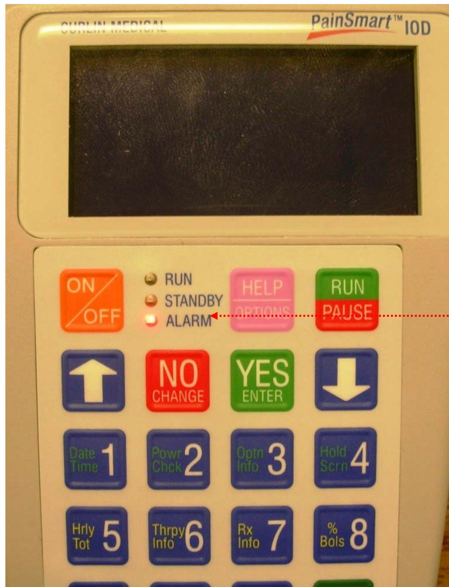
Connect an energized AC Adaptor (340-2004 / 340-2022) to the pump. (Connect the AC Adaptor's blue cable connector to the POWER connector on the bottom of the pump). Turn the pump ON. Resume the therapy and confirm that the infusion continues (observing the Vol INF) where it stopped due to Auxiliary Alarm occurrence.
