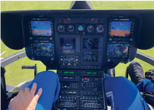
The Genesys Avionics Suite™ designed for the Airbus EC-145e helicopter features four IDU-450 displays in a dual-sided PFD/MFD format, dual redundant ADAHRS, Dual GPS/FMS, and IFR certified Genesys GRC™ Rotorcraft Autopilot & Stability Augmentation System (SAS).
