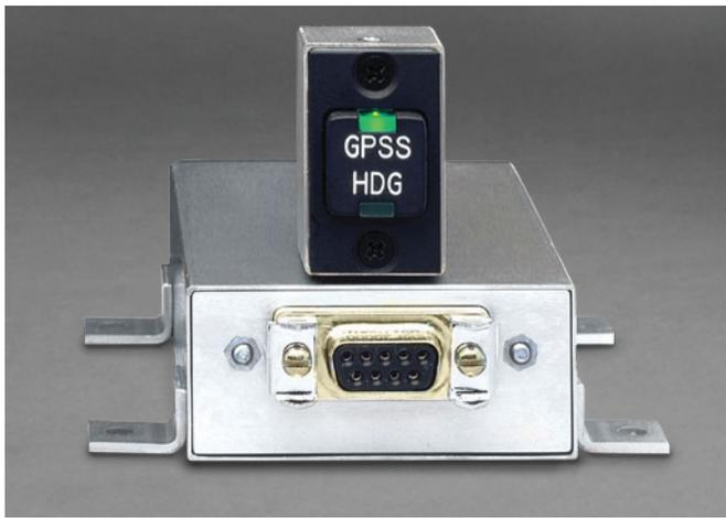
To save valuable panel space, the GPSS converter is configured as a separate panel-mounted switch and remotely-mounted control box. The control switch is 1.32 x .82", and projects only 1" behind the panel (plus cable connector).
