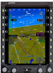
Genesys' 3D Synthetic Vision and Highway-In-The-Sky flight navigation enhances safety and reduces pilot workload plus provides precision aircraft operations including RNP and LPV approaches.
