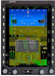
Genesys' IDU EFIS suites feature a variety of PFD and MFD formats that can be configured to show flight instruments, moving map, HSI, flight planner, traffic, terrain, weather radar, datalink, video, radio/audio management, and engine displays.
