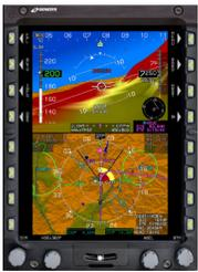
Genesys' patented OASIS (Open Architecture System Integration Symbology) software allows easy customization and display of engine information and CAS messages.
