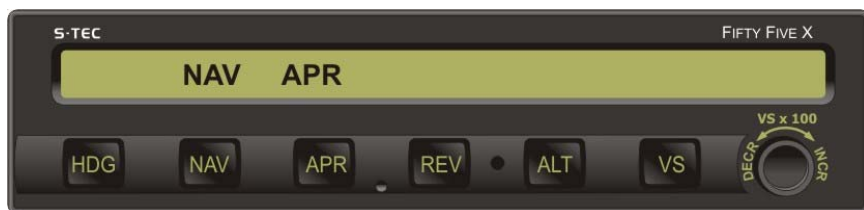
Fig. 3-29. AP Display, NAV APR Mode Engaged, Track VOR Front Course Inbound
