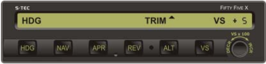
a. TRIM UP in Progress
