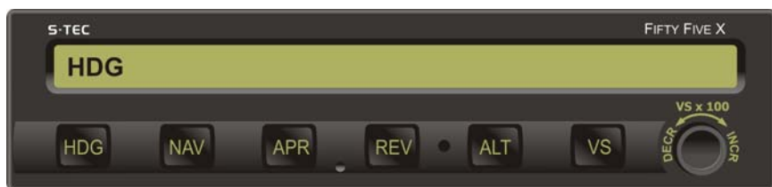
Fig. 2-6. AP Display, HDG Mode Engaged (Pre-Flight)
