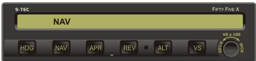
Fig. 3-2. AP Display, NAV Mode Engaged
