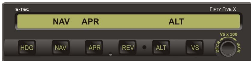
Fig. 3-17. AP Display, NAV APR and ALT HOLD Modes Engaged
