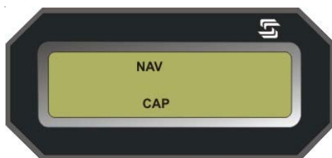
Fig. 3-3. Remote Annunciator Display, NAV Mode Engaged, CAP Condition
