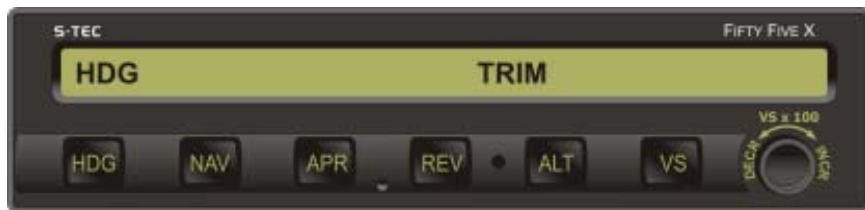
Fig. 3-16. AP Display, Manual Electric Trim in Progress
