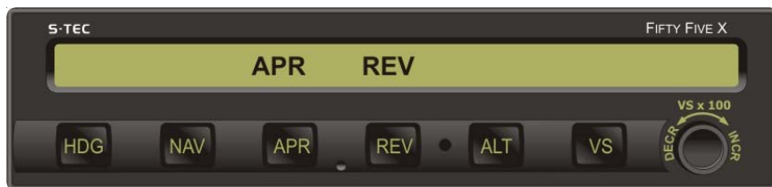
Fig. 3-25. AP Display, REV APR Mode Engaged, Track LOC Back Course Inbound
