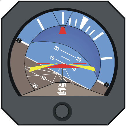
Fig. 3-39. FD Display, FD/AP Mode Engaged
