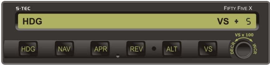
Fig. 3-12. AP Display, HDG and VS Modes Engaged
