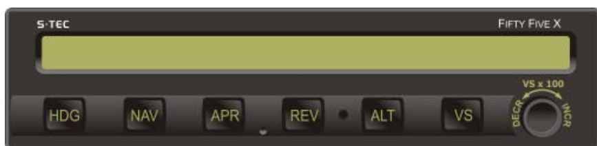
Fig. 2-5. AP Display, Turn Coordinator Failure
