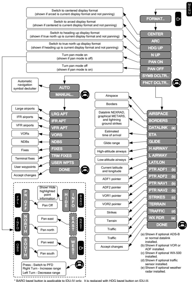
**Figure 5-98: Flowchart, MFD ND Screen Format (FORMAT) Menu**
