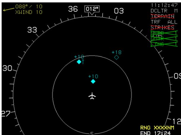
**Figure 8-60: ND Page during ADC and GPS Failure**
