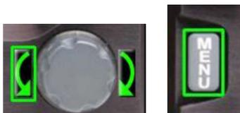
**Figure 8-12: Selection of Encoders and Buttons, Illustration of Counter-Clockwise and Clockwise Encoder Rotations**
