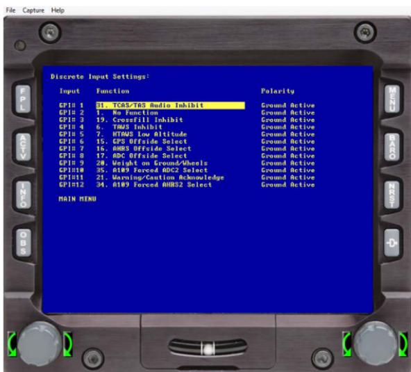
**Figure 8-20: Default Discrete Input Settings in Limits Editor**
