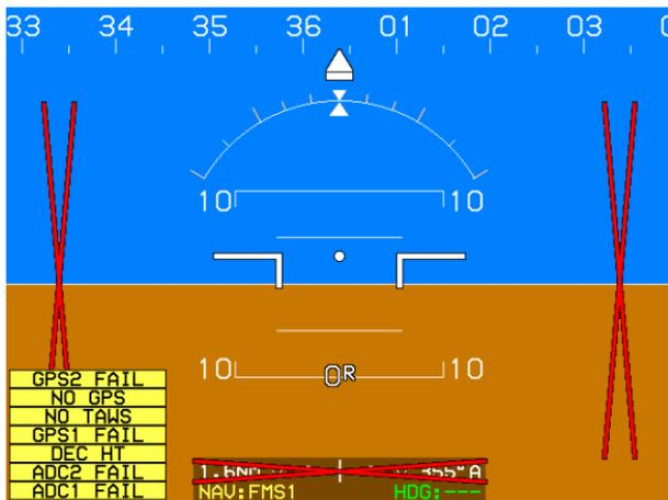
**Figure 8-59: PFD Page during ADC and GPS Failure**
