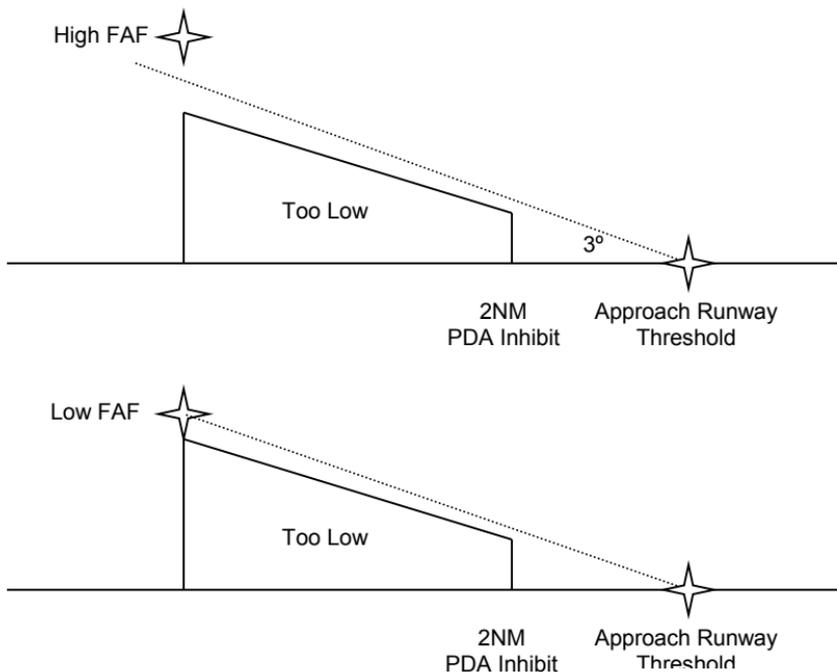
**Figure 8-38: PDA Alert Threshold**
