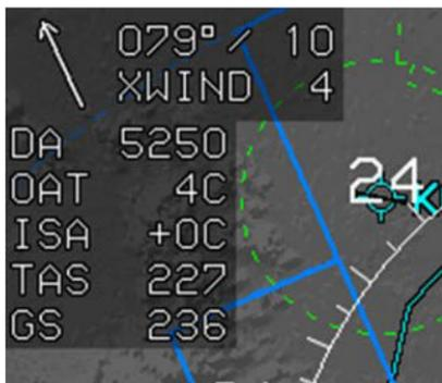
The aircraft's speed over the ground, in nautical miles per hour, is displayed in the upper left corner below the true airspeed. Groundspeed is based on GPS data.
