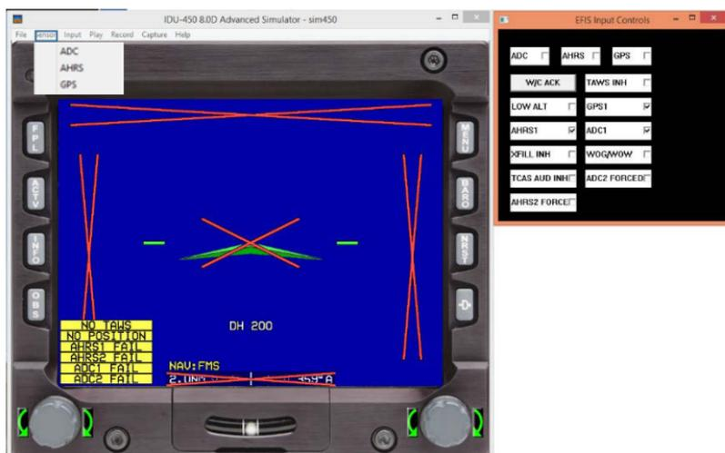
**Figure 8-19: EFIS Training Tool with All Sensors Failed**
