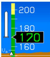
The Speed Trend Indicator is presented as a dynamic pointer that grows out of a fixed datum in correspondence with changes in horizontal velocity.
