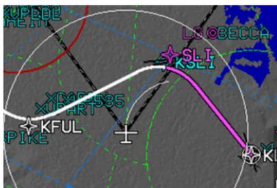
Route waypoints are displayed as four-point stars. The active waypoint is magenta; prior and subsequent waypoints in the route are white. Fly-over waypoints are enclosed in a circle, while fly-by waypoints are not. The identifier associated with each waypoint is shown next to the star in the same color. SLI is an example of a fly-by waypoint.
