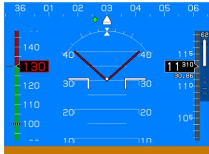
Rotorcraft in Basic mode pitching past  $\pm 30^\circ$ , the SVS mode reappears for best attitude recovery to level flight.
