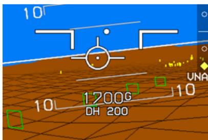
The altitude above ground level is displayed directly below the flight path marker or expanded waterline any time the indication is below the maximum height configured during system installation. AGL altitude is driven by the AGL altitude source being used for TAWS.
