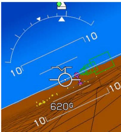
The PFD has a single width white pitch scale and horizon line that rotate in conjunction with the background according to the aircraft's roll angle. The pitch scale has increments every 5° with major increments and pitch scale labels every 10°. Pointer bars at the ends of each major increment indicate the direction to the horizon.
