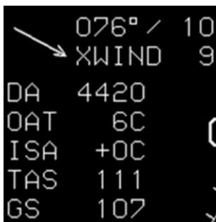
**Figure 4-22: Air Data and Groundspeed**
