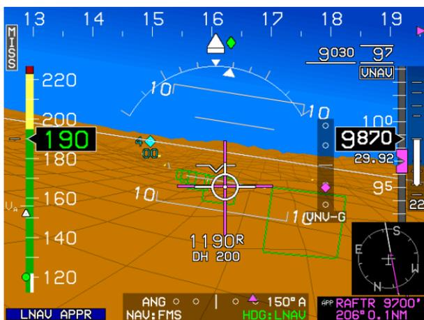
**Figure 3-30: Artificial Horizon and Actual Horizon, in Mountainous Terrain**
