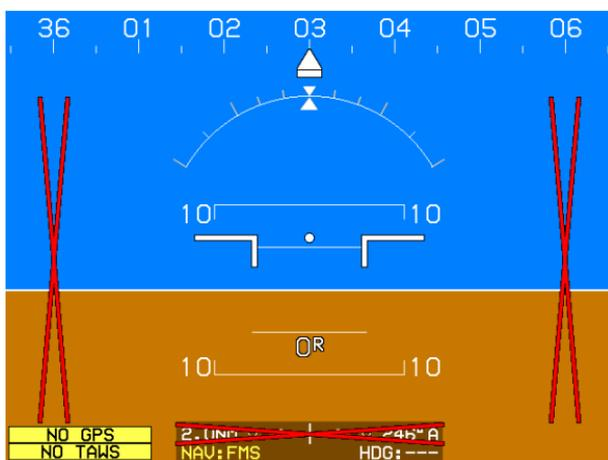
Figure 4-60: PFD Page during ADC and GPS Failure
