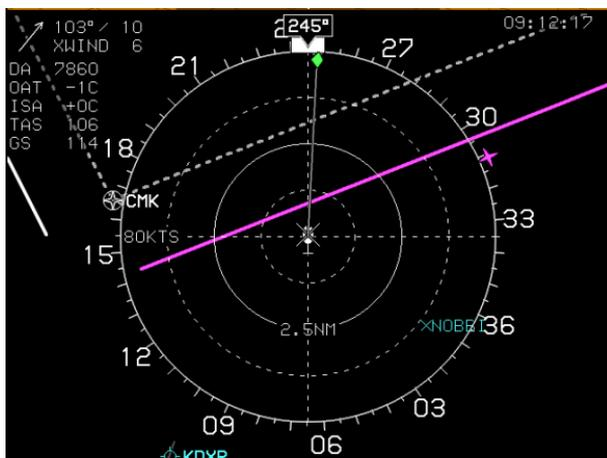
**Figure 4-19: Hover Vector Parallel Track - ND (Hover Vector Active Flight Plan Path/Parallel Course)**
