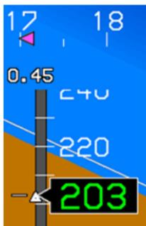
The Mach number is shown as an installation option above the airspeed tape on the airspeed indicator. It is automatically removed below Mach 0.45.
