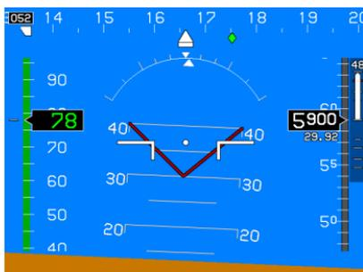
The FPM is automatically removed during the UAR mode and when inhibited if that feature is enabled.
