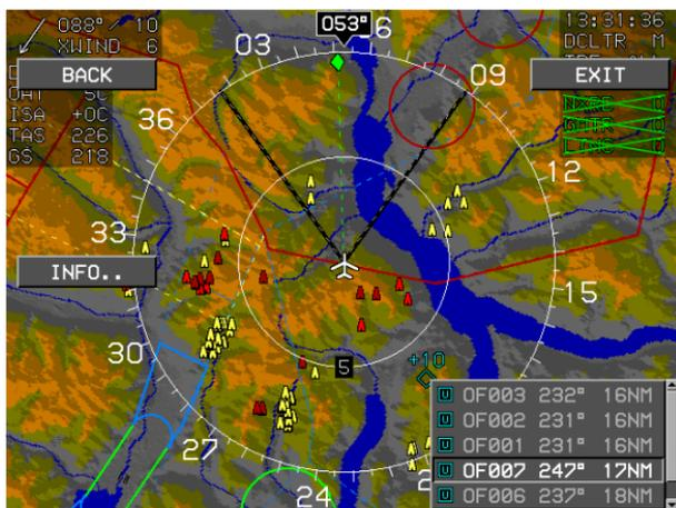
**Figure 5-109: Bearing and Distance from Original Position**
