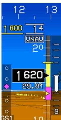
The altitude setting is indicated above the altitude tape. A line immediately below it identifies a minimum altitude value. Minimum altitudes may be set in 10-foot increments. In addition to setting minimum altitudes for non-precision approaches, a decision height may be chosen. This example shows a Minimum Altitude Setting of 1,800 ft. See Section 5 Menu Functions and Step-by-Step Procedures.
