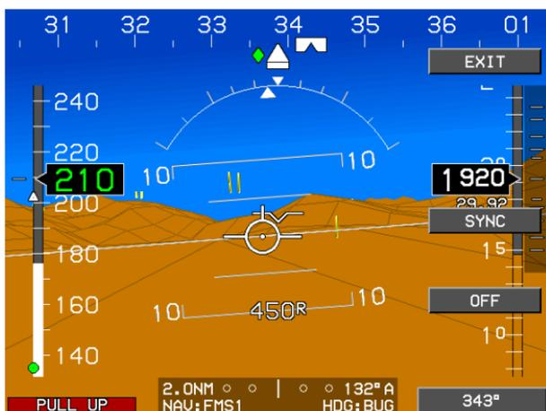
**Figure 3-55: Position of Flight Path Marker**
