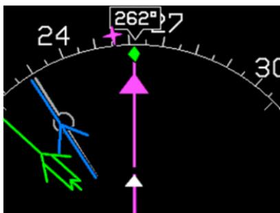
The bearing to the waypoint is indicated on the directional scale by a magenta star, which is the same symbol used for waypoints on the moving map and PFD directional scale.
