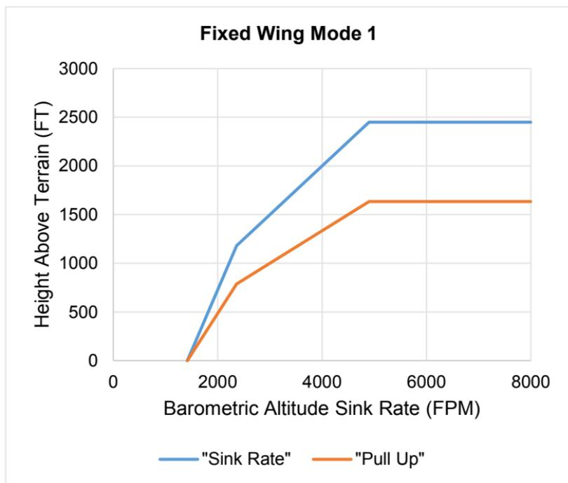
**Figure 8-39: Fixed Wing GPWS Mode 1**
