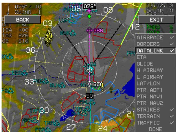
Figure 5-112: Datalink-Show/Hide Terrain (Moving Map)
