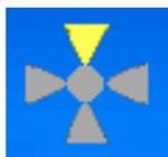
If commanded and controlled by the AFCS, the Cyclic Cue is displayed in the upper left of the PFD. The center circle is either gray or green as commanded by the AFCS. The outer triangles are either gray or amber (yellow) as commanded by the AFCS. (See 9.1.11.)
