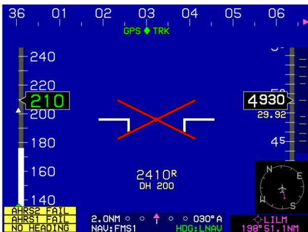
**Figure 8-57: PFD Page during AHRS Failure**
