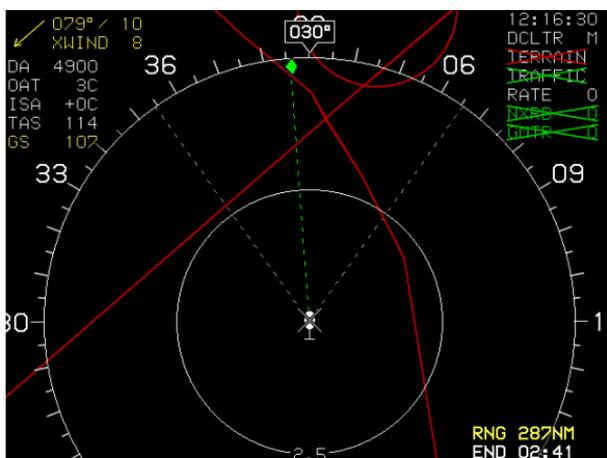
Figure 4-55: ND Page during GPS Failure
