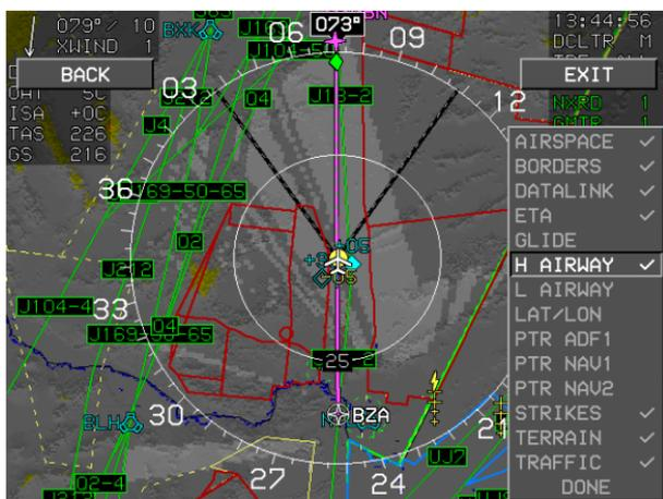
Figure 5-114: H Airway-Show I Hide Terrain (Moving Map)
