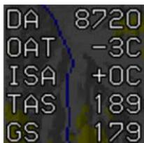
True airspeed (TAS) is displayed in the upper left corner of the display between ISA Temperature and groundspeed (GS). True airspeed is measured in knots and is corrected for altitude, temperature, and compressibility due to aerodynamic heating.
