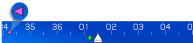
**Figure 3-14: Displaced Bearing to Waypoint Symbol**
