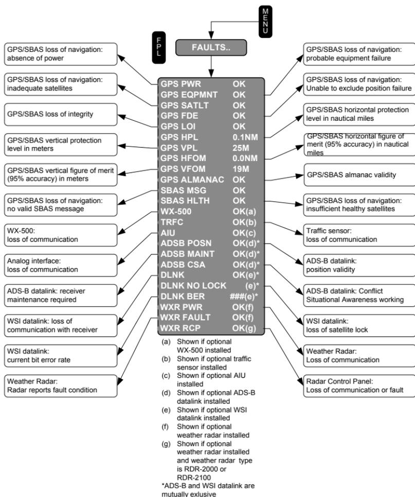
**Figure 5-82: Flowchart, MFD Fault Display (FAULTS) Menu**
