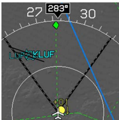
The aircraft's straight-and-level track over the ground is indicated on the directional scale by a green diamond. Ground track is based on GPS signal. The ground track symbol is connected to the aircraft symbol by a dashed green "lubber" line.
