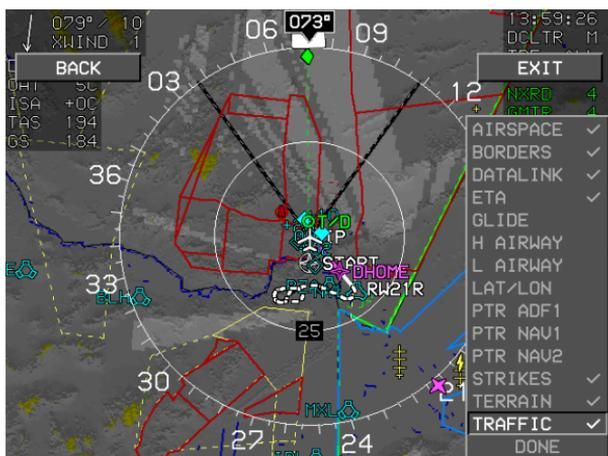
**Figure 5-120: Terrain-Show/Hide Terrain (Moving Map)**
