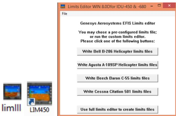
**Figure 8-10: ETT Limits Editor Icon and Configuration Tool**
