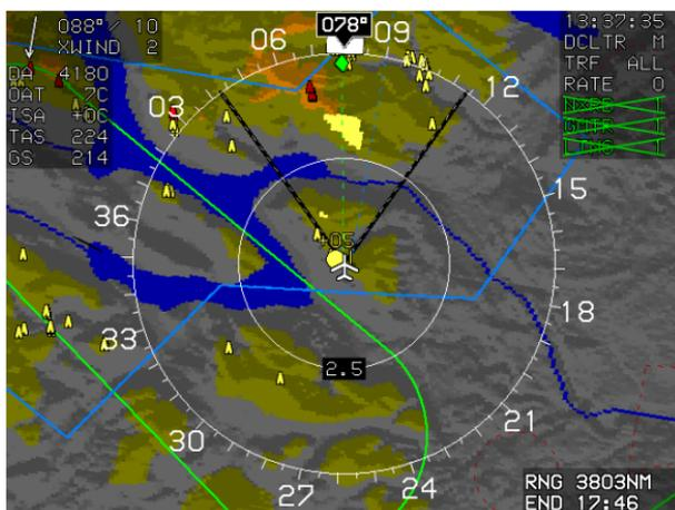
**Figure 3-119: Terrain Alert MFD**
