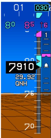
The AW-109SP VSI indication has a magenta Vertical Speed Datum Bug annunciated above the VSI scale with a resolution of 100 feet per minute.
