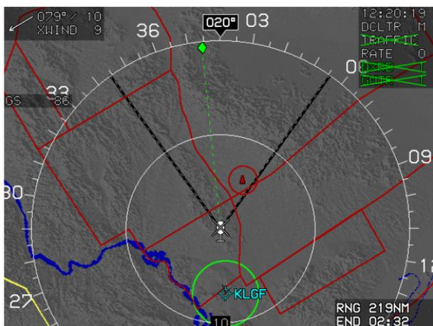
**Figure 4-57: ND Page during ADC Failure**
