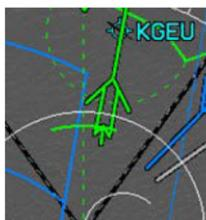
Thin (single pixel), dashed airspace lines indicate the airspace is cleared at the current altitude, and the aircraft is more than 500 ft. vertical from the airspace floor or ceiling.
