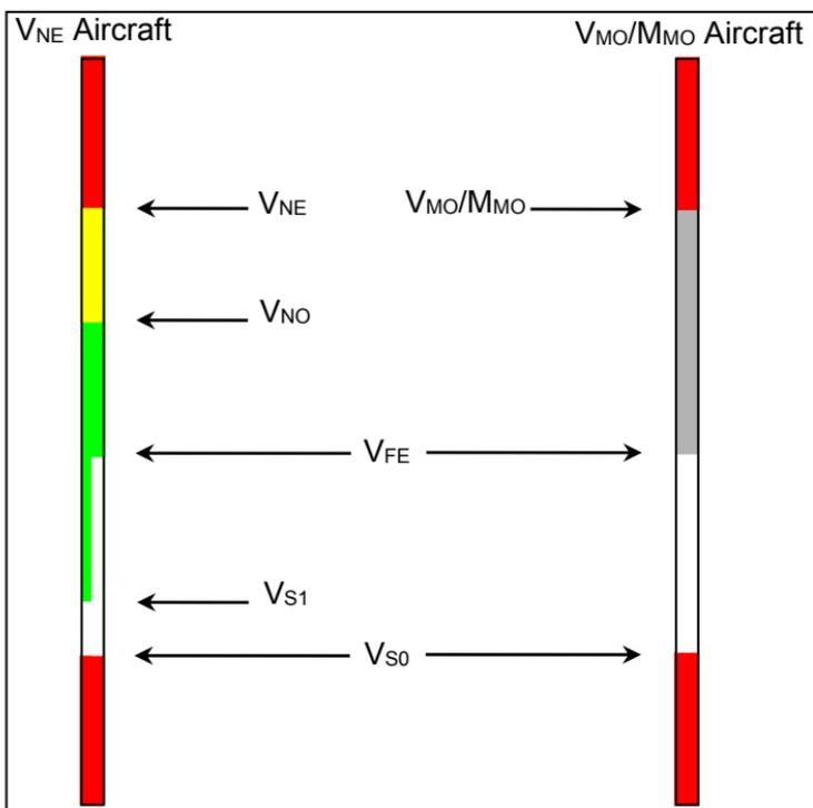
**Figure 3-34: Airspeed Scale Background**
