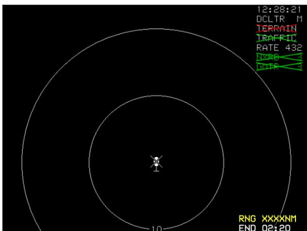
Figure 4-67: ND Page during GPS, ADC, and AHRS Failure
