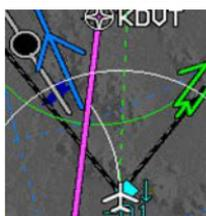
Thin (single pixel), solid airspace lines indicate the airspace is cleared at the current altitude, but the aircraft is within 500 ft. vertical of the airspace floor or ceiling.
