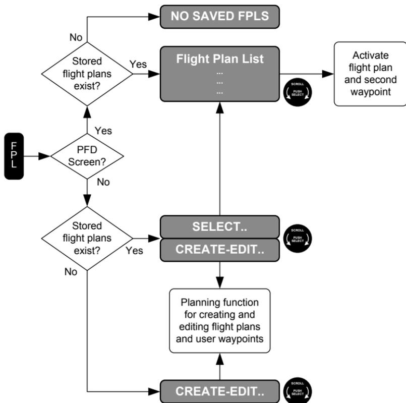
**Figure 5-18: Flowchart, Flight Plan (FPL) Menu**
