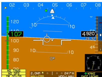
For the first minute after a GPS failure the FPM remains unchanged.
