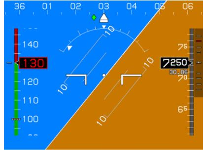
Rotorcraft in Basic mode rolling past  $\pm 50^\circ$  the SVS mode reappears for best attitude recovery to level flight.
