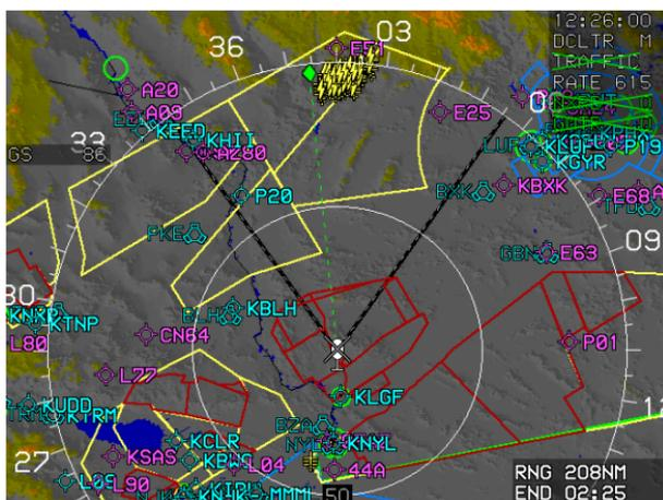
Figure 4-63: ND page during ADC and AHRS Failure
