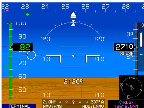
Figure 4-9: Pitch Scale
