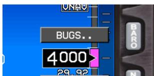
To activate a menu function, push the button corresponding with the menu. To display menus, push the Menu (R1). For example, push this button to activate the BUGS menu.
