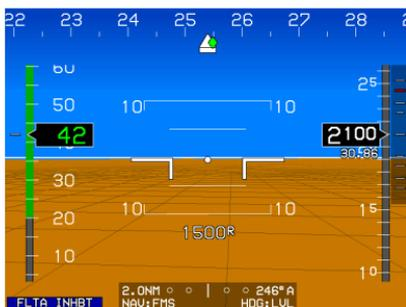
Bank angle scale decluttered from view in level flight above 30 Kts groundspeed.
