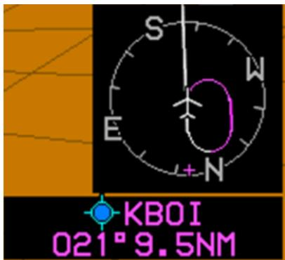
The waypoint information, indicating waypoint type and identifier, elevation, or crossing altitude, with bearing and distance is displayed immediately below the Mini Map.
