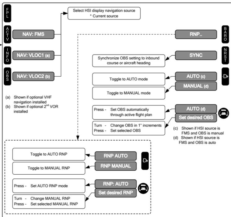
**Figure 5-54: Flowchart, Omnibearing Selector (OBS) Menu**
