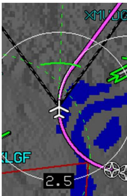
**Figure 3-77: Altitude Capture Predictor**
