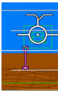
Waypoints (including destination airport) and fixes are displayed as magenta “tethered balloons”. The “X” on the ground at the bottom of the symbol indicates the waypoint's conformal (correct perspective) position on the surface of the earth, and the 200 ft. radius hoop at the top indicates the aircraft altitude or target altitude (if target altitude is set). In other words, fly the flight path marker through the hoop, and the aircraft is over the fix at the desired altitude.
