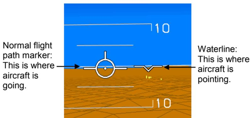
Normal pitch scale and flight path marker. Lateral position of flight path marker relative to waterline indicating a crab angle less than  $15^\circ$ .
