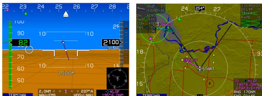
The Flight Path Marker is nearing the airspeed tape due to the excessive 36 knot crosswind from the right.
