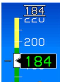
The current target airspeed is displayed in conjunction with the target airspeed bug, immediately above the airspeed tape. Lines above and below bracket the value. In this example, the target airspeed is set to 184 Kts.
