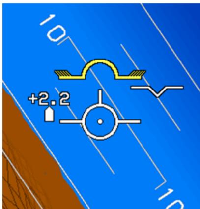
A G-Force indicator is located to the left of the Fight Path Marker (normal mode) or Large Aircraft Symbol Reference Marks (Basic Mode or Unusual Attitude Mode). The G-Force indicator has a “worm” format and gives an analog and digital representation of G-Force in gravitational acceleration units. The G-Force Indicator is decluttered when the difference between G-Force and 1-G is less than 0.3 Gs. Appearance of the G-Force
