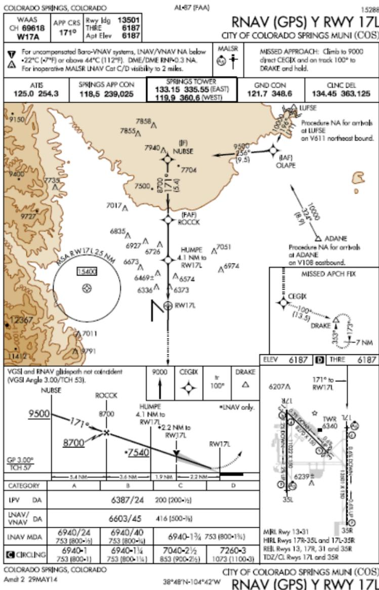
**Figure 7-22: RNAV (GPS) Instrument Approach to LPV Minima**
