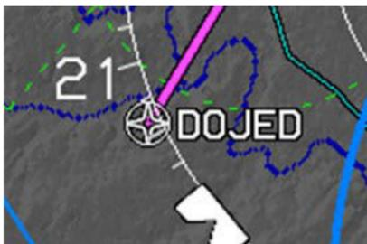
DOJED is an example of a fly-over fix, which has a wide circle around the waypoint star symbol.
