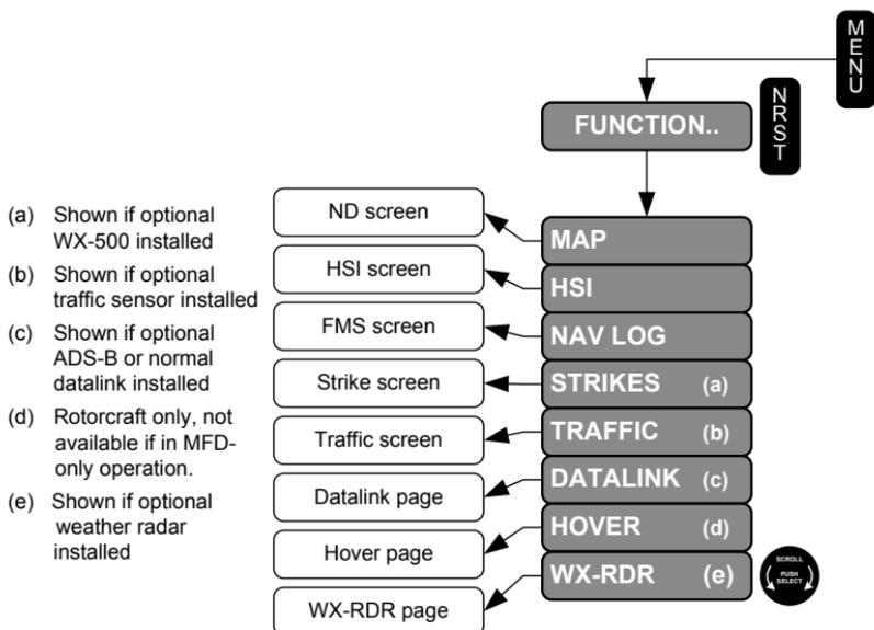
**Figure 5-86: Flowchart, MFD Function (FUNCTION) Menu**
