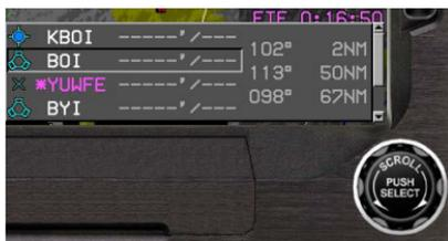
The right-hand encoder controls the menu when it appears in the lower right-hand corner of the screen. The encoder is numbered #1 from the right side as noted by **1**.
