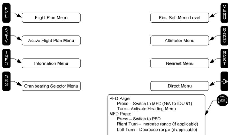
**Figure 5-5: IDU-450 Flowchart, Top Level Menu**
