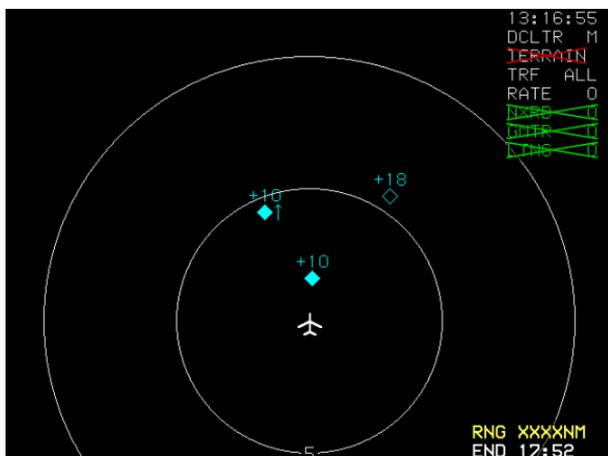
**Figure 8-66: ND Page during GPS, ADC, and AHRS Failure**
