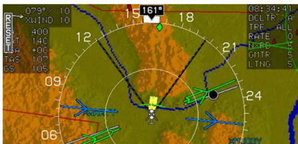
**Figure 4-73: Popup Mode Excessive Rate of Descent (GPWS Mode 1)**
