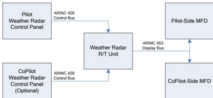
**Figure 8-50: Standard ARINC-708, Collins and Most Honeywell Digital Radars**
