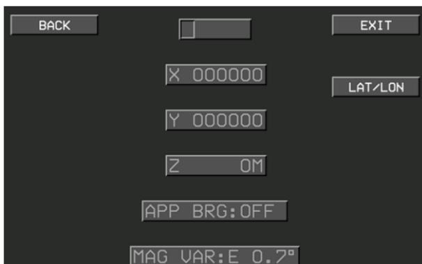
Figure 9-32: Creating a Waypoint Using Swiss Grid YXZ
