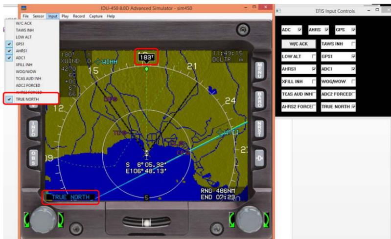
**Figure 8-22: True North Discrete Input Selected**
