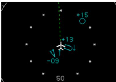
Asterisks are shown around the ownship aircraft symbol on the dedicated traffic display corresponding to positions of the clock to aid in identifying traffic relative to aircraft position. The scale of the reference ring is shown at the six o'clock position.
