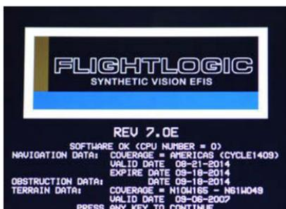
Power up the EFIS. The system performs a built-in test routine. If all tests pass, the system displays a screen identifying the database coverage. Press any button to acknowledge. The system begins a two-minute count down while awaiting sensor initialization (for the purposes of flight planning, etc., press any button to override this countdown).
