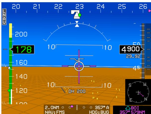
**Figure 3-29: Artificial Horizon and Actual Horizon, over Featureless Terrain**
