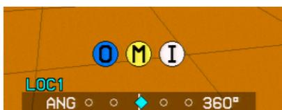
Conventional marker beacon indicators are shown centered in the lower portion of the PFD just above the CDI. During a built-in test more than one marker beacon may be active. In this mode, all active Marker Beacons (Inner, Middle, and Outer) is displayed side-by-side.
