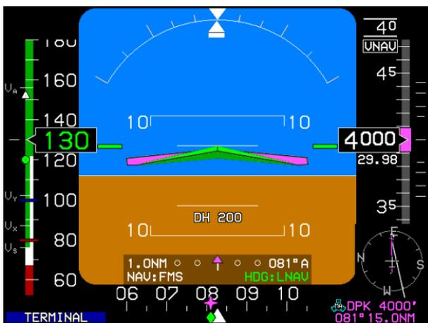
**Figure 3-44: Basic PFD Display with Conventional Flight Director Command Bar**
