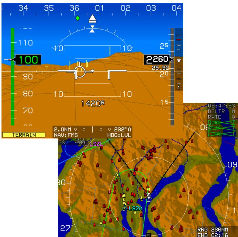
**Figure 4-68: PFD and MFD Terrain Display**
