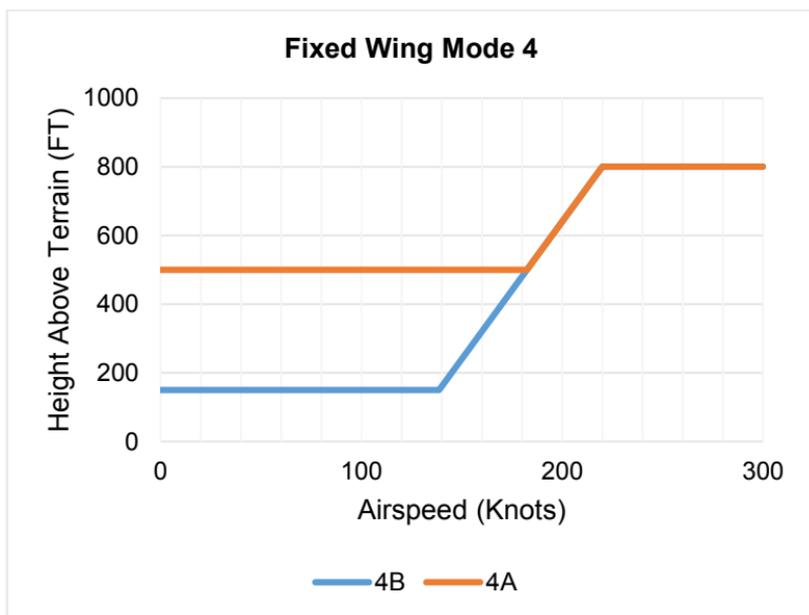
**Figure 8-42: Fixed Wing GPWS Mode 4**
