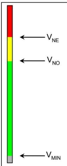
The airspeed scale for rotorcraft has markings to indicate  $V_{NE}$  (power off), commonly referred to as a "Barber pole", and also for translational lift reference if enabled. The  $V_{NE}$  marking is a red cross-hatched line on the airspeed Indicator. This normally indicates the power off recommended autorotation airspeed. If enabled, the translational lift marking is a white triangle on the airspeed indicator.
