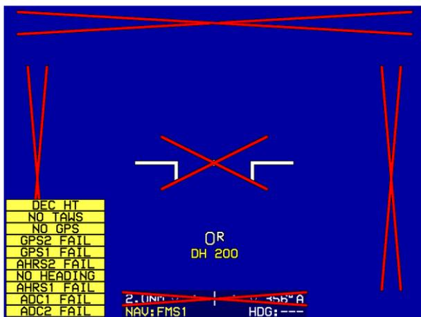
**Figure 8-65: PFD Page during GPS, ADC, and AHRS Failure**
