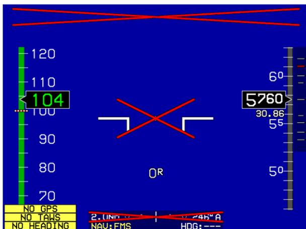
Figure 4-64: PFD Page during GPS and AHRS Failure
