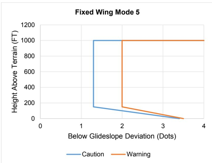
**Figure 8-43: Fixed Wing GPWS Mode 5**
