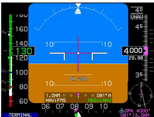
**Figure 3-45: Basic PFD Display With Cross Pointer Flight Director**
