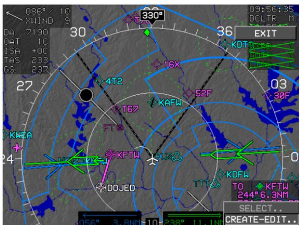
**Figure 5-27: Create a User Waypoint Using Latitude and Longitude-MFD Only**
