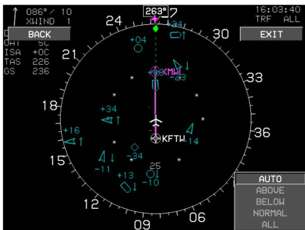
Figure 5-134: Optional ADS-B Datalink and Traffic
