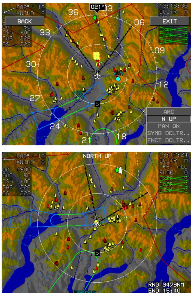
**Figure 5-101: Centered Display Format North-Up Orientation**
