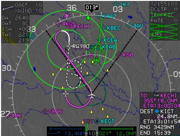
**Figure 3-89: Directional Scale in Arc Format**
