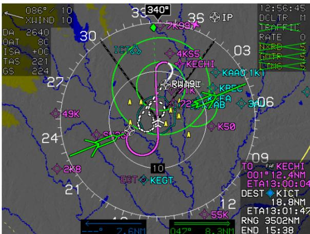
**Figure 3-90: Directional Scale in Centered Format**
