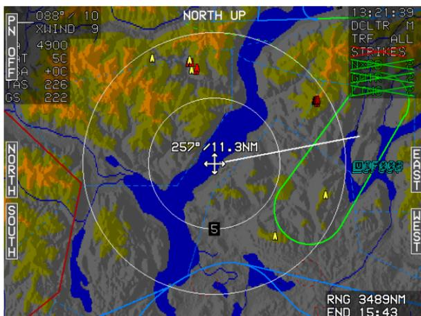
**Figure 5-105: Bearing and Distance from Current Position**
