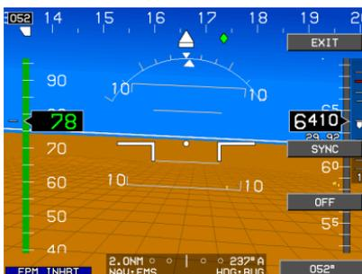
**Figure 4-8: Flight Path Marker Removal**
