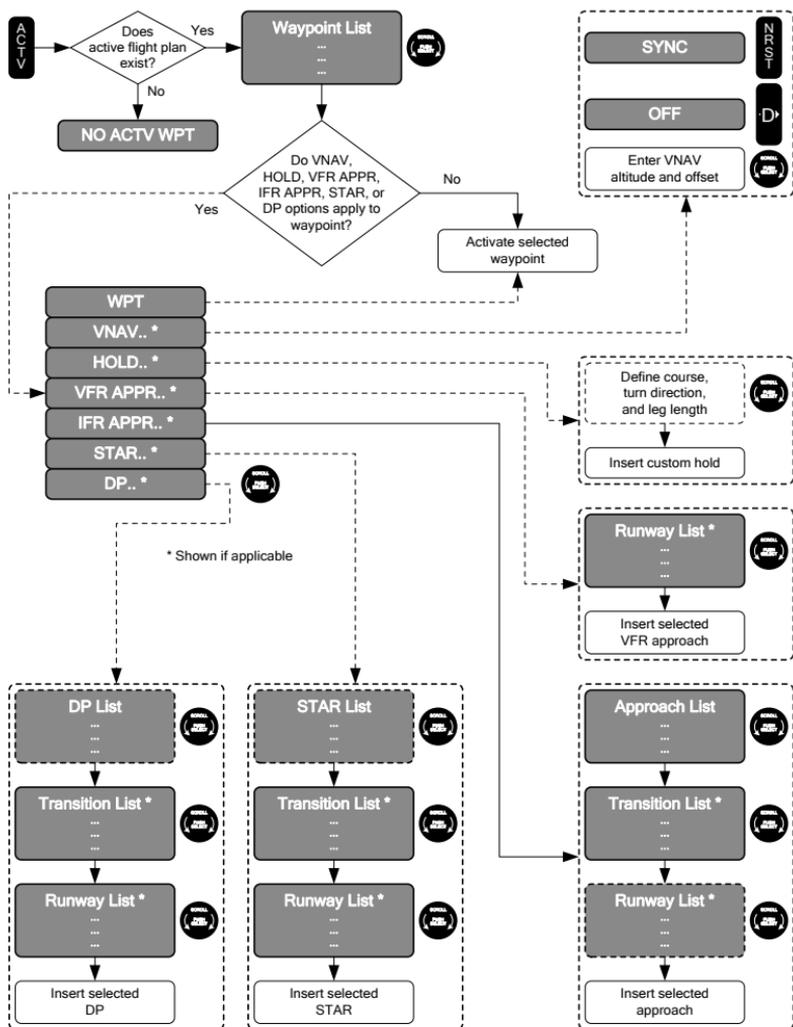
Figure 5-40: Flowchart, Active Flight Plan (ACTV) Main Menu
