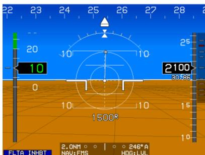
Bank angle scale automatically reappears below 30Kts groundspeed in hover vector mode.
