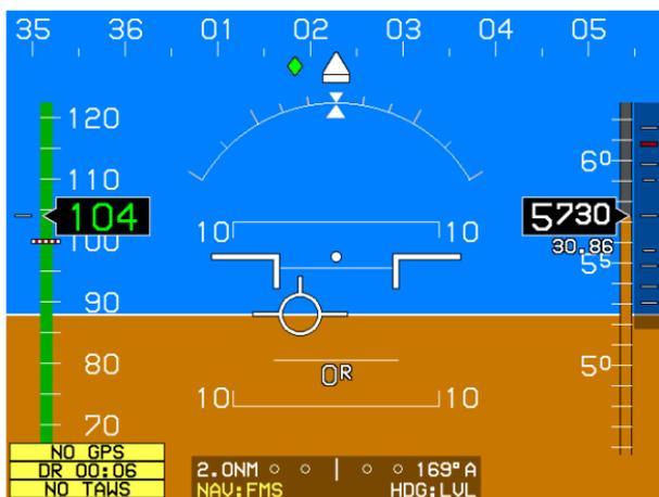
**Figure 4-54: PFD Page during GPS Failure**
