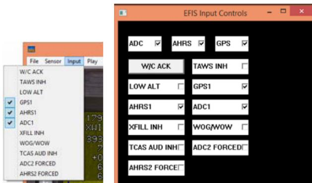
**Figure 8-21: Discrete Input Options in the Menu Bar**
