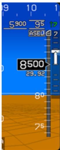
A vertical speed indicator (VSI) is located to the right of the altitude box. The VSI has a “worm” format and gives an analog and digital representation of VSI in feet per minute. This example of 700 FPM climb is set as a VSI bug and the actual rate of climb is 700 FPM.
