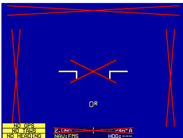
Figure 4-66: PFD Page during GPS, ADC, and AHRS Failure
