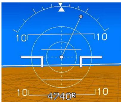
The hover vector is used to indicate direction and groundspeed of drift and appears at low groundspeeds of 30 Kts or less. The hover vector consists of Large Aircraft Symbol Reference Marks, an inner concentric ring indicating 10 knots groundspeed, an outer concentric ring indicating 20 knots groundspeed, and a vertical and horizontal dashed line passing through the center extending to the outer ring.
