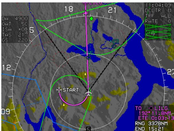
**Figure 8-58: ND Page during AHRS Failure**
