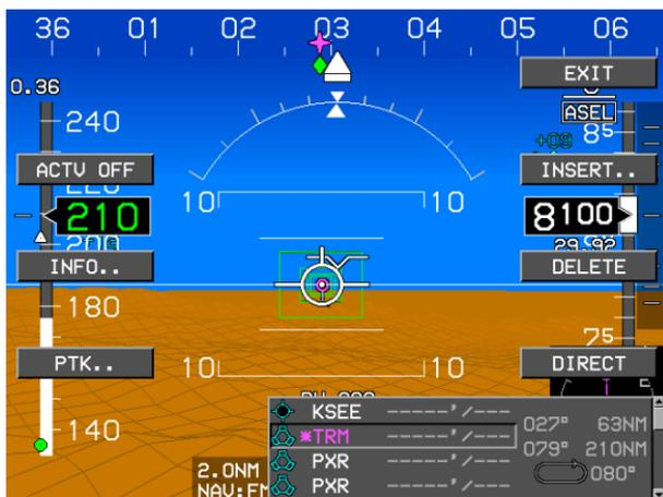
**Figure 5-50: Parallel Track Function-Set a Parallel Track**
