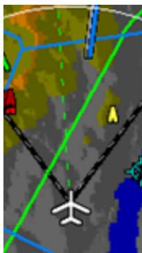
Heavy (double pixel), solid airspace lines indicate the airspace is penetrated at the current altitude.
