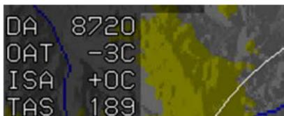
Outside air temperature (OAT) is displayed in the upper left corner of the navigation display, between density altitude (DA) and International Standard Atmosphere (ISA) temperature.
