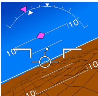
The roll datum bug is a magenta colored triangle bug that moves along the roll scale to indicate the desired roll.
