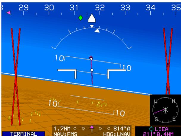
**Figure 4-56: PFD Page during ADC Failure**
