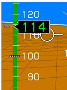
Flight Path Marker nearing Airspeed tape due to strong crosswind
