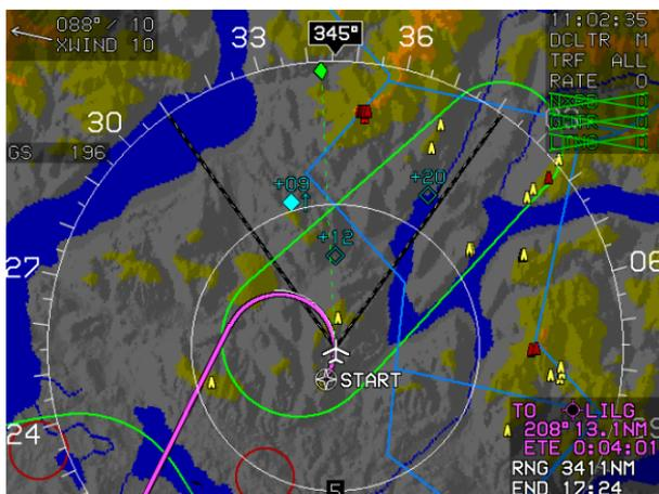
**Figure 8-56: ND Page during ADC Failure**
