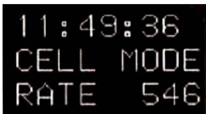
If the WX-500 sensor is enabled and functioning normally, the strike rate value is displayed next to the RATE annunciation in the upper right corner. The strike rate value, based upon the strikes within the selected range,
