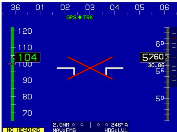
Figure 4-62: PFD Page during ADC and AHRS Failure
