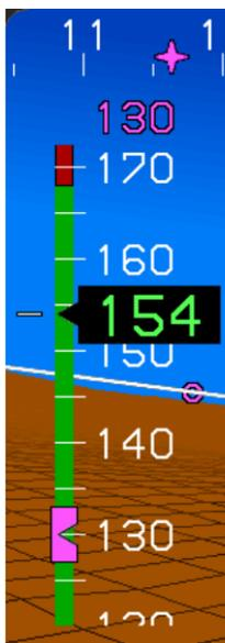
The AW-109SP airspeed scale has a magenta Airspeed Datum Bug indicating the desired airspeed. A digital readout of the desired airspeed is displayed in magenta above the airspeed scale. The example below indicates a value of 130 knots.
