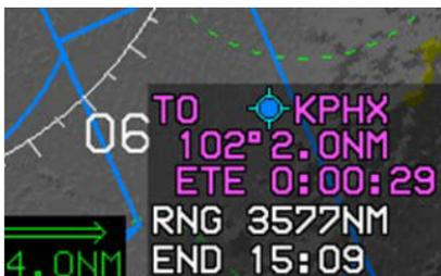
Fuel range (RNG) and endurance (END), based on fuel totalizer calculations, are displayed in nautical miles and hours: minutes, respectively. Totalizer information is displayed at the bottom of the waypoint navigation log for quick comparison with flight plan information. Totalizer data is not available in all installations.
