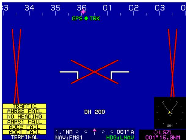
Figure 8-61: PFD Page during ADC and AHRS Failure
