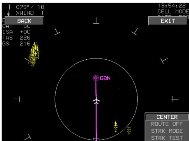
Figure 5-125: Stormscope Display (Arced Format)
