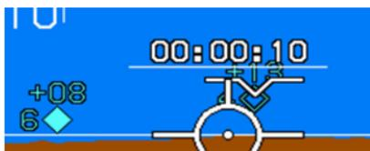
At the pilot's option, a timer (hours: minutes: seconds) is displayed immediately above the flight path marker. Timer may be set to count up indefinitely or count down from a pilot-specified
