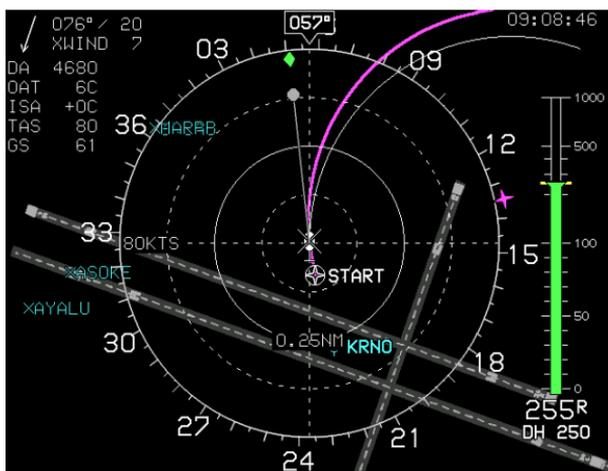
**Figure 4-18: Hover Vector Screen - ND (Hover Vector Active Flight Plan Path/Manual Course)**
