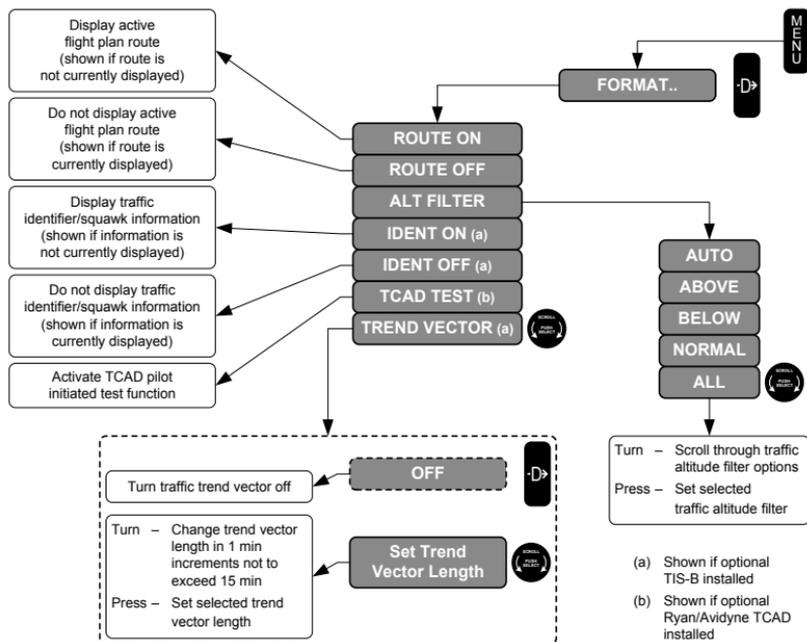
**Figure 5-127: Flowchart, MFD Traffic Format (FORMAT) Menu**
