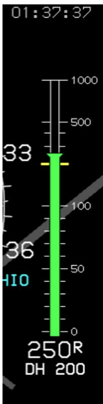
AGL altitude is displayed as an analog indication and digital readout on the right side of the hover screen, which is driven by whatever AGL altitude source being used as follows:.
