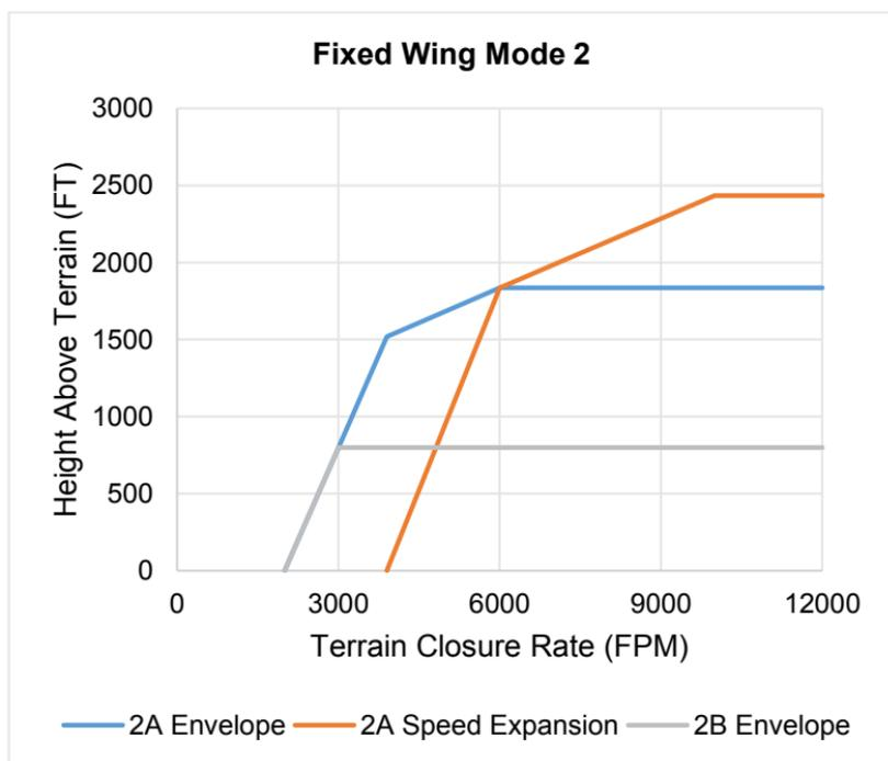
**Figure 8-40: Fixed Wing GPWS Mode 2**
