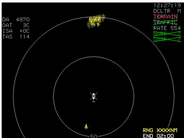
Figure 4-65: ND Page during GPS and AHRS Failure
