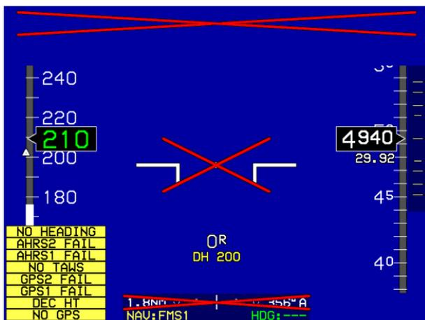
Figure 8-63: PFD Page during GPS and AHRS Failure
