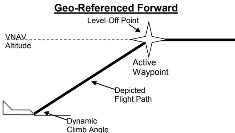
**Figure 7-4: Highway in the Sky (Geo-Referenced Forward)**
