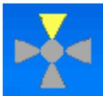
The AW-109SP Cyclic Cue is the autopilot's indication of the direction in which the cyclic control stick should be moved. The example below indicates the cyclic control stick should be moved in the forward direction.
