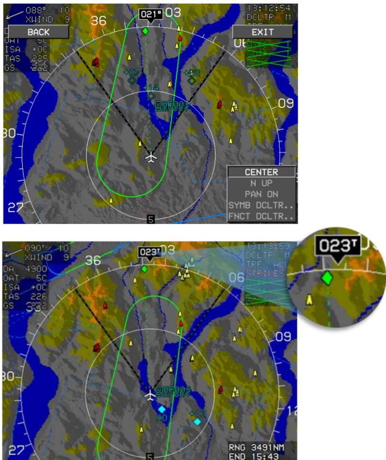
**Figure 5-100: Arced Display Format Heading-Up Orientation (True North Mode)**
