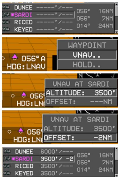
**Figure 7-14: Standard Terminal Arrival Route (STAR) (Step-by-Step)**
