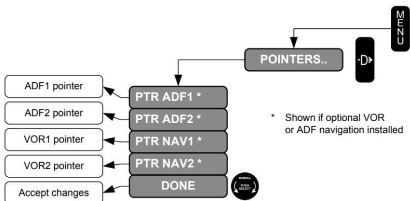
**Figure 5-121: Flowchart, MFD HSI Pointer (POINTER) Menu**
