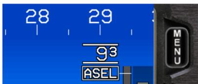
Press any of the peripheral buttons to activate the function indicated by the button label. In this example of button functions, press the **MENU** button to display the menus on the screen.
