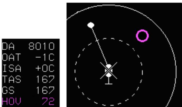
**Figure 9-20: Groundspeed Bug and Readout**
