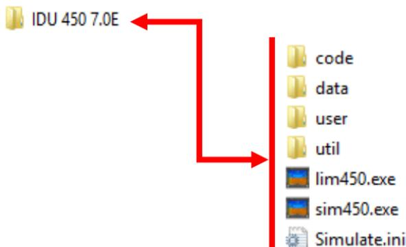
**Figure 8-5: Directory Mapping of EFIS Training Tool (IDU-450)**
