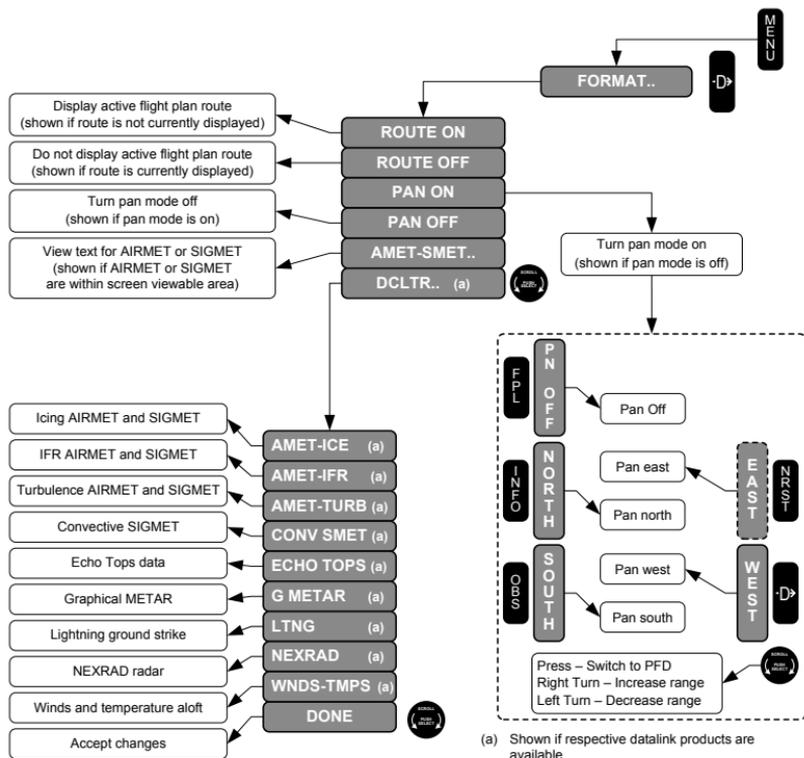
**Figure 5-129: Flowchart, MFD Datalink Format (FORMAT) Menu**
