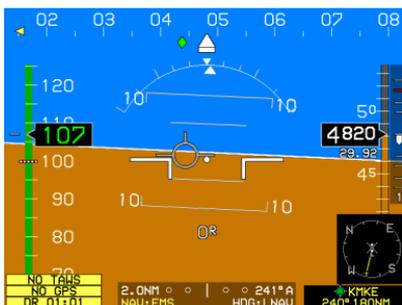
After one minute of dead reckoning following a GPS changes to a light gray color to indicate degraded performance.
