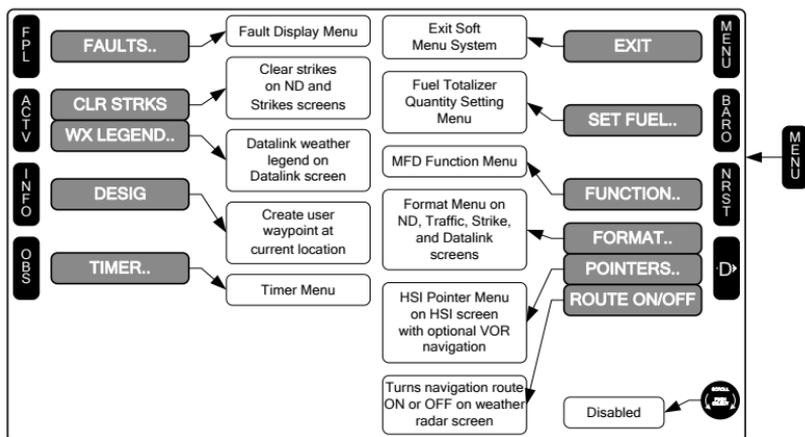
\* BARO bezel button is applicable to IDU-IV only. It is replaced with HDG bezel button on IDU-III.
