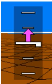
The AW-109SP Collective Position is displayed as a white bar on the collective scale and indicates the current position of the collective stick. The Collective Cue is displayed as a magenta arrow and indicates the direction in which the collective stick should be moved.
