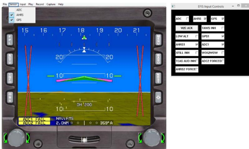
Figure 8-18: EFIS Training Tool ADC Sensor Failed
