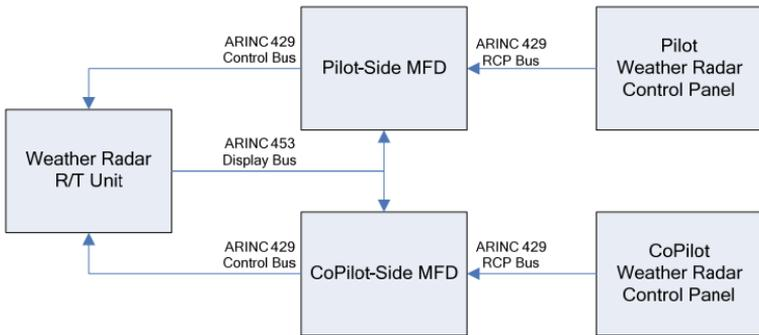
**Figure 8-52: Honeywell RDR-2XXX with Dual Radar Control Panel**
