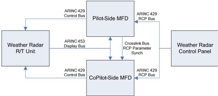
**Figure 8-51: Honeywell RDR-2XXX with Single Radar Control Panel**
