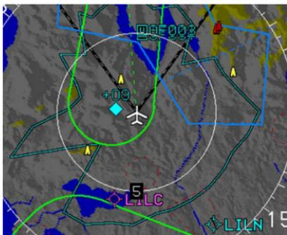
The range ring is a white circle (centered on the aircraft's position) used to quickly estimate distances. Distance (in nautical miles) from the aircraft to the ring is a white figure, overlaying the six o'clock position of the ring. The range ring is half the distance to the directional scale. Consequently, when the range ring shows a
