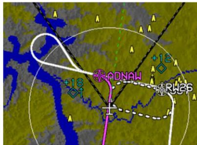
**Figure 3-102: Procedure Turn at Fix ADNAW**
