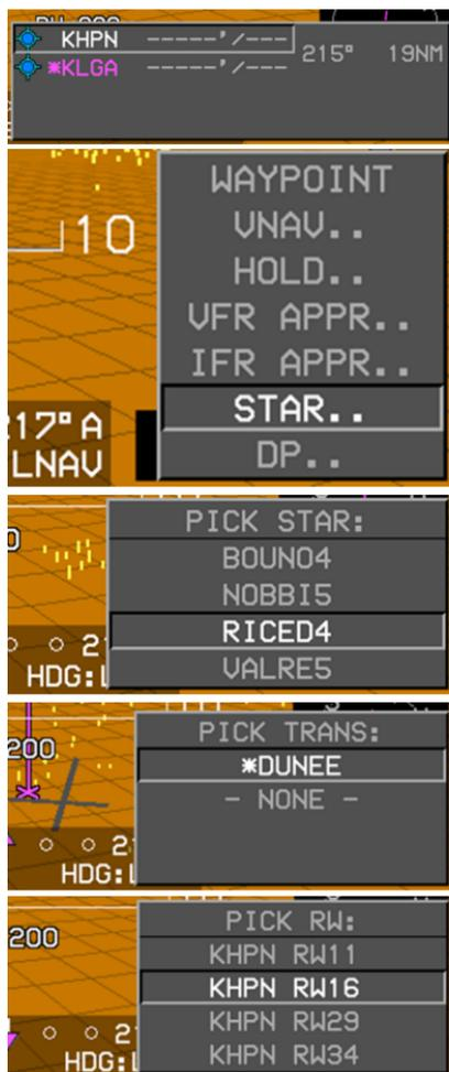
**Figure 7-13: Standard Terminal Arrival Route (STAR) (Step-by-Step)**
