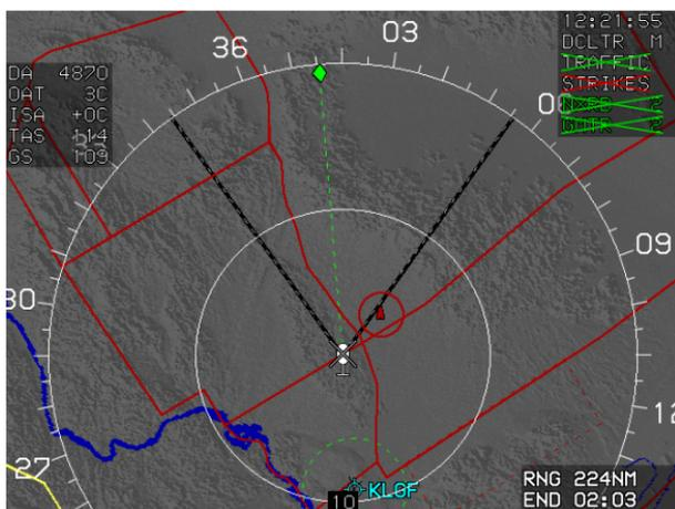
Figure 4-59: ND Page during AHRS Failure
