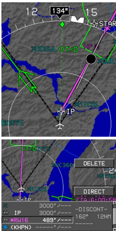
During this VTF VFR approach, the aircraft is proceeding direct to the IP. Since the IP is designated as a discontinuity, proceeding direct is not possible. When attempting to proceed direct to the IP, only the active leg between the IP and RW16 is activated.
