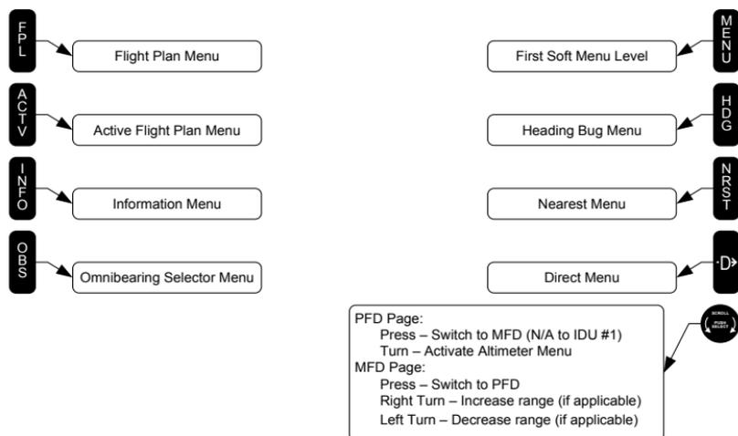
**Figure 5-6: IDU-III Flowchart, Top-Level Menu**
