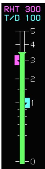
The Radar Height Bug is a magenta-filled bug with a notch to geometrically interact with the AGL indication. The Radar Height Readout is magenta text “RHT” followed by magenta numerical text indicating the value of the Radar Height Bug, placed above the AGL scale. The AFCS communicates the Radar Height value to the EFIS.
