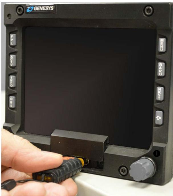
Figure 1-2: USB Memory Flash Door (IDU-450)
