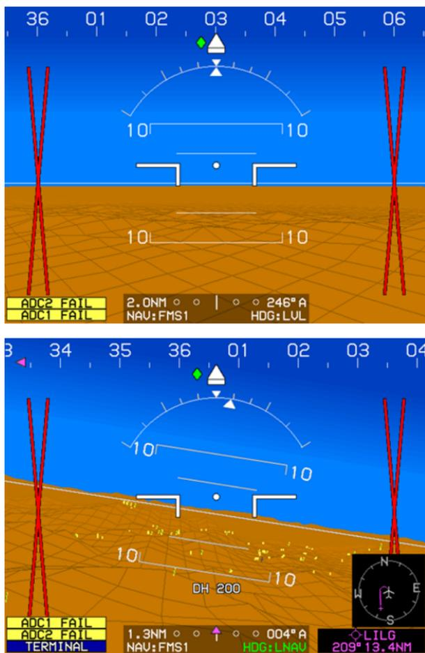
**Figure 8-55: PFD Page during ADC Failure**
