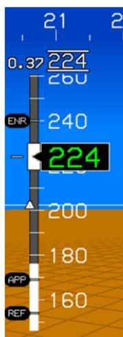
Approach speeds are shown here with  $V_{ENR}$ ,  $V_{APP}$ , and  $V_{REF}$  speeds selected.
