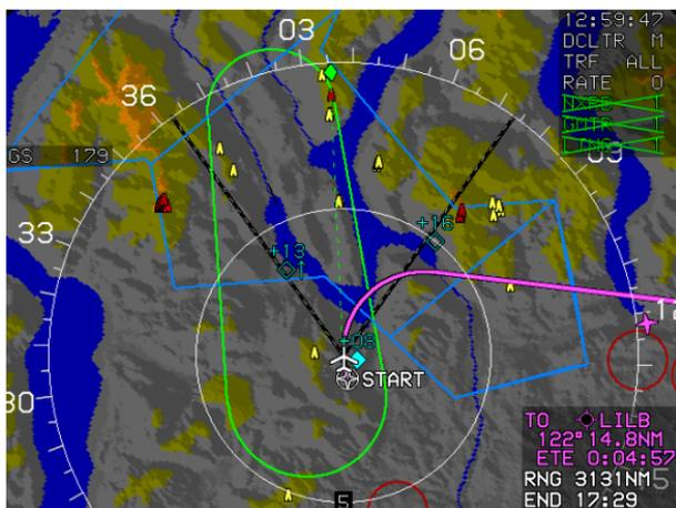
Figure 8-62: ND page during ADC and AHRS Failure
