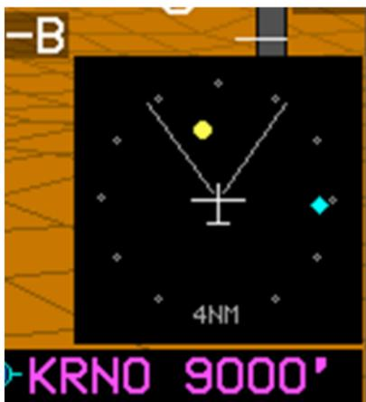
A traffic thumbnail is displayed in the lower right corner of the PFD above the active way point identifier.
