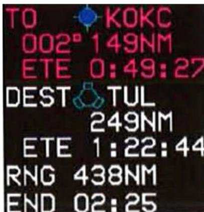
Waypoint navigation information is displayed in the navigation log box, located in the lower right corner of the display. The navigation log is only displayed when there is an active waypoint. The navigation shows the range, bearing, and estimated time enroute to the active "TO" waypoint and the destination "DEST" waypoint (along the route). Only the "TO" waypoint is shown if the "TO" and "DEST" waypoints are the same.
