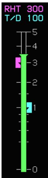
The Radar Height Datum Bug is a magenta bug sliding along the AGL scale on the Hover Page. The Transition-Down Pre-select Bug is a cyan bug sliding along the AGL scale. Both bugs have digital readouts above the scale.
