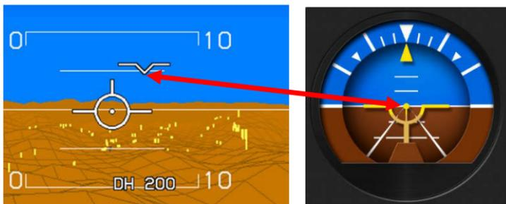
**Figure 3-65: Two Views of the Waterline; Aircraft is Pointed and Not Adjustable**
