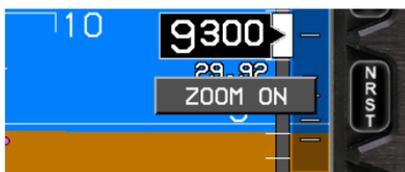
If menu tiles are shown, press the button adjacent to the menu tile to activate the menu. In this example of menu functions, press the **NRST** button (ZOOM ON menu tile) to turn on the PFD zoom function.
