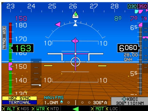
**Figure 9-30: Horizon Synchronization**
