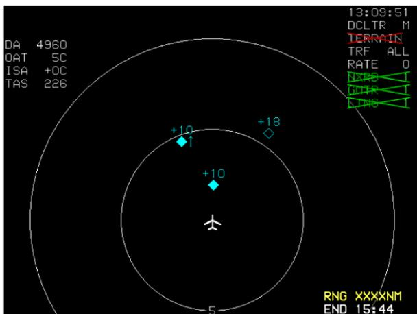
**Figure 8-64: ND Page during GPS and AHRS Failure**
