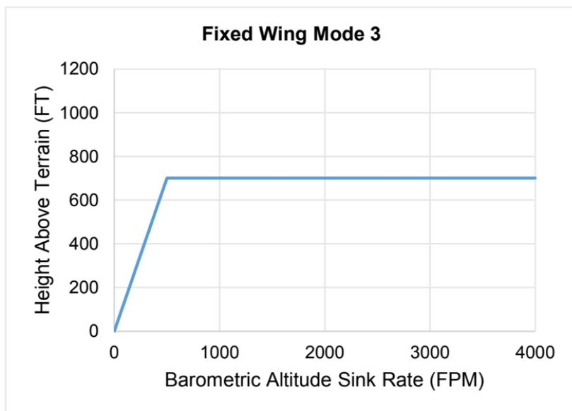
**Figure 8-41: Fixed Wing GPWS Mode 3**
