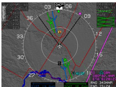
Obstruction within TAWS FLTA warning envelope with aural annunciation “Warning Obstruction, Warning Obstruction”, the obstruction symbols flash on the MFD only.
