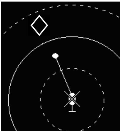
The A/C Acceleration Cue is an unfilled white diamond indicating the normalized Lateral and Longitudinal Acceleration. This symbol originates from the end of the hover vector and is independent of the current scale of the Hover Page. The input range is -1 to 1, and full scale (1) corresponds to the number of pixels from the center to the outer ring of the display. The A/C Acceleration Cue is limited and cropped at the outer circle of the HSI.
