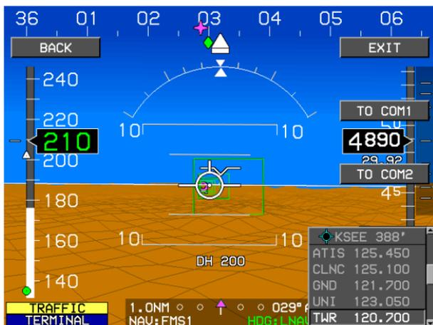
**Figure 5-53: Tuning Radios Using the EFIS**
