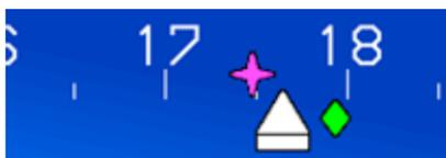
A magenta bearing to waypoint symbol is displayed on the directional scale. If the bearing to the waypoint is beyond the limits of the directional scale, a magenta arrow on the scale indicates the closest direction to turn.
