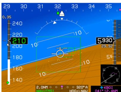
Airspeed is on the left, altitude on the right, heading across the top, and a FMS/VLOC CDI at the bottom. VSI is to the right of the altitude tape.
