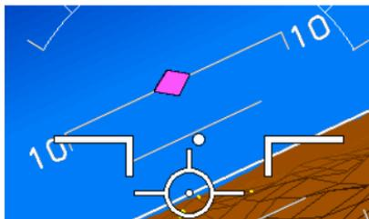
The pitch datum bug is a magenta colored diamond bug that moves along the pitch scale to indicate the desired pitch.
