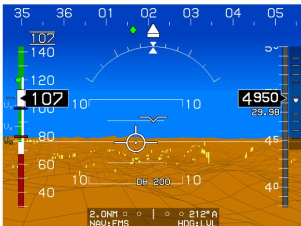
**Figure 3-64: V<sub>1</sub>, V<sub>R</sub>, and V<sub>2</sub> Selected with Bugs Menu**
