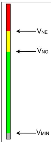
The airspeed scale background for Part 27 and 29 rotorcraft (Part 27 or 29 Airspeed Scale Type) has colored regions conforming to FAR § 27.1545 and FAR § 29.1545 as follows:
