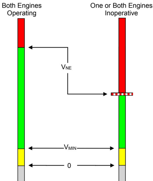
**Figure 9-6: Airspeed Scale with Engines Operating and Inoperative**
