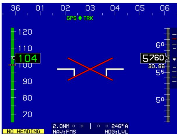
Figure 4-58: PFD Page during AHRS Failure
