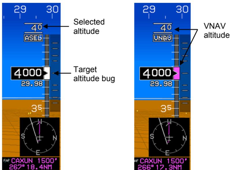
**Figure 3-51: Skyway Vertical Navigation (VNAV)**
