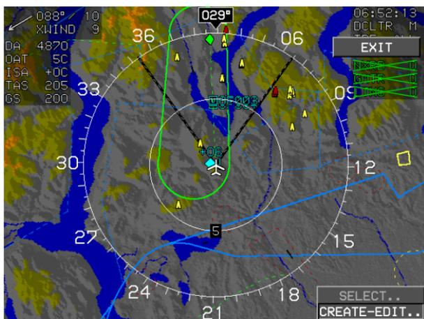
**Figure 5-30: Create a User Waypoint using Radial and Distance-MFD Only**
