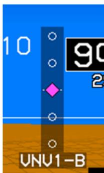
The PFD has a vertical deviation indicator on the right side of the display which displays vertical deviation for the currently selected vertical navigation source. When the selected vertical navigation source is FMS, the vertical deviation indicator conforms to the vertical deviation requirements of TSO-C146c.
