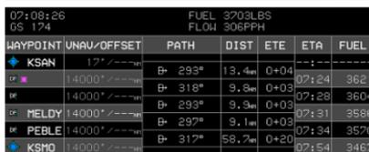
The MFD display shows the NAV LOG table. The table has columns for WAYPOINT, UNAV/OFFSET, PATH, DIST, ETE, ETA, and FUEL. The data is as follows:
