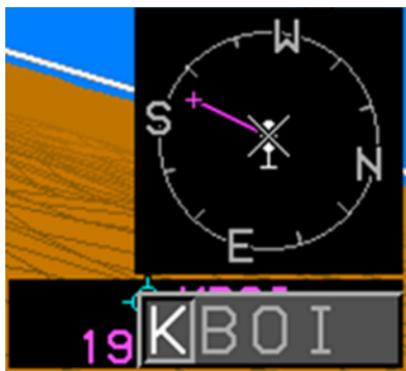
For example: To enter Boise Airport, scroll to select "B" then push to enter; scroll to select "O" then enter; scroll to select "I" then enter. Push two more times to step through the last two characters spaces (the leading "K" identifier may be entered but is not required). An exact match is accepted and entered automatically.
