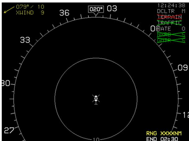
**Figure 4-61: ND Page during ADC and GPS Failure**
