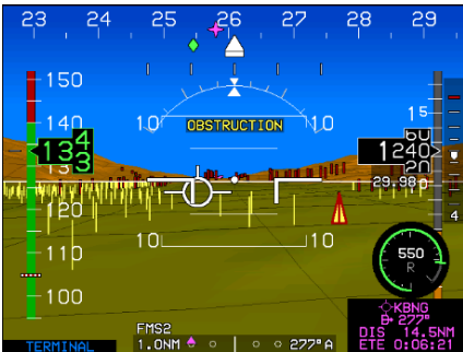
Obstructions creating an OBSTRUCTION caution
