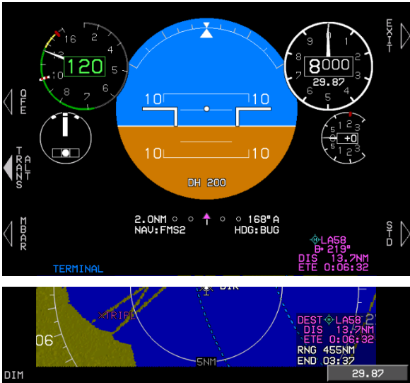
Figure RD-9: Altimeter Setting
