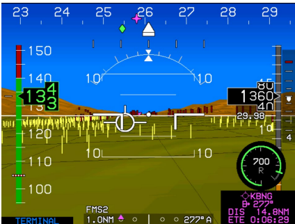
Obstructions without hazardous condition
