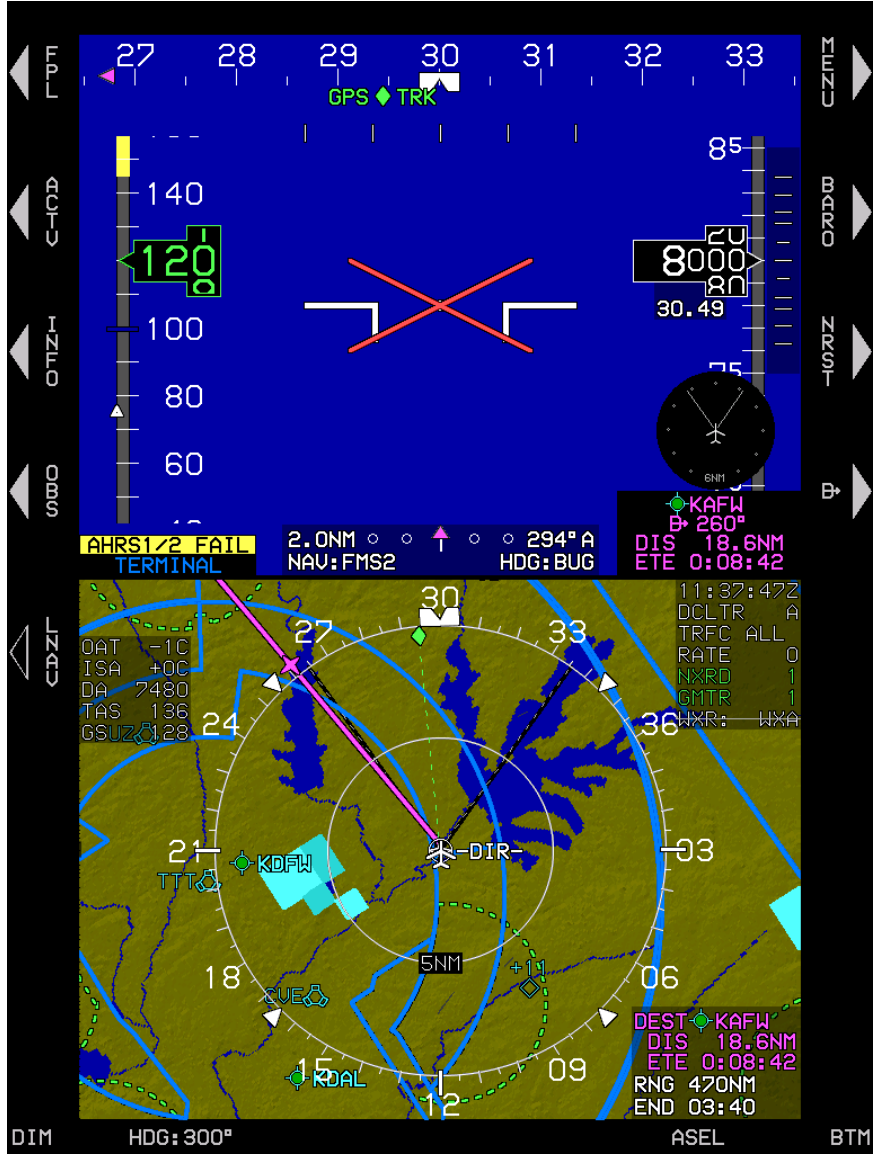
Figure 5-13: PFD Failure Mode 3 AHRs Failed, GPS/SBAS and ADC Normal
