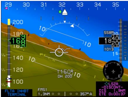
Obstructions without hazardous condition
