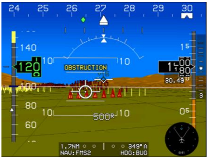
Obstructions creating an OBSTRUCTION caution
