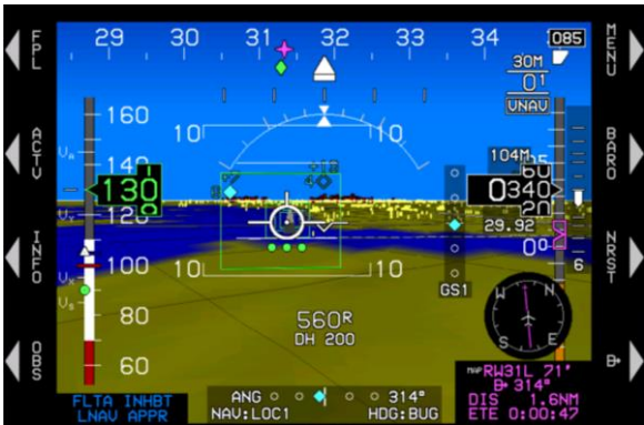
Figure 6-9: Highway in the Sky Final Approach Segment
