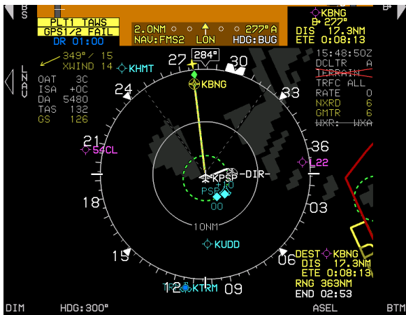
Figure 2-79: Loss of Integrity or Loss of Navigation
