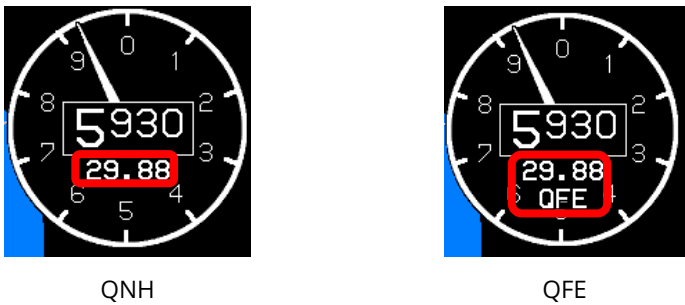
Figure RD-11: Altimeter
