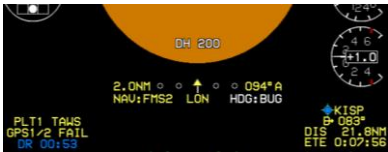
NAV Source FMS2 (GPS/SBAS failed LOI/LON condition)
