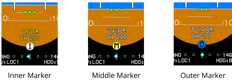
Figure RD-3: Marker Beacon Indicators
