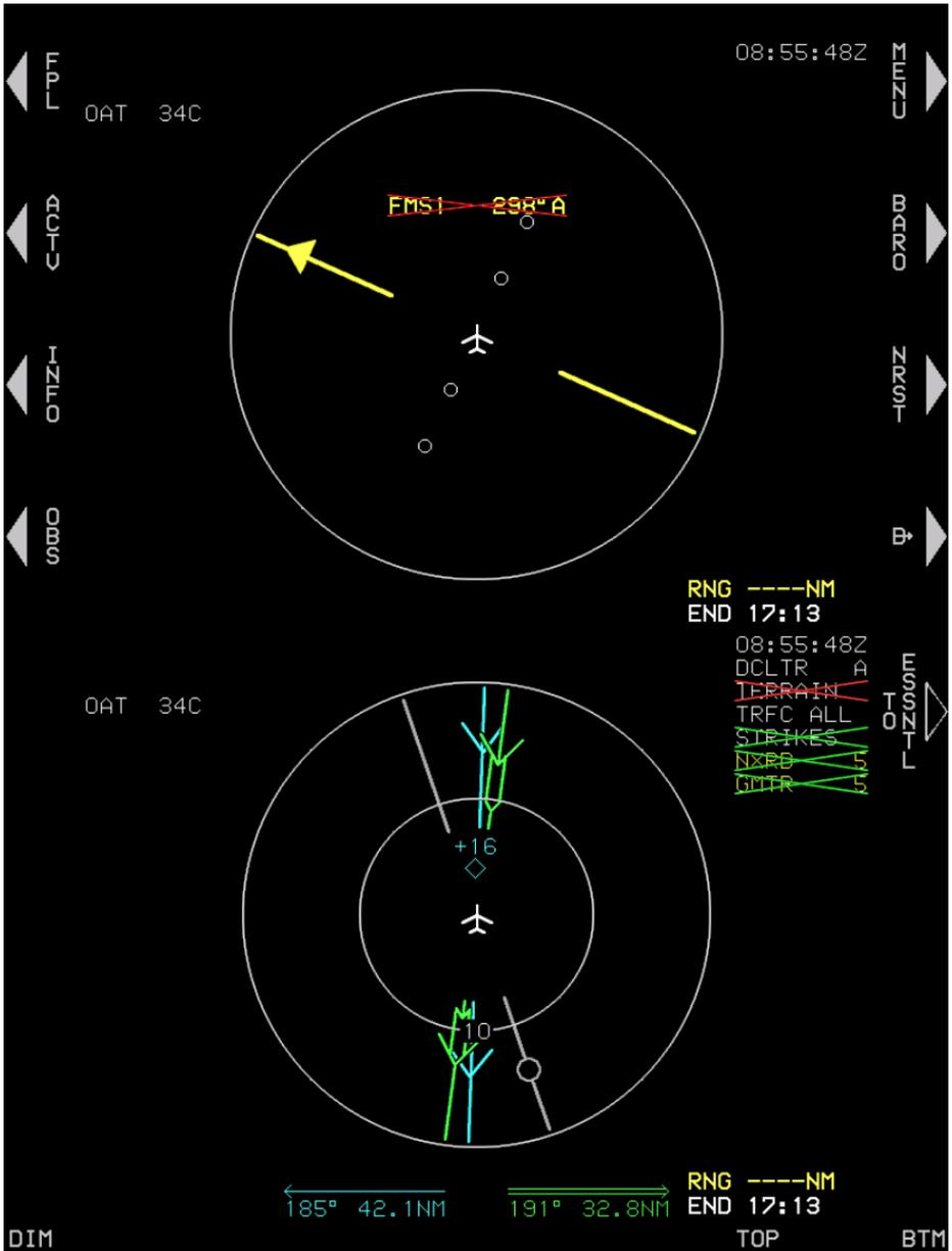
**Figure 4-28: MFD Failure Mode 7 (Normal Mode)
