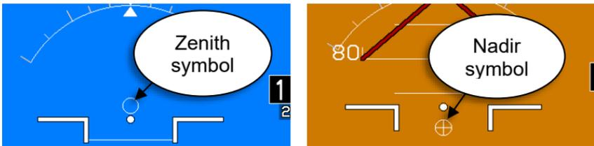
**Figure 3-34: Pitch Scale Zenith and Nadir Symbol**
