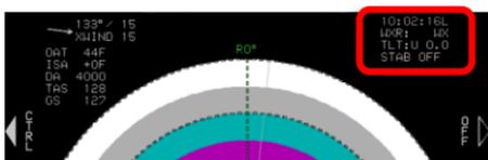
15) Radar mode of operation annunciated in upper right corner.
