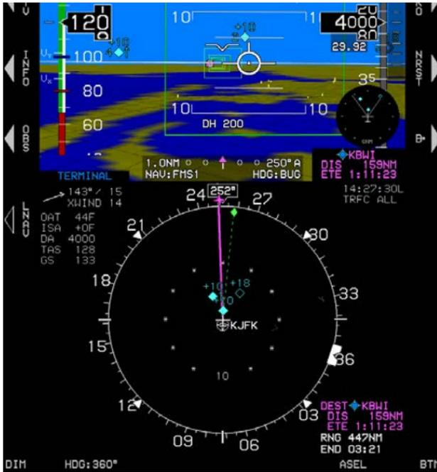
**Figure T-8: Traffic Display Format**
