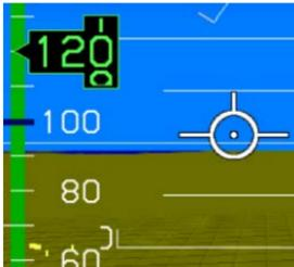
FPM nearing airspeed tape due to strong crosswind from the right.
