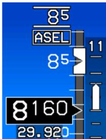
A target altitude may be set on the autopilot controller. When in selected altitude sub-mode, the altitude scale has a pilot-settable target altitude bug geometrically interacting with the altitude box pointer. The target altitude bug value has a resolution of 100 feet and a range from -1000 feet to 50,000 feet. The target altitude bug setting annunciation includes “ASEL” indicating selected altitude sub-mode.
