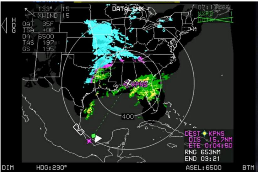
Figure D-2: Datalink Symbology with NEXRAD On
