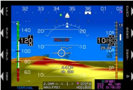
Indicated airspeed is on the left, altitude is on the right, and heading is across the top. FMS/VLOC CDI is located on the bottom. VSI appears on the right side of the altitude tape. Time-critical caution is displayed in the primary field of view.
