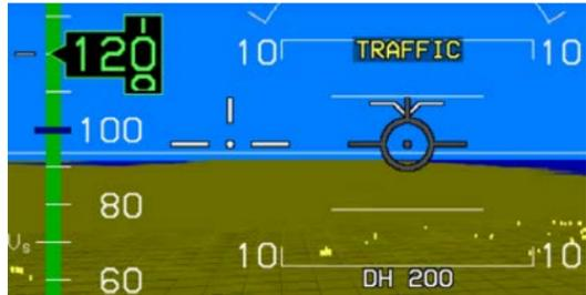
FPM caged in center due to excessive crosswinds from the right. Ghost FPM appears in proper lateral location.
