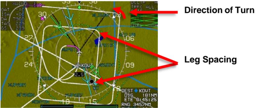
Figure SAR-3: Expanding Square Pattern-Turn and Leg
