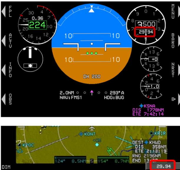
Figure RD-13: Altimeter Setting
