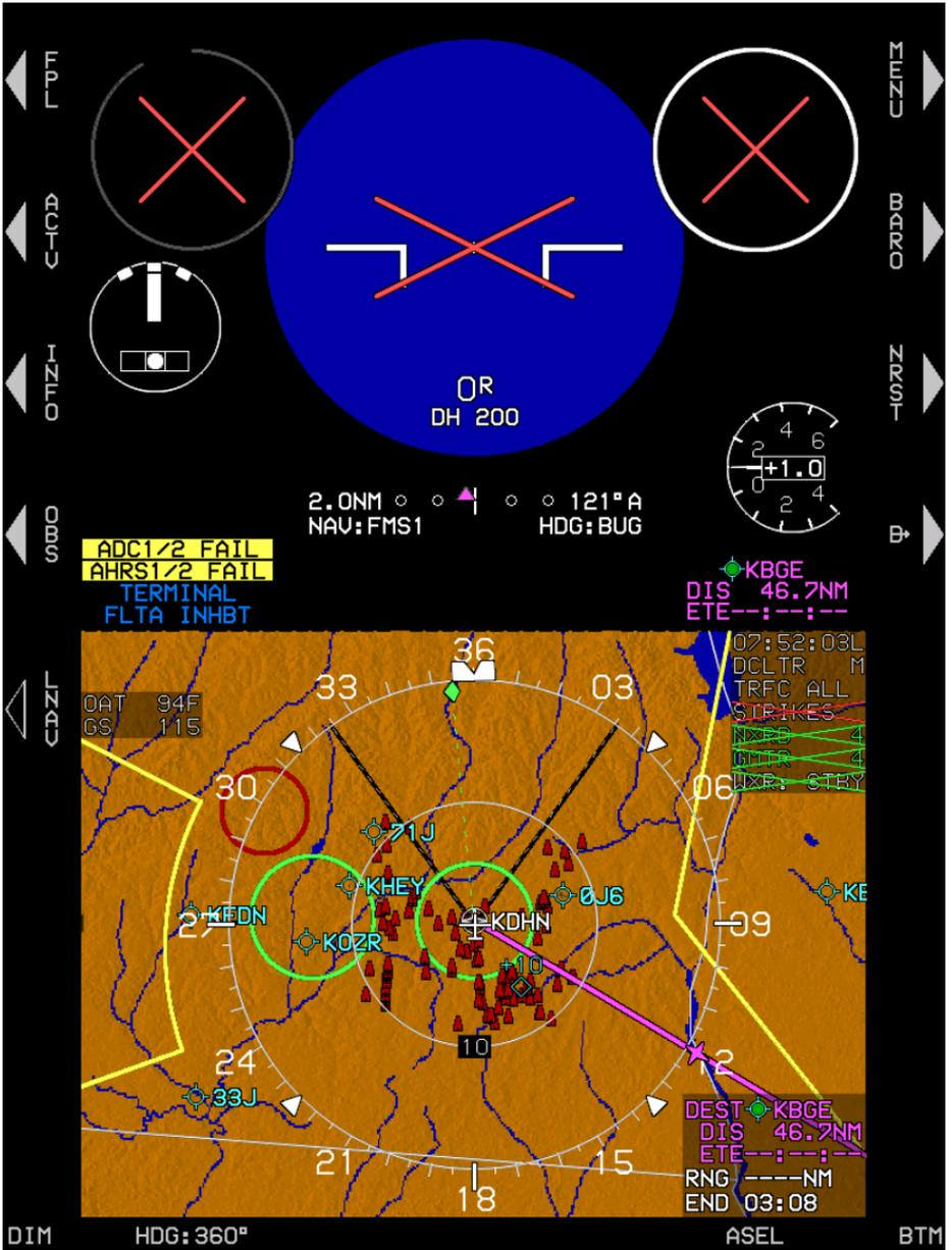
Figure RD-47: PFD Failure Mode 6
