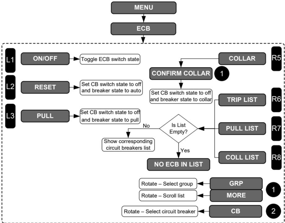
**Figure ECB-6: Second Level ECB Control Menu**
