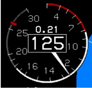
The airspeed display digitally displays indicated airspeed in knots, miles per hour, or kilometers per hour as set in the EFIS limits. The display is scaled to show the entire operating range of the aircraft. CW movement corresponds to increasing speed. When an ADC sensor fails, the display appears as shown in Figure RD-18.
