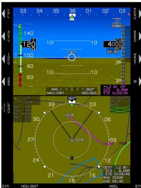
15) Rotate **1** CW to change map scale to **5NM** (inner scale) **10NM** (outer scale) and then turn the aircraft for a right downwind toward the IP. (Automatically created approximately **12NM** out on the **130°** approach bearing to the runway.)
