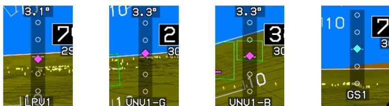
**Figure 3-60: Vertical Deviation Indicator**
