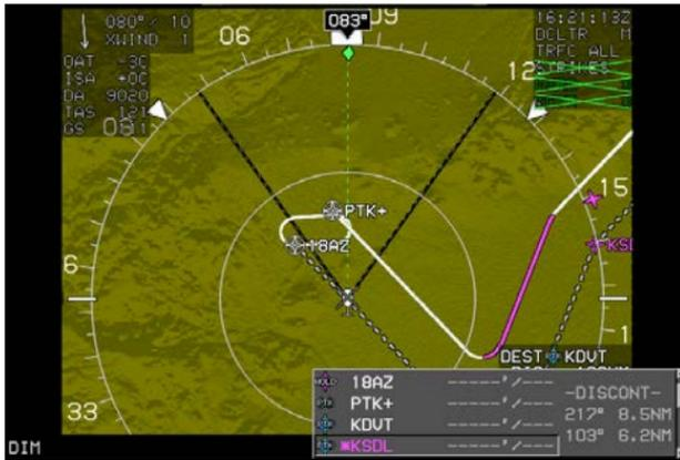
**Figure 7-12: Parallel Offset PTK+/PTK ENTRY**
