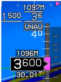
Altitude values (altitude display and pilot-selectable target (ASEL) and VNAV altitudes) may be displayed in metric units with a resolution of 1 meter.
