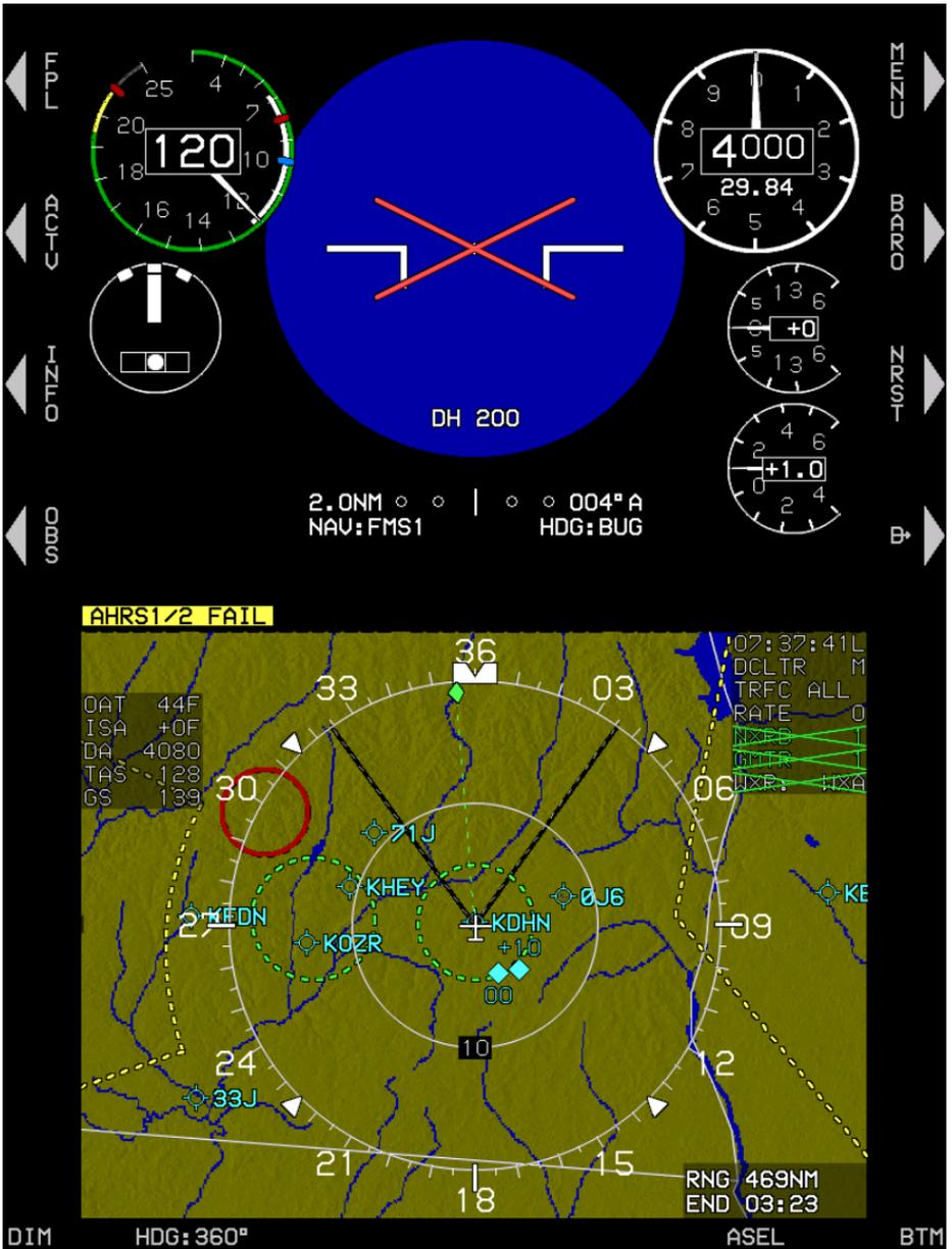
**Figure RD-44: PFD Failure Mode 3
