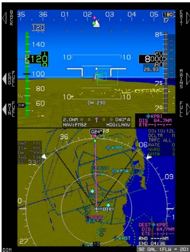
Figure 5-35: Fuel Totalizer Quantity Setting (SET FUEL) Menu
