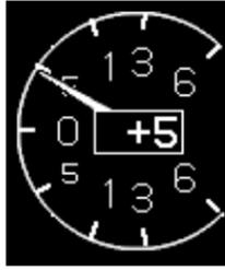
**Figure RD-22: Vertical Speed Indicator**
