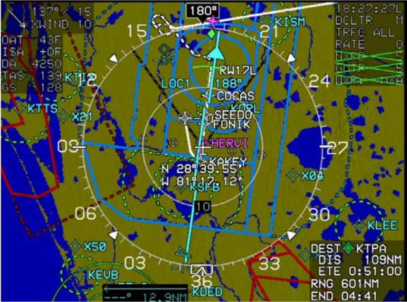
Figure 3-68: Moving Map with Instrument Approach with HSI Enabled
