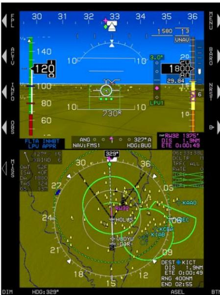
17) VDI displays vertical guidance for the LPV vertical profile based on GPS/SBAS.
