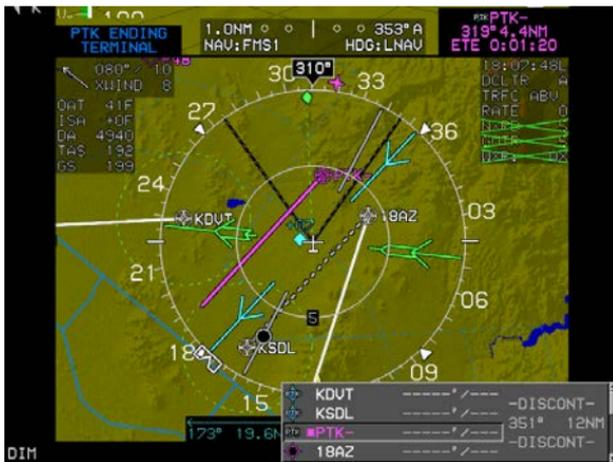
**Figure 7-13: Parallel Offset PTK-/PTK ENDING**
