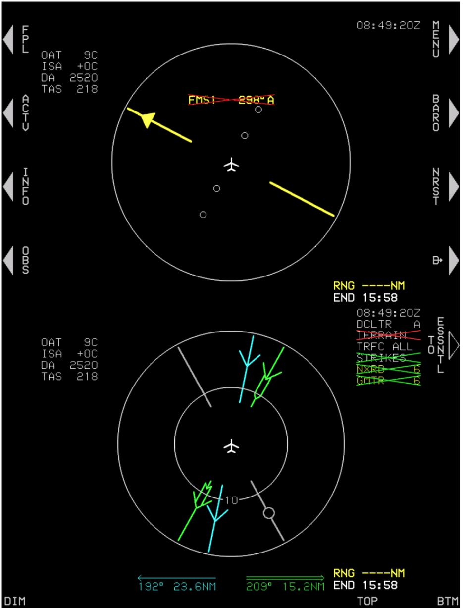
**Figure 4-22: MFD Failure Mode 5 (Normal Mode)
