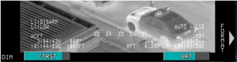
**Figure V-3: Video Page Contrast and Brightness Setting**
