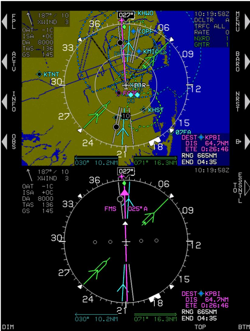
**Figure 2-2: IDU-680 Multifunction Display (MFD)**
