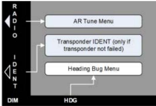
**Figure 5-6: PFD or MFD Essential Mode Top-Level Menu with Audio Radio Management Option**
