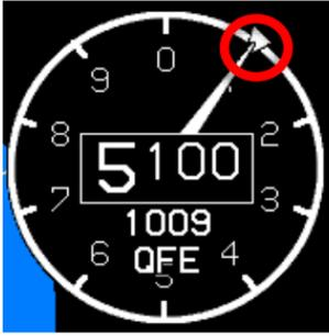
When in VNAV sub-mode, the VNAV altitude bug appears when within 500' from the current altitude. In this example, the VNAV altitude is 5,100'.
