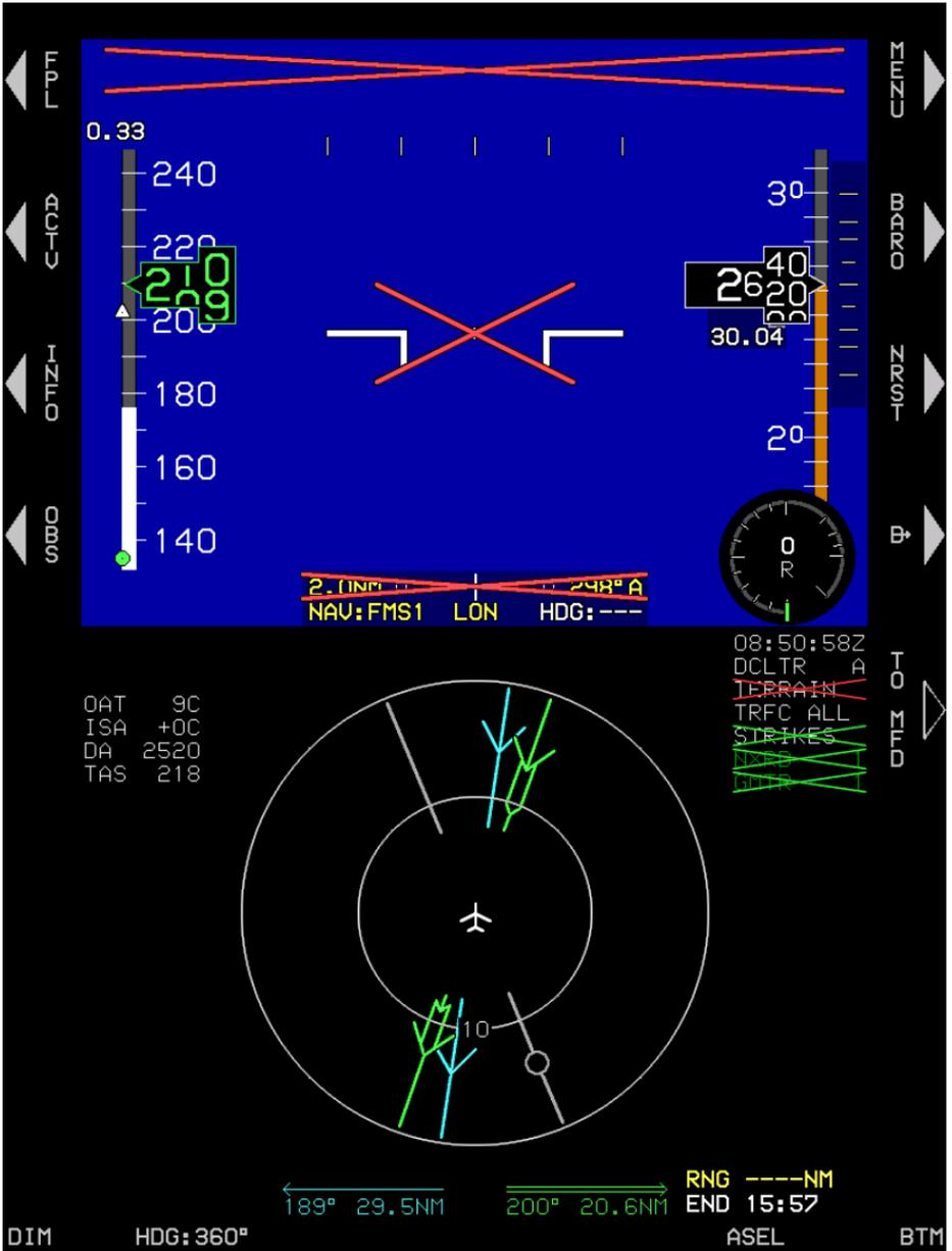
Figure 4-23: MFD Failure Mode 5 (Essential Mode)
