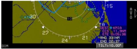
12) In manual mode, rotate **2** to set tilt angle between  $\pm 15^\circ$ . Set angle is annunciated above **2** and in the upper right corner.
