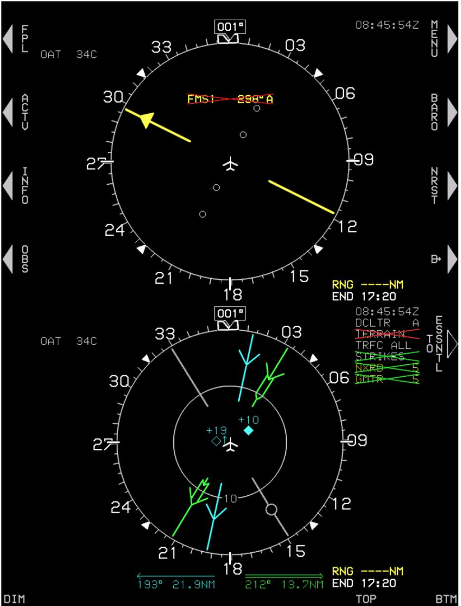
**Figure 4-19: MFD Failure Mode 4 (Normal Mode)
