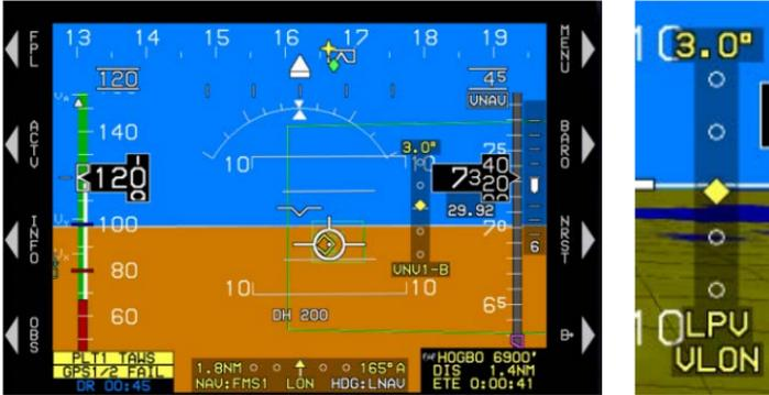
Figure 3-61: VDI Color during GPS/SBAS LON or VLON
