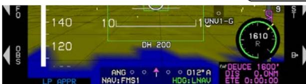
**Figure 7-15: FSD Lateral Deviation Indicator Linear Deviation (not VTF Approach)**
