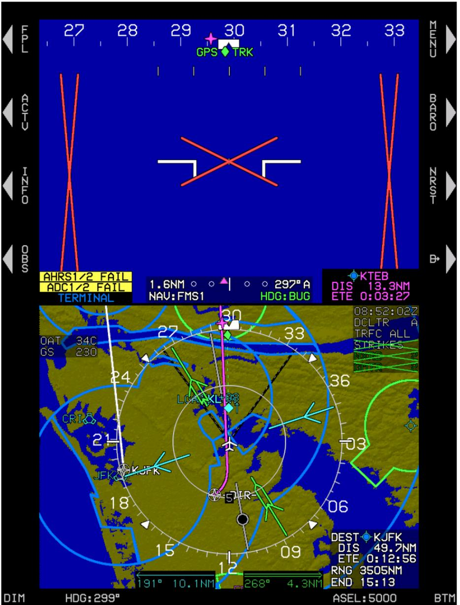
**Figure 4-24: PFD Failure Mode 6**
