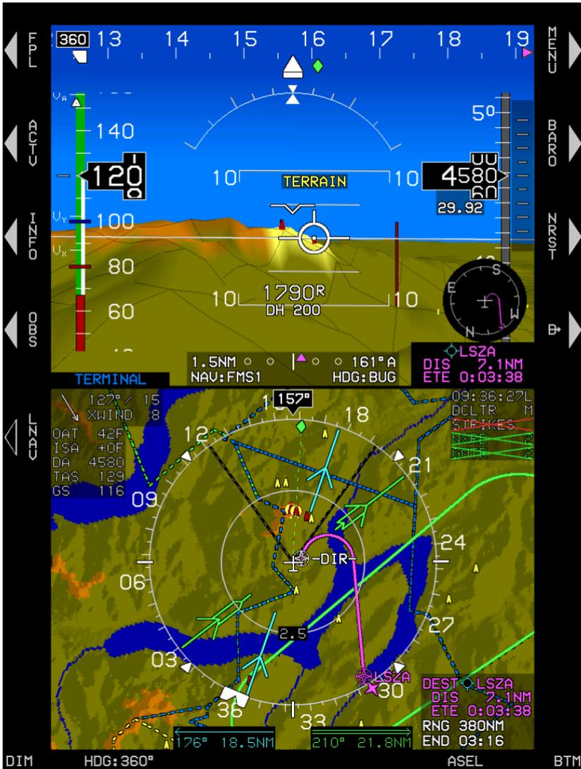
If SVS TAWS and SVS BASIC were not checked and the aircraft pierced the TAWS FLTA Terrain envelope, the EFIS automatically enables SVS TAWS. **TERRAIN** takes precedence over **OBSTRUCTION**.
