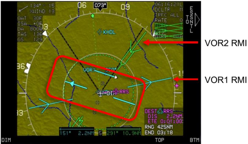
**Figure 3-80: Analog Navigation Symbolology, HSI in ARC Mode**
