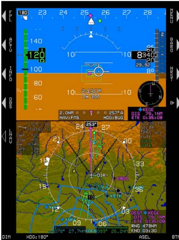
**Figure 3-45: PFD with Terrain Deselected but Retained on Map**
