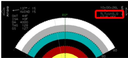
13) Tilt mode was in manual and tilt angle set to  $6.00^\circ$  and annunciated in full IDU image.
