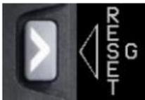
Press **RESET G (L2)** to reset telltales to zero, unless the aircraft G-limits have been exceeded. If G-limits have been exceeded, reset exceedance in GMF.
