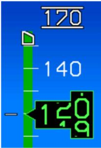
When the airspeed bug value differs from aircraft speed to the extent the bug is off scale, the bug appears to be “parked.”
