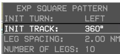
Figure SAR-2: Expanding Square Pattern Parameters
