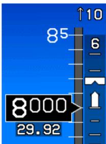
The VSI indication can have a pilot-settable vertical speed bug with a 100 fpm resolution and a range from -3000 to +3000 fpm. It is mutually exclusive with the airspeed bug.
