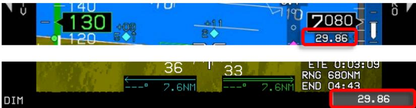
**Figure 3-13: Altimeter Setting**
