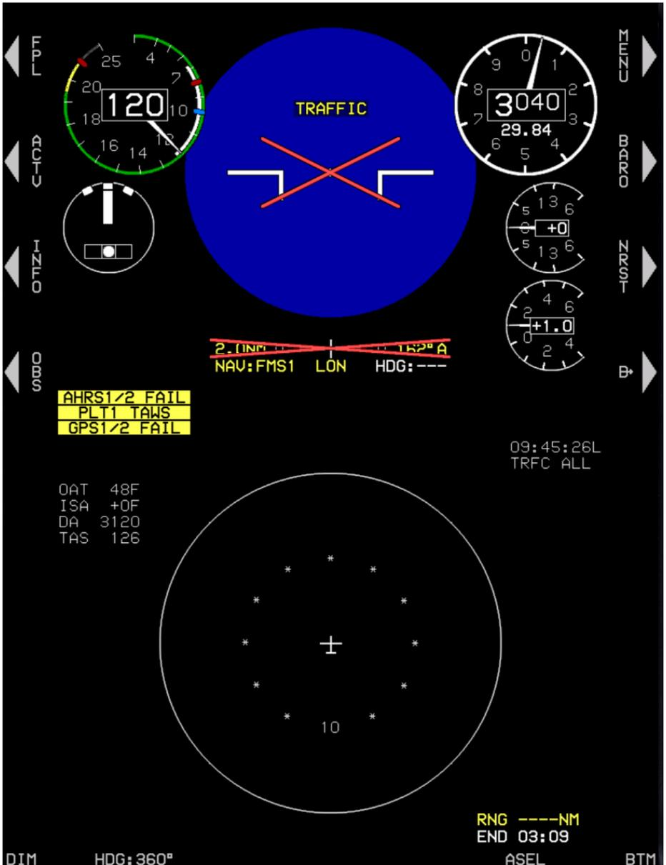
**Figure RD-46: PFD Failure Mode 5
