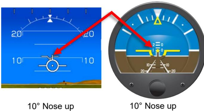
**Figure 3-33: Pitch Scale**
