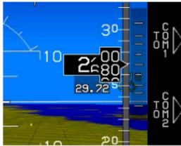
For remote tuning, **TO COM1 (R2)** and/or **TO COM2 (R3)** is shown to allow transmission of the frequency to remote radios when frequencies greater than or equal to 118 MHz are highlighted in the INFO block.
