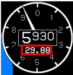
The altimeter setting digitally displays the altimeter setting in either inches of mercury (inHg) or millibars (mbar) according to the pilot-selected units.
