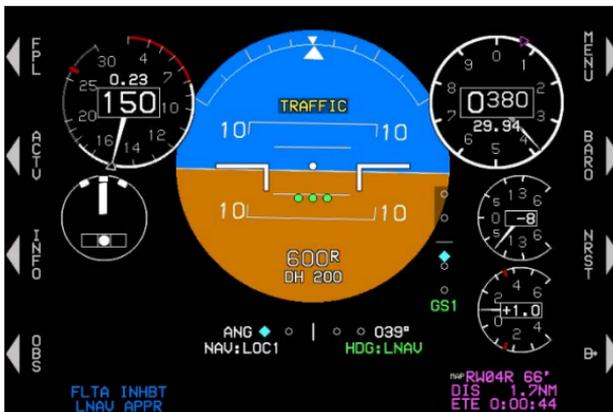
**Figure RD-37: EFIS Coupled Vertically with Glide Slope Mode**
