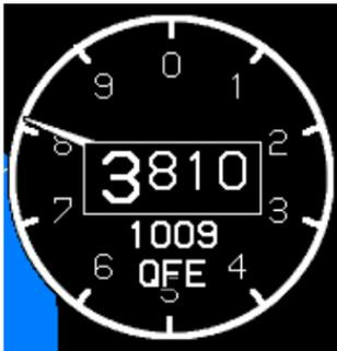
The altitude readout digitally displays barometric altitude to the nearest ten feet as adjusted by an altimeter setting and shows a 1000-foot range with labels and graduations every 100 feet. Clockwise rotation of the pointer corresponds to increasing altitude. All graduations are removed when below sea level.
