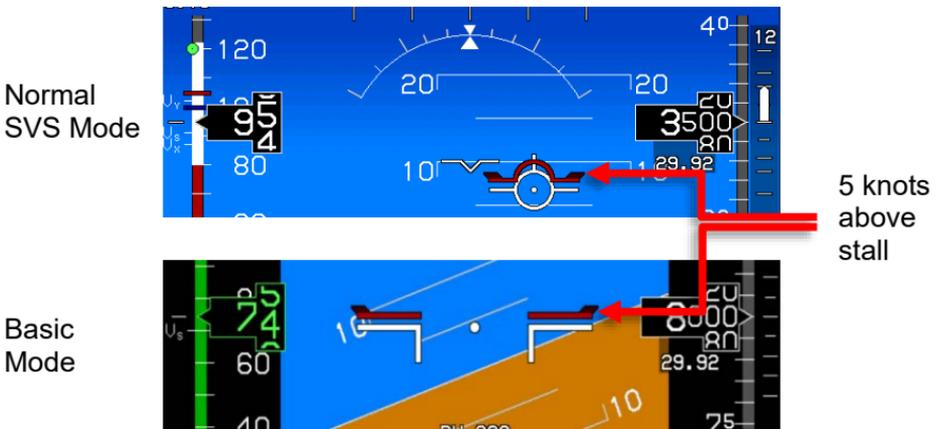
Figure 3-36: Pitch Limit Indicator (5 Knots above Stall)
