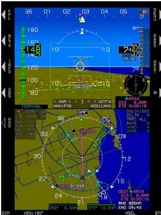
**Figure 2-9: PFD PFI on Top and Map on Bottom**
