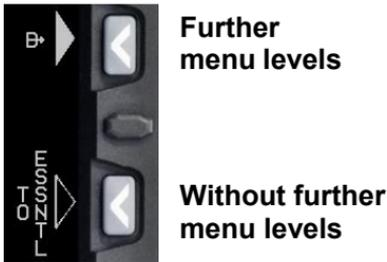
Soft menu function tiles appear in the margins next to IDU buttons and indicate further menu levels with a filled triangle or no further menu levels with a hollow triangle. The triangles point to the associated button.
