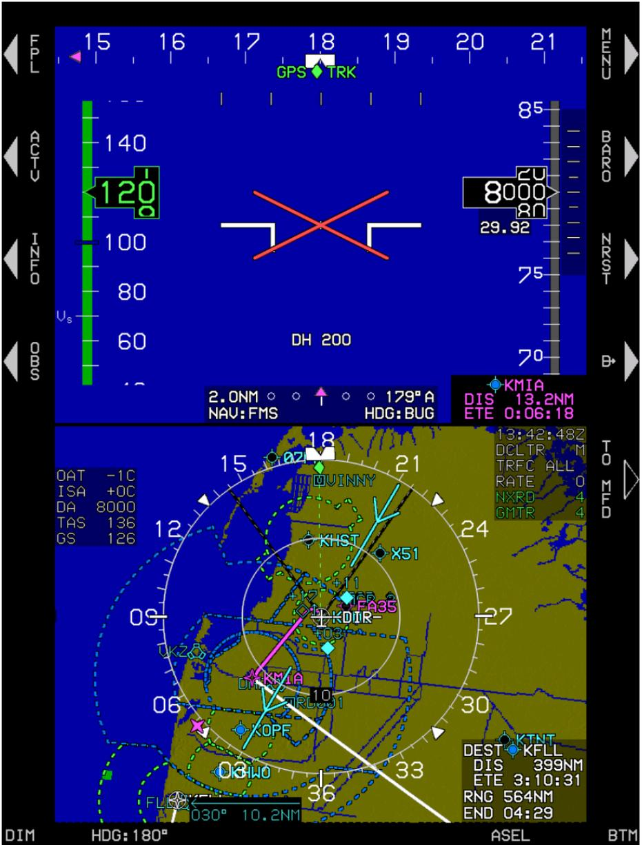
**Figure 4-17: MFD Failure Mode 3 (Essential Mode)
