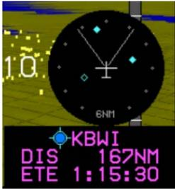
When selected from declutter options, **MINI TRFC** ✓, thumbnail is displayed in the lower right corner of the PFI area of the PFD above the active waypoint identifier and has clock face markings fixed at the 6 NM scale.
