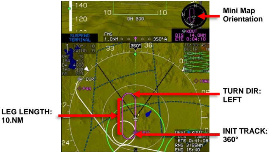
Figure SAR-14: Race Tack Pattern-Turn, Leg, and Track
