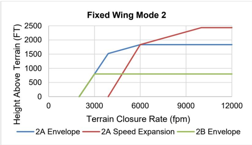
**Figure 8-10: Fixed Wing GPWS Mode 2**
