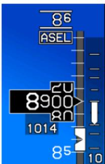
When an autopilot is not installed, the selected altitude is a reference only. The target altitude bug setting is white, and the target altitude bug is filled-white at all times.
