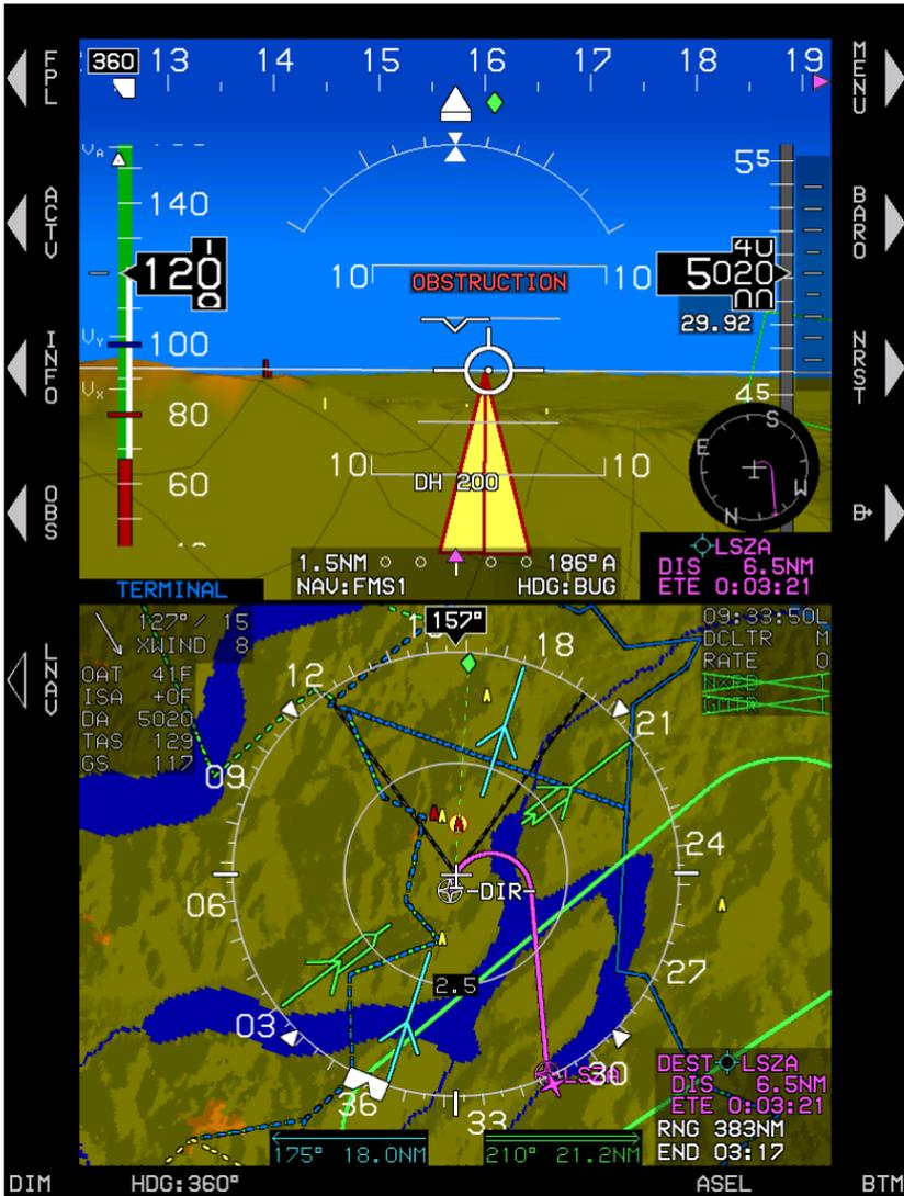
Obstruction within TAWS FLTA warning envelope with audible alert, "Warning Obstruction, Warning Obstruction." Obstruction symbols flash.
