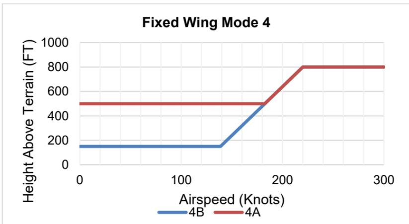
**Figure 8-13: Fixed Wing GPWS Mode 4**
