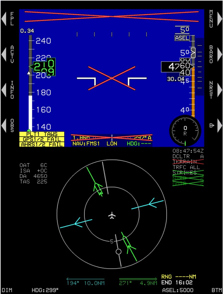
**Figure 4-21: PFD Failure Mode 5
