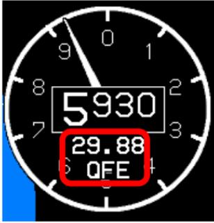
The mode is annunciated as QFE operations; otherwise, no mode is annunciated
