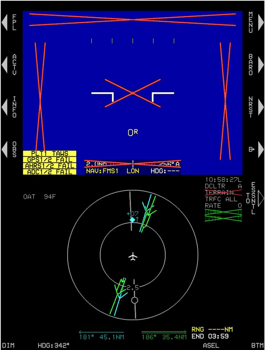
**Figure 4-27: PFD Failure Mode 7
