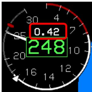
When enabled the Mach indicator is displayed above the airspeed readout with a resolution of .01 Mach.
