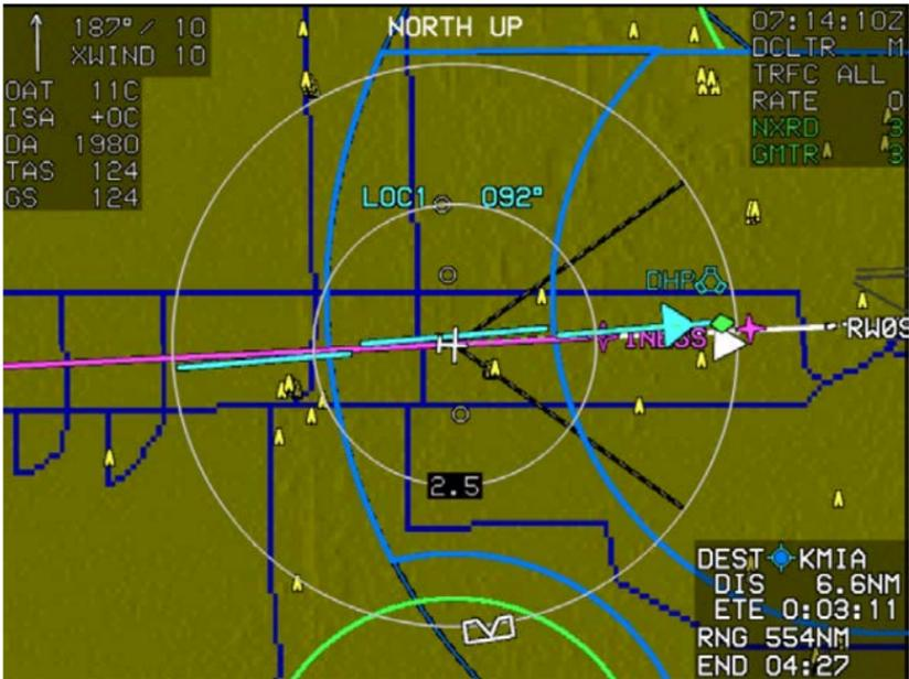
**Figure 3-70: North-Up Centered Mode with HSI Enabled and VLOC1 Selected**
