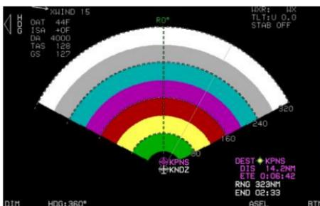
16) Rotate **1** to alter range of weather radar from 5.00 NM to 320.00 NM. Rotation direction dependent upon EFIS limits setting.
