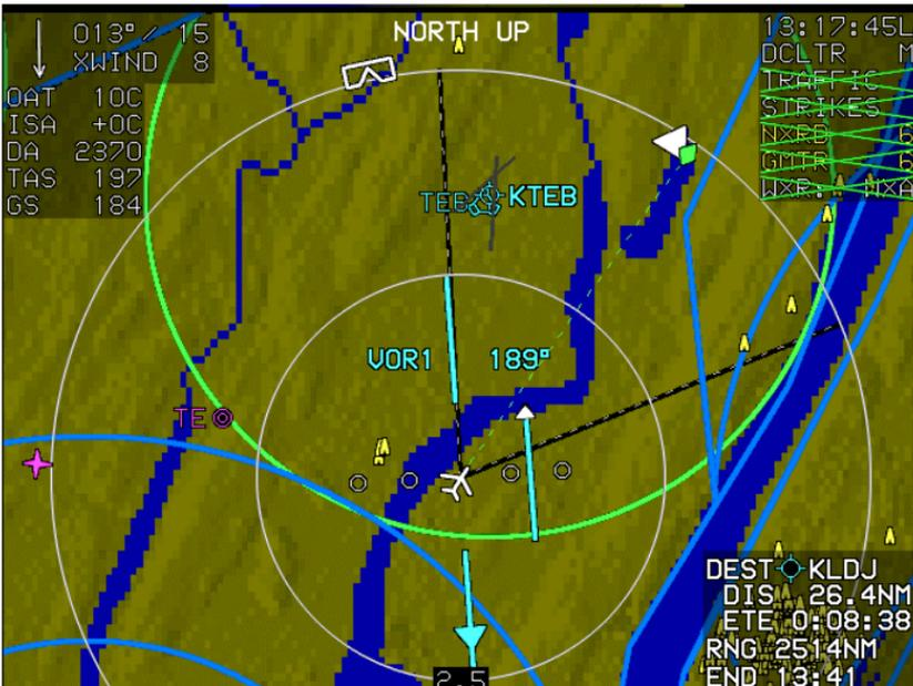
Figure 3-69: North-Up Arc Mode with HSI Enabled and VOR1 Selected
