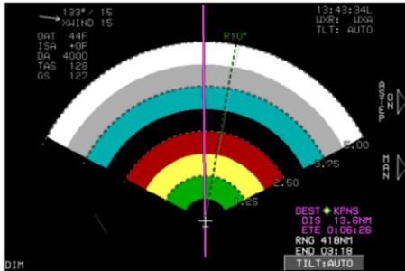
28) Press **ASTEP ON (R6)** or **ASTEP OFF (R6)** to toggle antenna tilt to sequentially step in  $4^\circ$  increments. (Auto step scan is entered initially by adjusting the tilt to  $+15^\circ$  or  $-15^\circ$ .)
