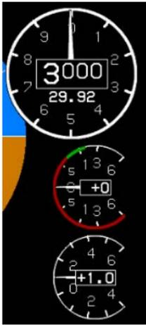
When TCAS-II is enabled, the background of the VSI functions as an RA display with green and red colored regions to provide RA maneuver guidance.
