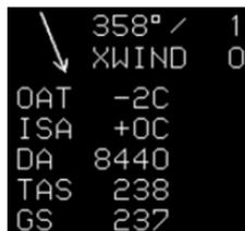
Figure S-3: Air Data and Ground Speed in Upper Left Corner
