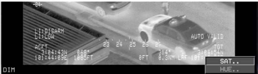
**Figure V-4: Video Page Saturation and Hue Setting**
