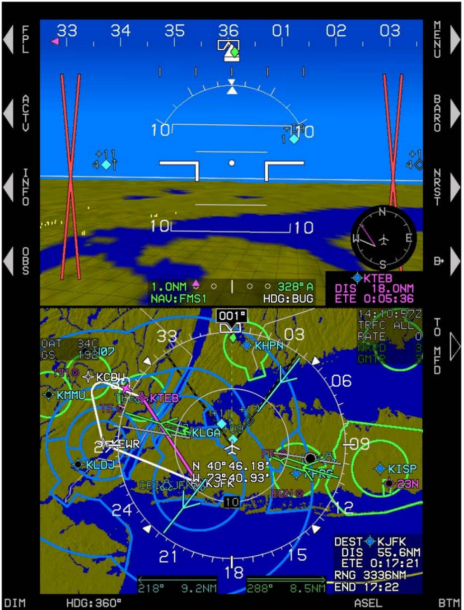
**Figure 4-14: MFD Failure Mode 2 (Essential Mode)
