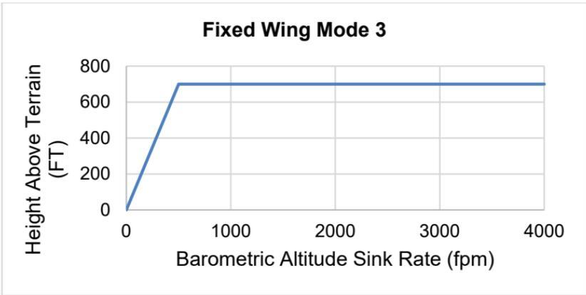
**Figure 8-12: Fixed Wing GPWS Mode 3**
