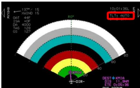
14) When in tilt auto mode, annunciation is above and in upper right corner of the top area.
