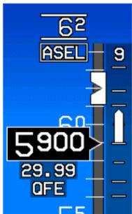
The altimeter setting is immediately below the altitude readout box and digitally displays the altimeter setting in either inches of mercury (inHg) or millibars (mbar) according to the pilot-selected units. Press **BARO (R2)** to enter altimeter setting mode and view the altimeter setting in inHg or mbar value in the lower right corner (Figure 3-13). Rotate **⬄** CW to increase or CCW to decrease the altimeter setting. Push **⬄** to enter the new value.
