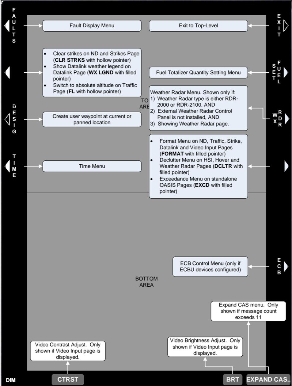
Figure 5-10: First-Level (MFD IDU #2) with an MFD Page in Both Areas (Normal Mode)
