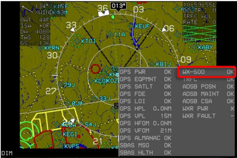
Figure S-10: MFD Fault Display Menu
