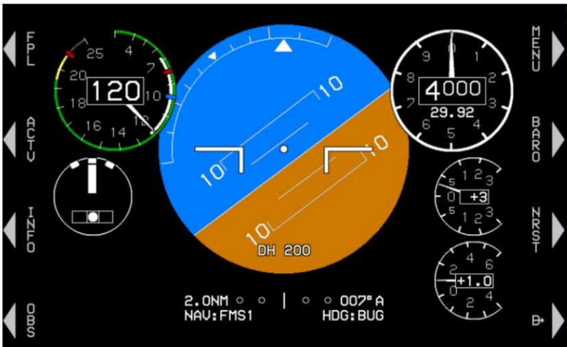
**Figure RD-5: Bank Angle Scale Roll Pointer Type**
