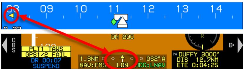
**Figure 3-32: GPS Loss of Navigation (LON)**
