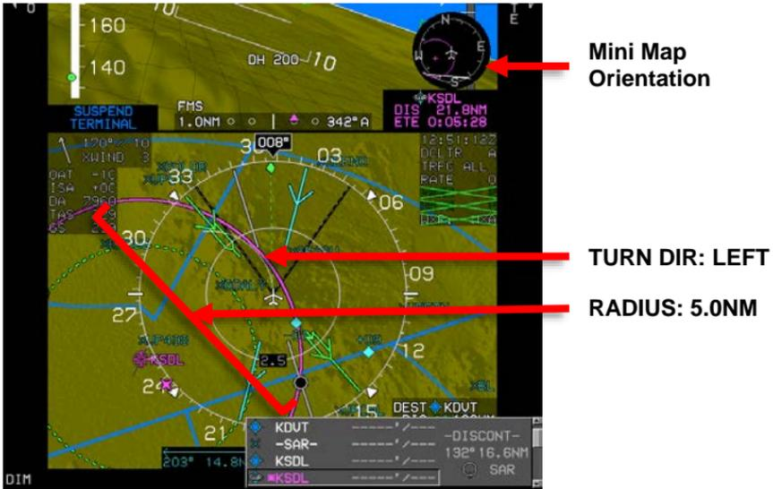
Figure SAR-11: Orbit Pattern-Turn and Radius
