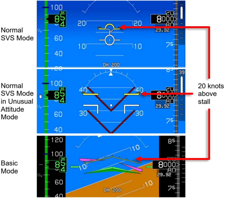
Figure 3-35: Pitch Limit Indicator (20 Knots above Stall)
