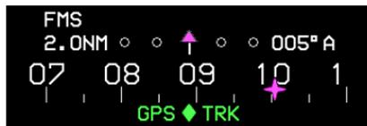
Figure RD-28: Heading Indicator with Heading Failure and Good GPS
