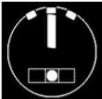
The turn rate indicator is displayed below the airspeed display. This standard “turn needle” displays marks representing a standard rate turn. The full scale for the turn needle is beyond the standard rate turn mark. This allows the pilot to fly a standard rate turn. The “balance ball” is driven from accelerometers within the AHRS.
