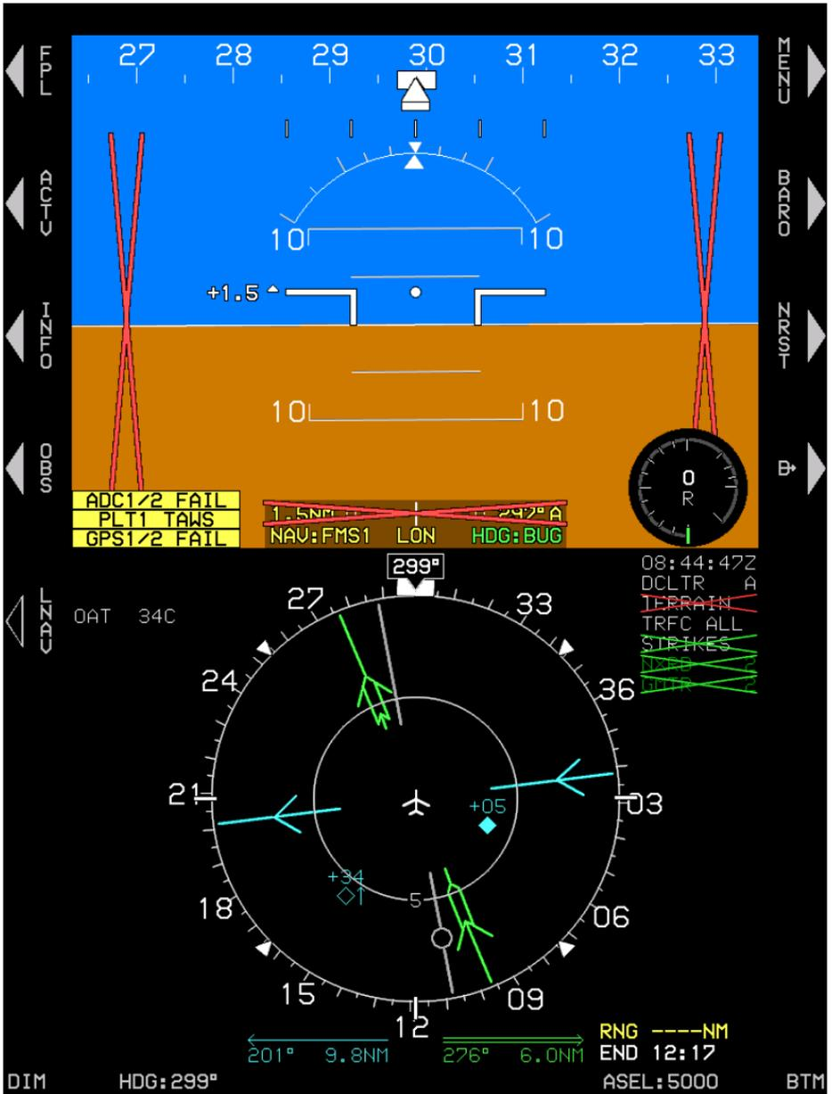
**Figure 4-18: PFD Failure Mode 4
