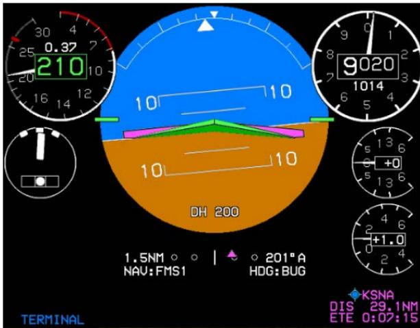
Figure RD-1: Pitch Scale
