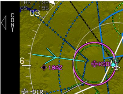
The SAR exit waypoint is a duplicate of the previous waypoint. This SAR pattern is unique in that the navigation path never goes through the waypoint. The path is a circle around the waypoint intercepted along tangents. With no other menus displayed on the PFD, **CONT (L6)** appears to allow for continuing out of the orbit and normal sequencing in the active flight plan.
