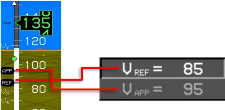
**Figure 3-27: Airspeed Indicator V-Speeds**
