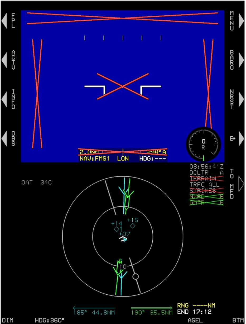
**Figure 4-29: MFD Failure Mode 7 (Essential Mode)
