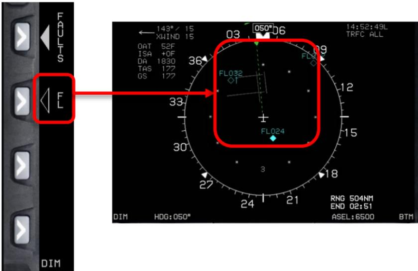
Figure T-14: Flight Level Option
