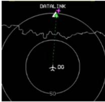
When not panning with AHRS in the DG mode, “DG” appears right of the ownship symbol. The datalink page is always displayed in a north-up orientation with a boundary circle in place of the compass rose. If not in pan mode, the ownship symbol is aligned with the aircraft heading.
