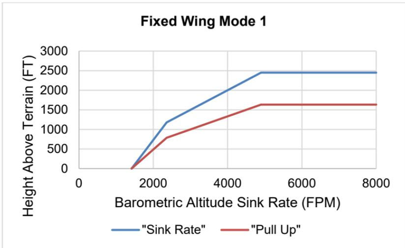
Figure 8-9: Fixed Wing GPWS Mode 1
