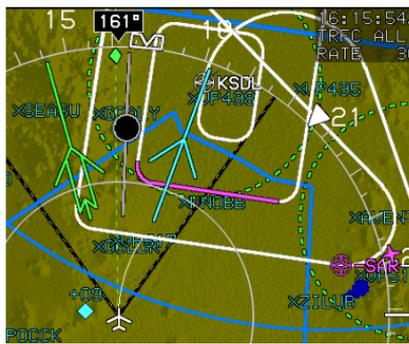
Figure SAR-4: Expanding Square Pattern-Individual Leg Selected
