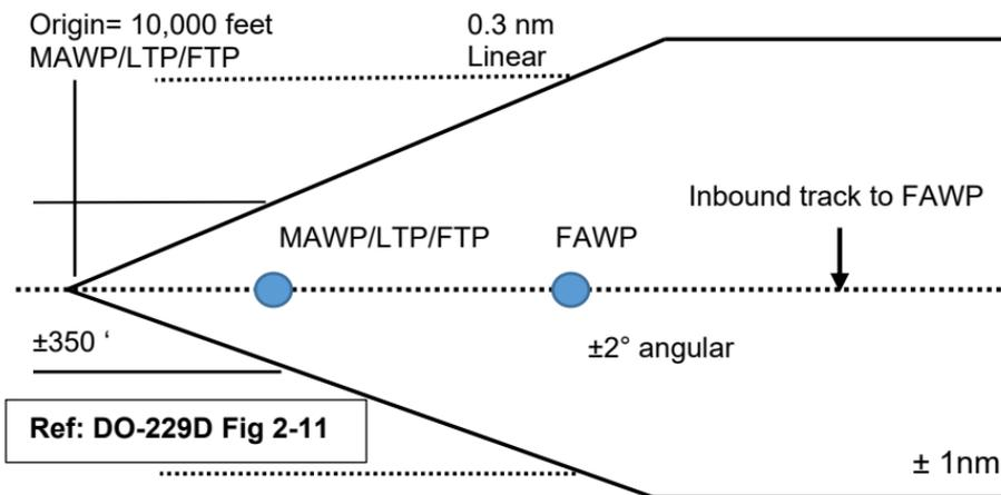
**Figure 7-16: FSD Lateral Deviation Indicator Linear Deviation VTF Approach**
