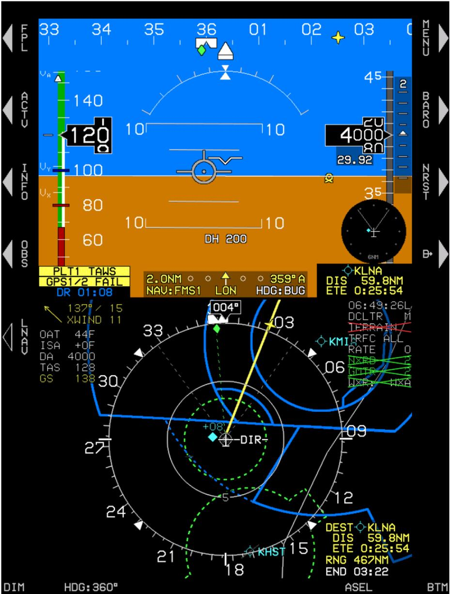
**Figure 4-9: PFD Failure Mode 1
