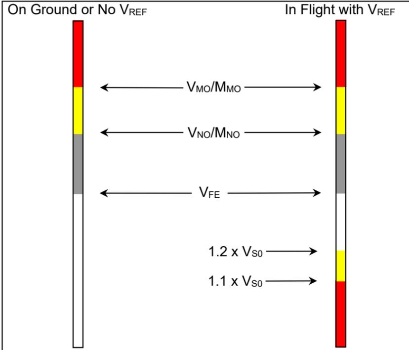
**Figure 3-29: Airspeed Scale FAR Part 25**
