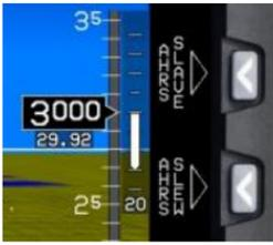
**AHRS SLAVE/AHRS DG (R2)** toggles between the two AHRS modes. **AHRS SLEW (R3)** enters a submenu to adjust the DG mode slewing value (if a DG/Slave input is not configured in EFIS limits for that AHRS.) When Genesys AHRS is installed and in DG mode without being configured in EFIS limits for the selected AHRS are not selected.
