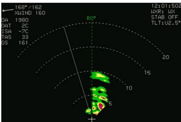
**Figure WX-5: Radar Image in Arc Format**
