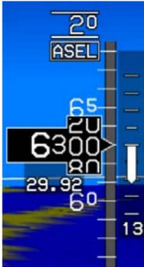
The vertical speed indicator (VSI) is depicted in a "worm" format providing analog and digital representation of VSI in feet per minute (fpm).
