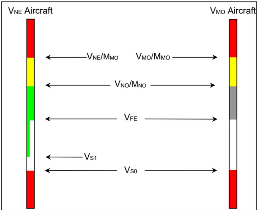
**Figure 3-28: Airspeed Scale FAR Part 23**
