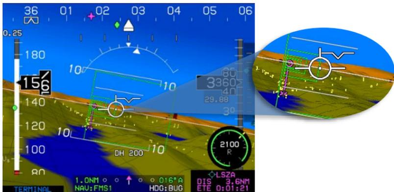
**Figure 3-47: Flight Path Marker**
