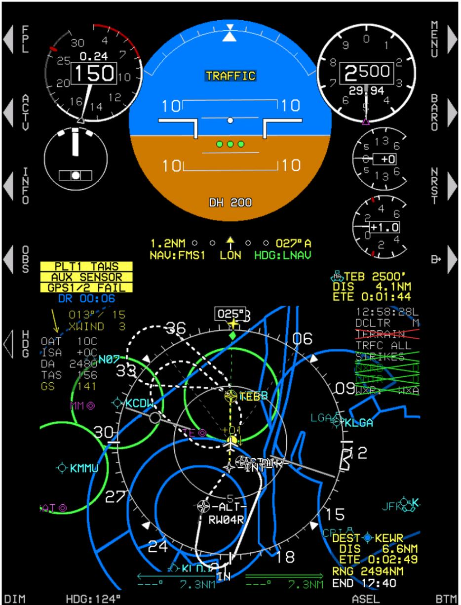
**Figure RD-42: PFD Failure Mode
