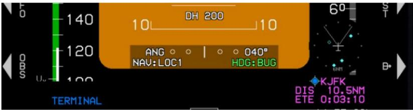
**Figure T-15: Basic Mode Mini Traffic**
