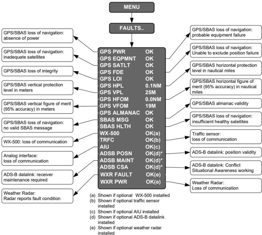
**Figure 5-32: MFD Fault Display Menu**
