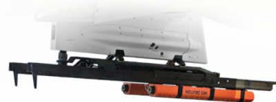
MISSILE SIMULATOR ON DUAL RAIL LAUNCHER
