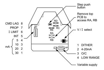
The servoamplifier consist of a number of functional blocks. Many of the blocks are configurable and there is some degree of flexibility in how the blocks are interconnected. The blockwiring diagram on page 5 shows each block and how they are interconnected.
