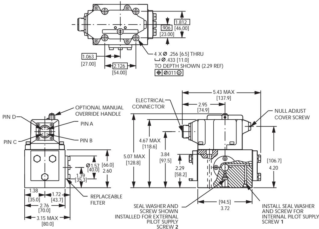
The mounting manifold must conform to ISO 4401-05-05-0-94\*
