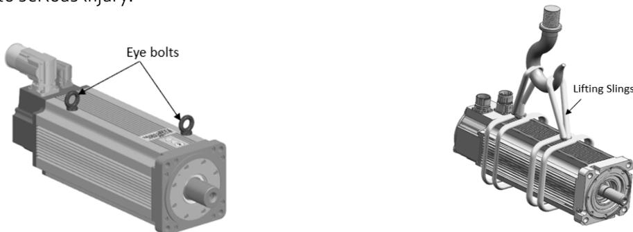
Figure 2: Lifting points (With and without eyebolt)
