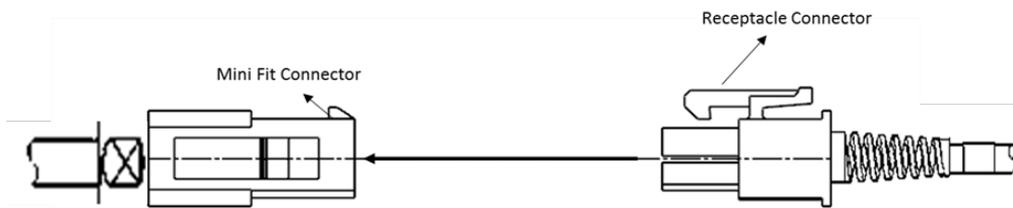
Figure 19: Fan connector with mating connector
