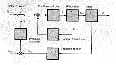
Flow control with superimposed pressure limiting control
