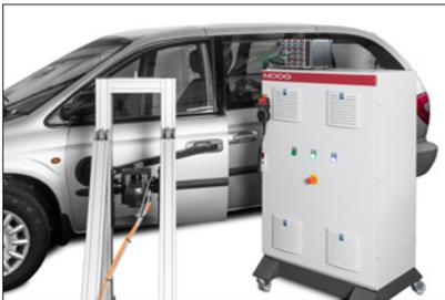
Closure tests are a vital part of measuring vehicle durability and quality. With the hood, door, sliding door, tailgate, decklid and more requiring cyclic durability regularly combined with hot/cold/humidity environments, Electric Multi-axis test systems can provide precise and repeatable position, velocity and force and record it all to provide reliability and confidence in your test results.
