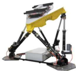
The human rated Electric Simulation Table, with the small Stewart platform footprint, incorporates electric actuators to deliver 6 degree-of-freedom motion. The test controller plays vibration spectra or time histories to provide exact control for comfort evaluation.
