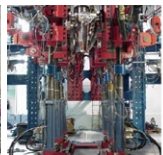
Landing Gear Structural Test
