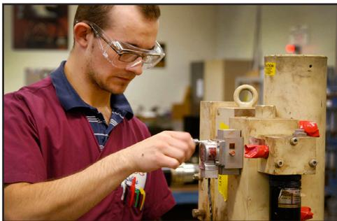
**Evaluate:** After initial receipt of actuator into repair facility technician breaks it down, logs in the parts and readies for refurbishment
