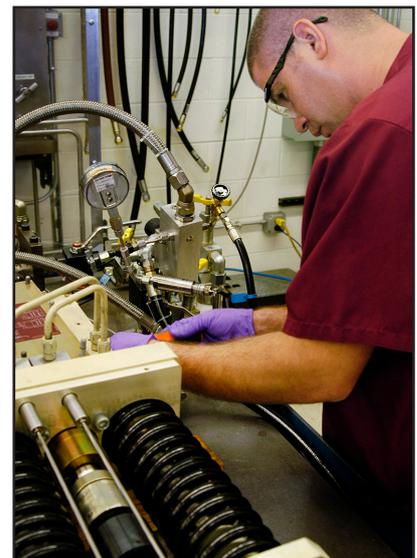
**Test:** Technician working on finished actuator on test bench to assure it meets or exceeds original OEM specifications before sending it back to customer
