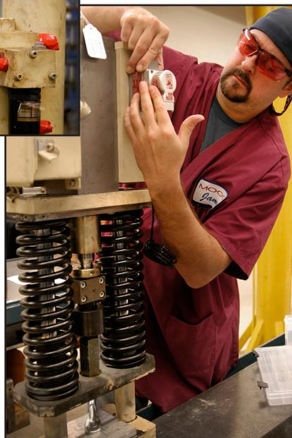
**Repair:** Technician cleans, repairs and reassembles each actuator
