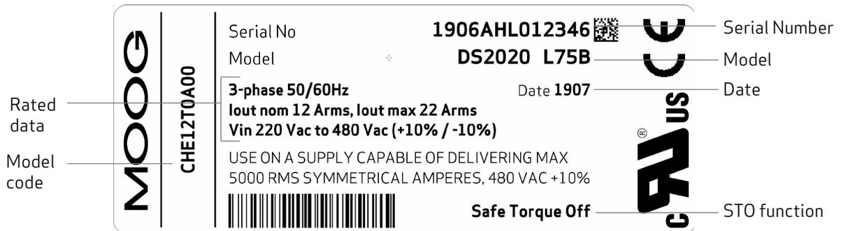
Figure 3: Example Drive Plate
