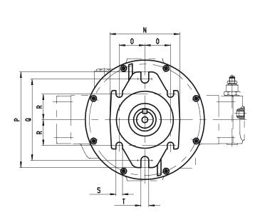
Key to SAE Standard SAE flange according to ISO 3019/1 (imperial dimensions)
