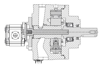
Radial piston pump with tandem-mounted gear pump using SAE-B adapter
