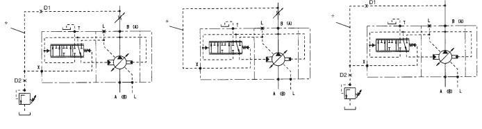
Pressure and flow compensation "load sensing"
