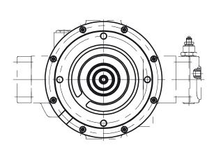
Involute spline according to DIN 5482 (for B1) (obligatory with multiple arrangement of RKP and SAE-B) Metric round flange
