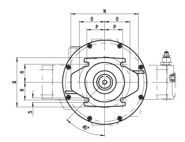
Involute spline according to DIN 5480 (obligatory with multiple arrangement of RKP and SAE-B) ISO flange according to ISO 3019/2 (metric dimensions)
