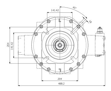
Straight key according to ISO 2491 ISO mounting flange to DIN ISO 3019/2 (metric dimensions)
