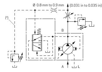
When high dynamics are required for flow control, adjust orifice and control line accordingly.
