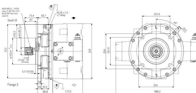
Involute spline according to SAE 744 C (for RKP mounting obligatory) SAE mounting flange to DIN ISO 3019/1 (imperial dimensions)
