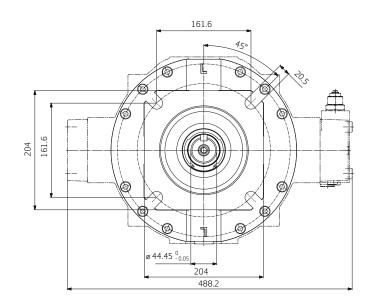
Key to SAE Standard SAE mounting flange to DIN ISO 3019/1 (imperial dimensions)
