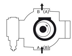
Note: Except for RKP 19 Counterclockwise rotation: Suction port (B) Pressure port (A)
