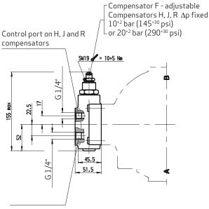
Tank connection on R compensator
