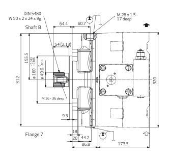
Involute spline according to DIN 5480 (for RKP mounting obligatory) ISO mounting flange to DIN ISO 3019/2 (metric dimensions)
