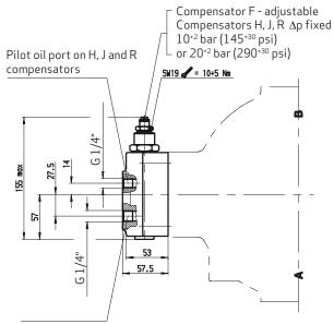
Tank connection on R compensator
