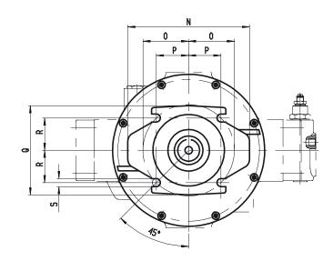
Involute spline according to SAE 744 C (obligatory with multiple arrangement of RKP and SAE-B) SAE flange according to ISO 3019/1 (imperial dimensions)
