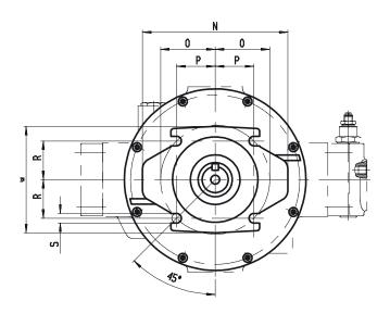
Straight key according to ISO 2491 ISO flange according to ISO 3019/2 (metric dimensions) HFA pumps have an unplugged inspection hole in the drive flange which must always be located at the bottom. If necessary, the mounting flange must be rotated.
