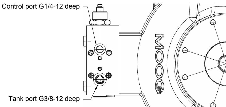
Figure 2: R1 and R2-type compensator of the RKP-II, size 140 cm<sup>3</sup>/rev
