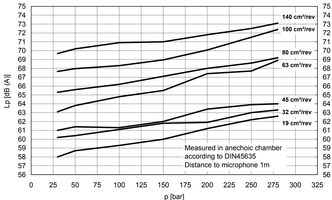
Figure 1: Noise pressure levels of the RKP-II with load sensing compensator J1
