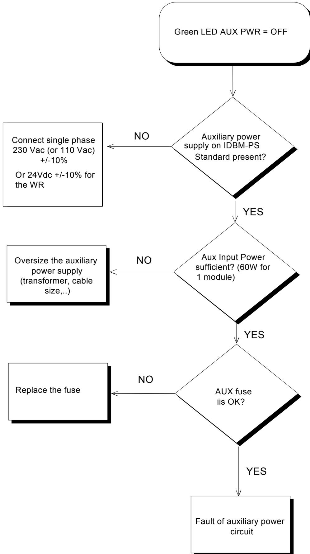
FIG. 6.5 - IDBM Module - POWER OK green LED off
