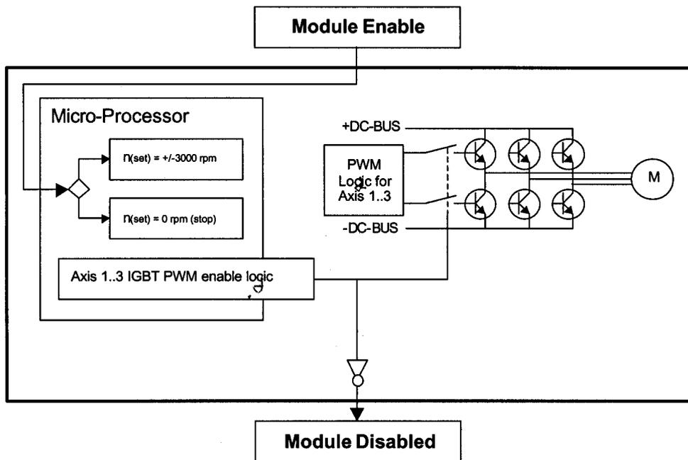
For observing Interlocking System III the input signal Module Enable and the output signal Module Disabled must be checked to have the appropriate status under the following conditions:
