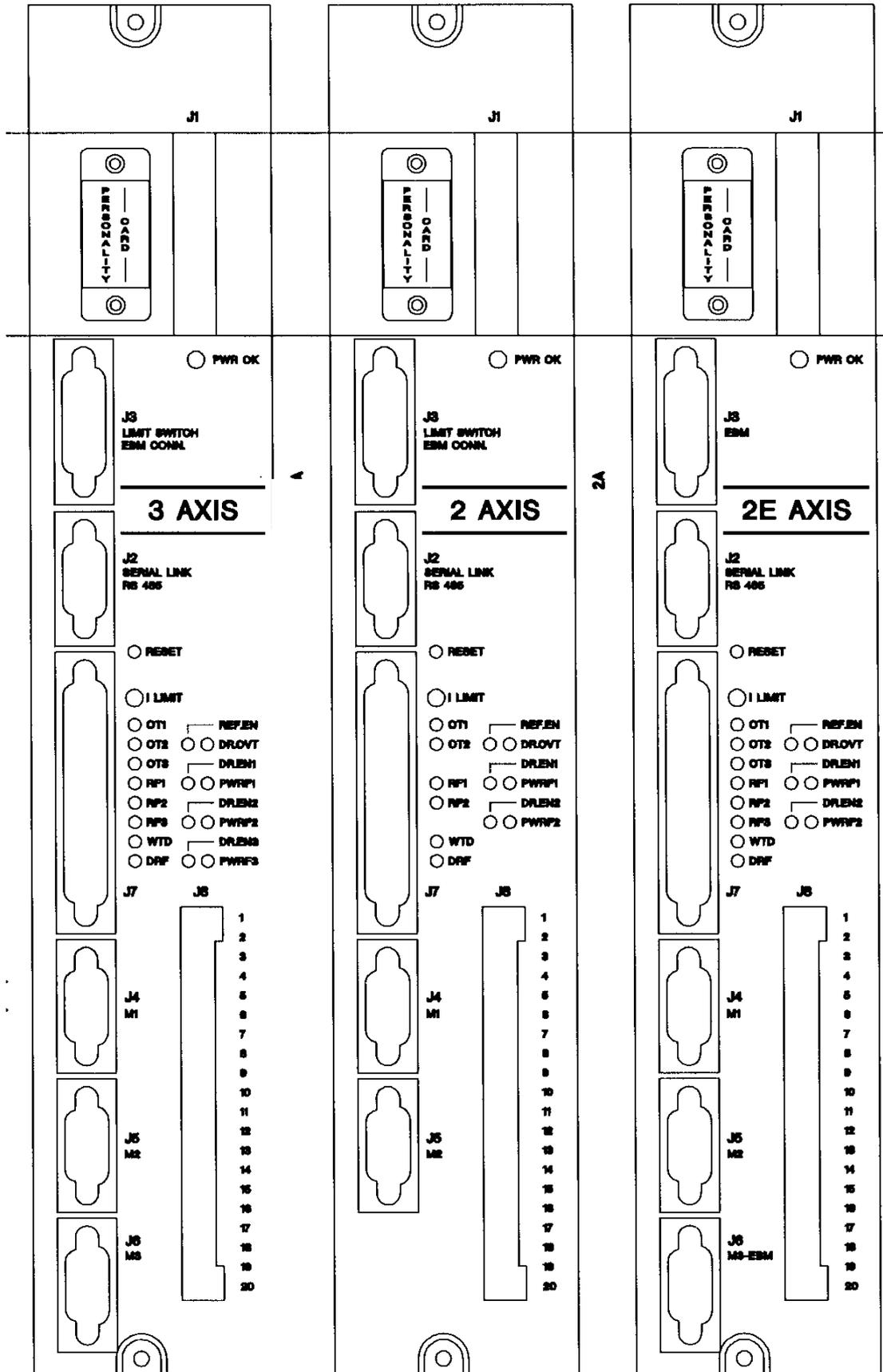
Fig. 2.6 Expansion-EBM - Removable Control Panel
