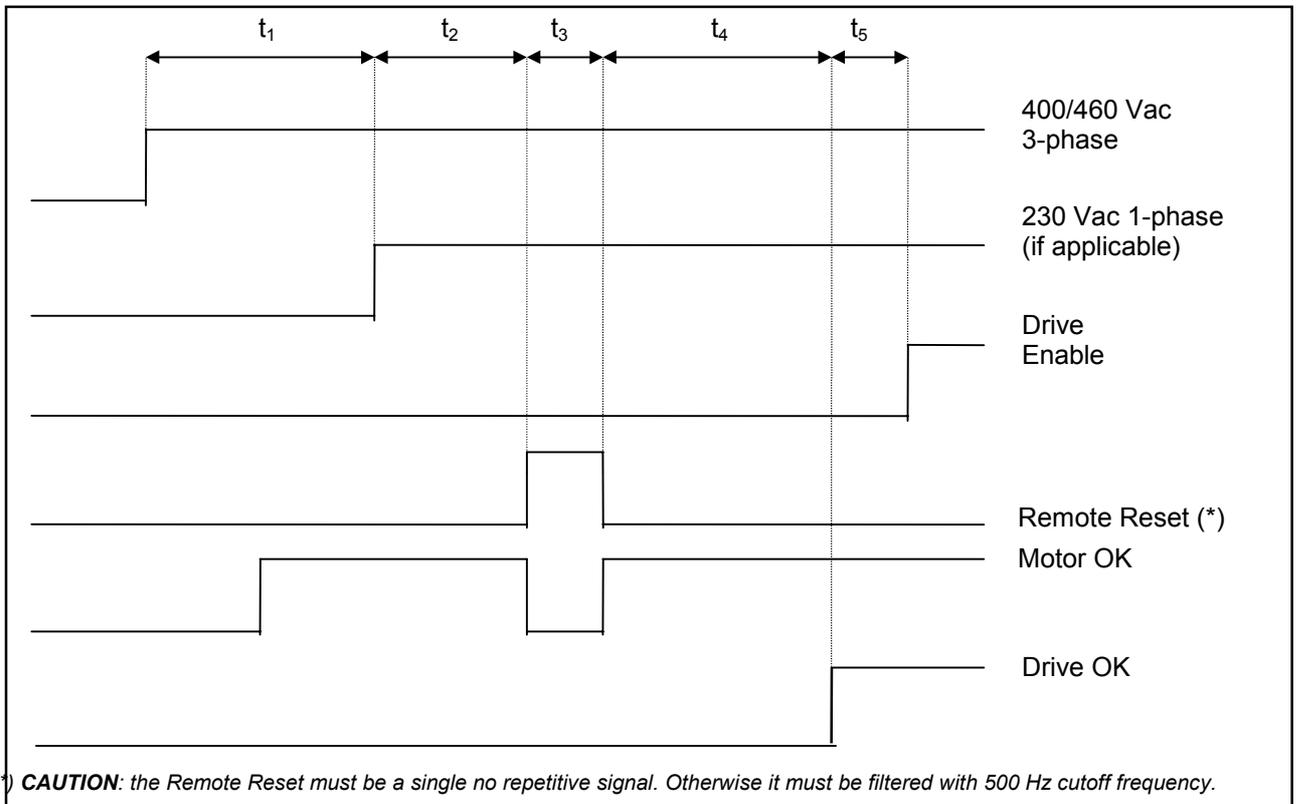
(\*) **CAUTION:** the Remote Reset must be a single no repetitive signal. Otherwise it must be filtered with 500 Hz cutoff frequency.
