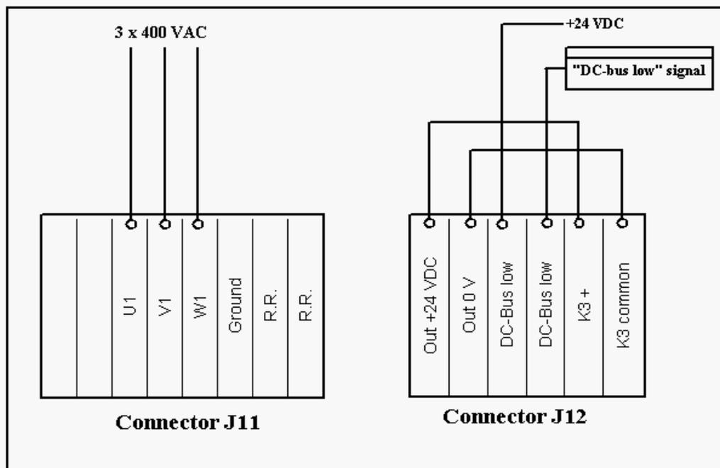
Fig. 2: Wiring Sample if no DC-bus discharge function is required
