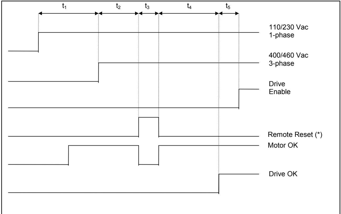
**2. PS-Standalone and PS-120:  $t_1 \geq 20$  ms,  $t_2 \geq 1$  s,  $t_3 \geq 20$  ms,  $t_4 = 3$  s,  $t_5 \geq 0.5$  s**
