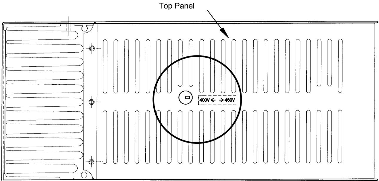
**CAUTION:** make sure that the correct wiring has been set for auxiliary input voltage on the PS-Standard and PS-6M front panel.
