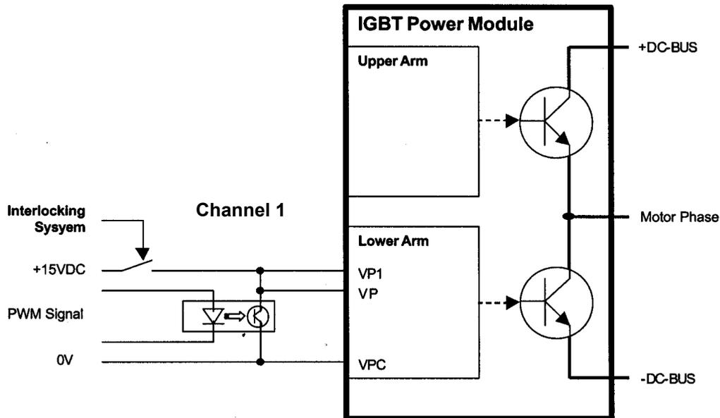
For observing Interlocking System II the input signal Channel 1 door (Lower Arm IGBT Enable) and the output signal Channel 1 verification (Lower Arm IGBT disabled) must be checked to have the appropriate status under the following conditions:
