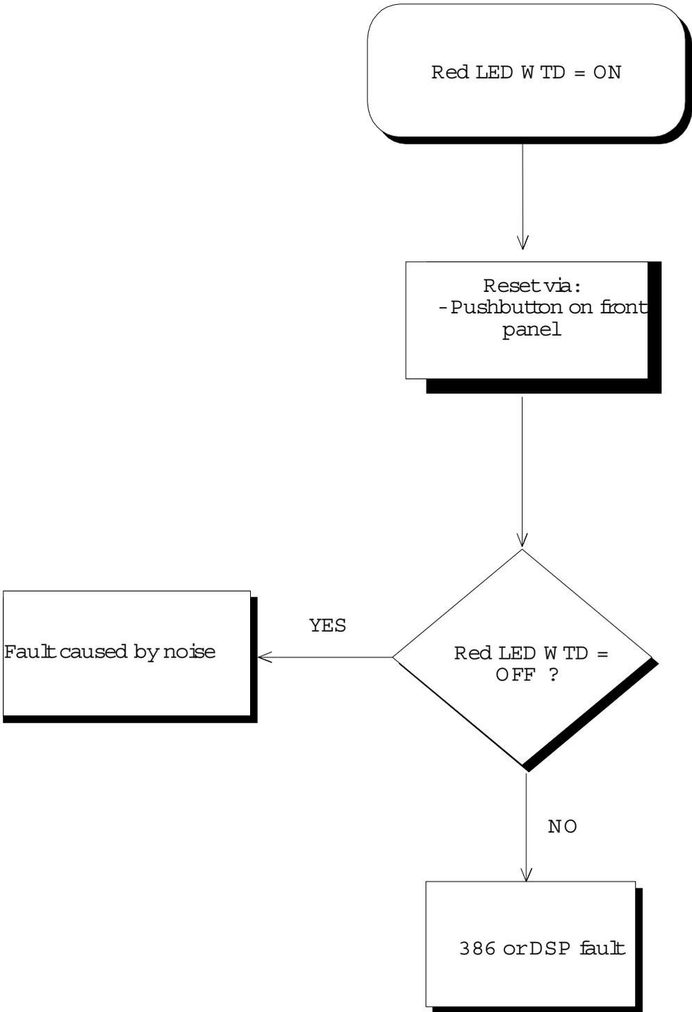
**FIG. 6.13 - IDBM Module - DRF red LED on Module Fault**
