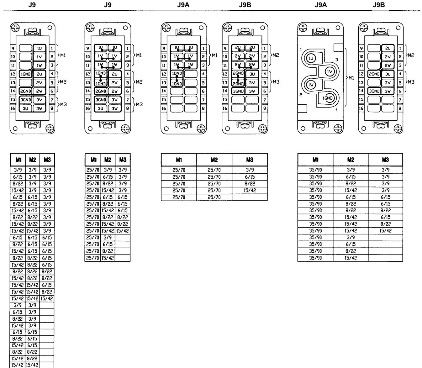
**Tab.2.22B - J9 Connector(s) - Motor Phases (2/2)**
