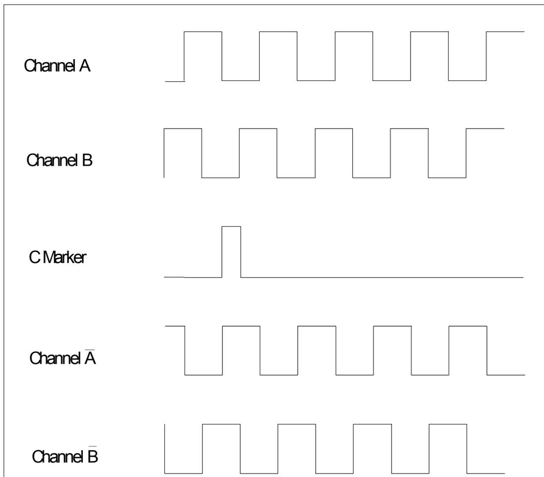
Note: to make C Marker high when Channel A and Channel B are high (like Siemens), swap Channel A with Channel  $\bar{A}$  and Channel B with Channel  $\bar{B}$ .
