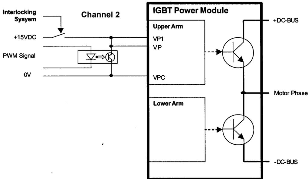
For observing Interlocking System I the input signal Channel 2 door (Upper Arm IGBT Enable) and the output signal Channel 2 verification (Upper Arm IGBT disabled) must be checked to have the appropriate status under the following conditions:
