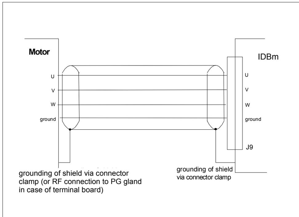
**Note:** All the motor phases must be connected from J9 connector(s) to motor connector(s). Note that M1 always corresponds to the more powerful axis, while M3 must not be connected in 2 axis configuration.
