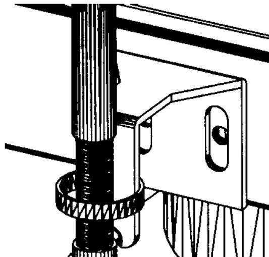
**Fig. 3.4 - Cable Grounding At Drive Side**
