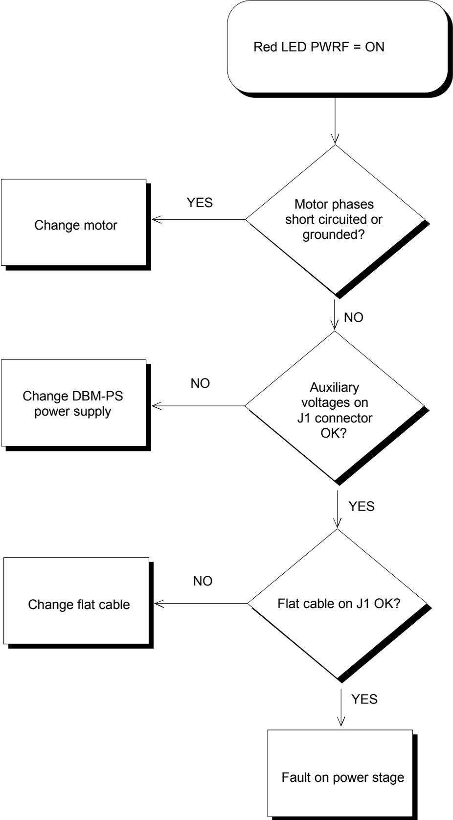
**FIG. 6.10 - IDBM Module - OT1/OT2/OT3 red LED on Motor Overtemperature Axis 1/Axis 2/Axis 3**
