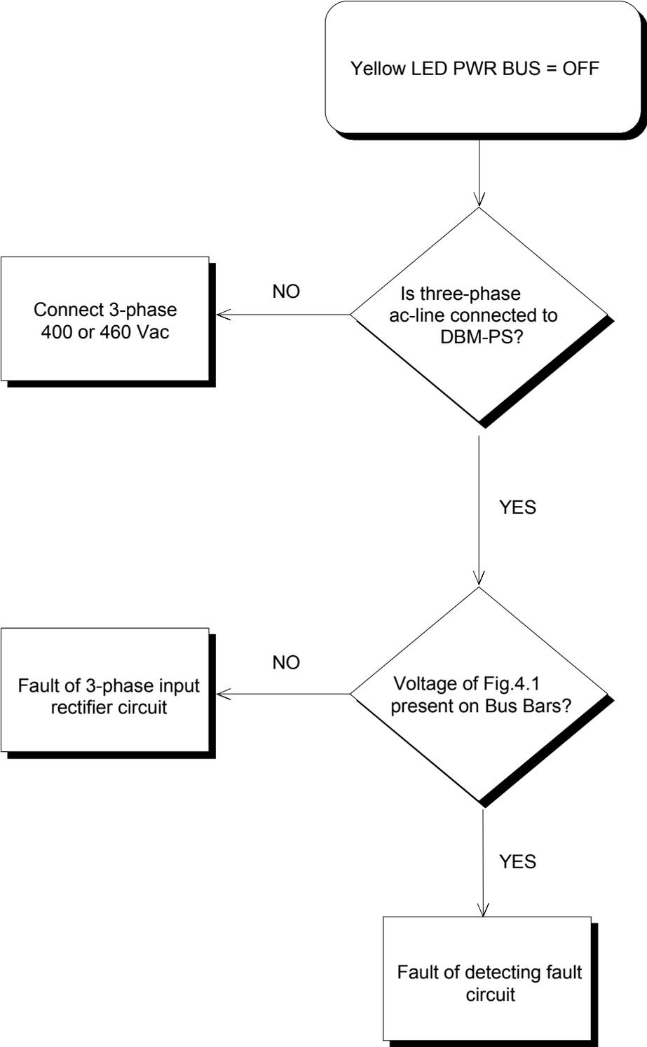
**FIG. 6.4 - IDBM PS-Standard and PS-6M Power Supply - AUX PWR green LED off**
