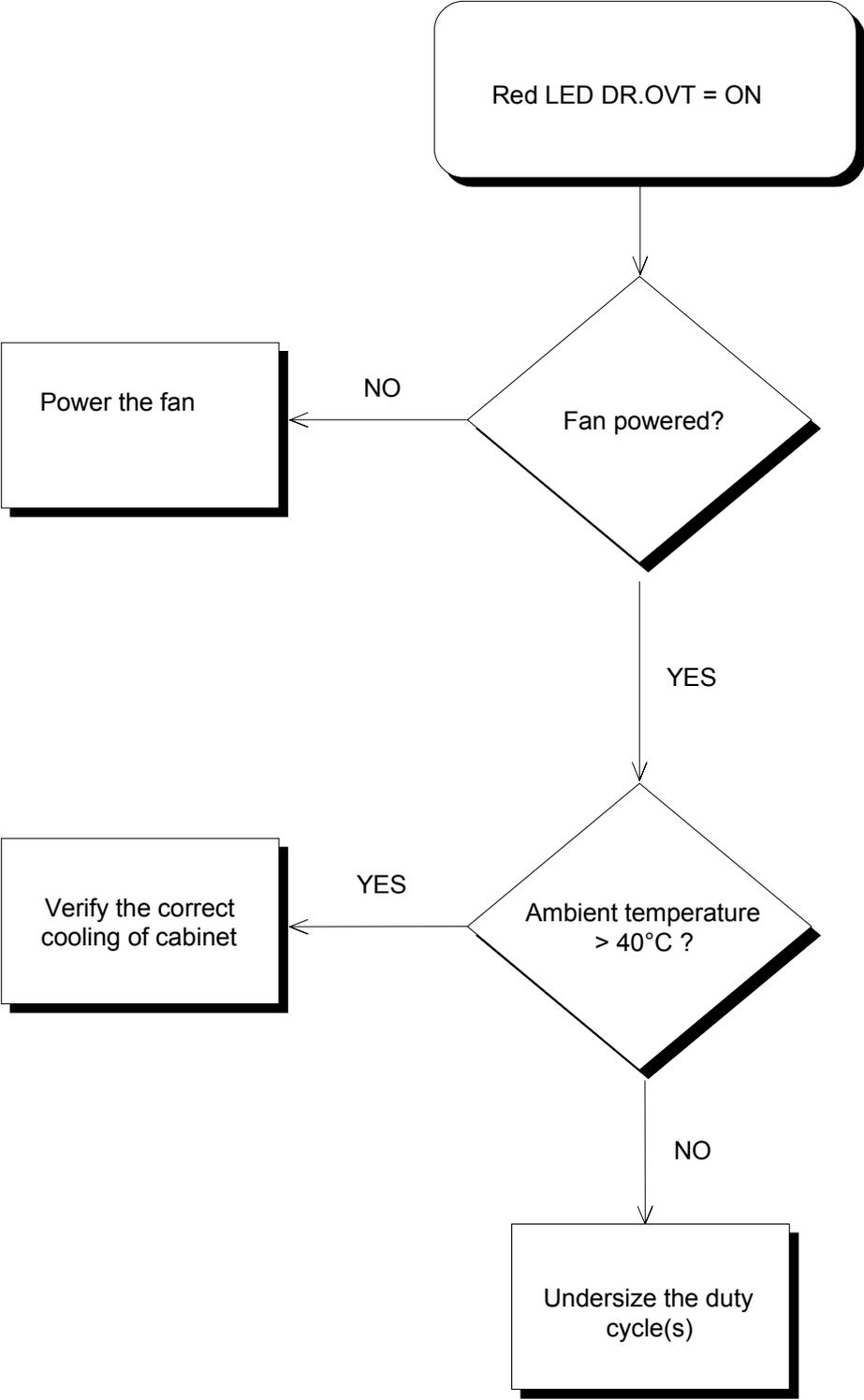
**FIG. 6.9 - IDBM Module - PWRF1/PWRF2/PWRF3 red LED on Power Circuit Fault Axis 1/Axis 2/Axis 3**
