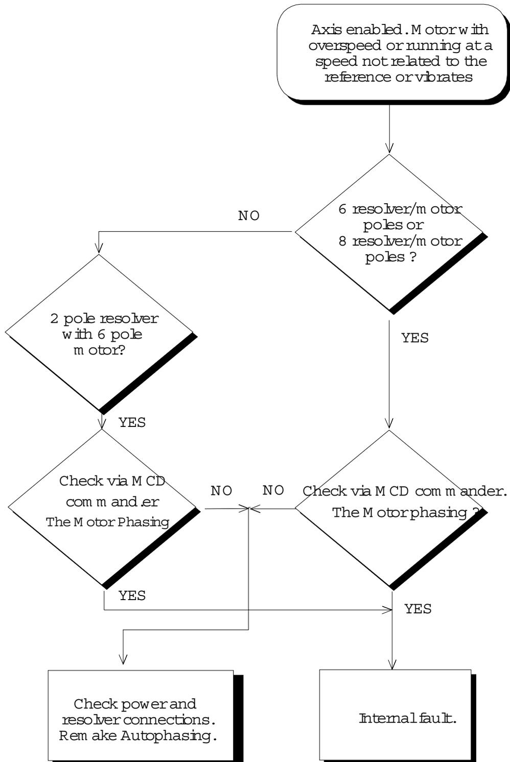
FIG. 6.15 – MCD Commander Fault
