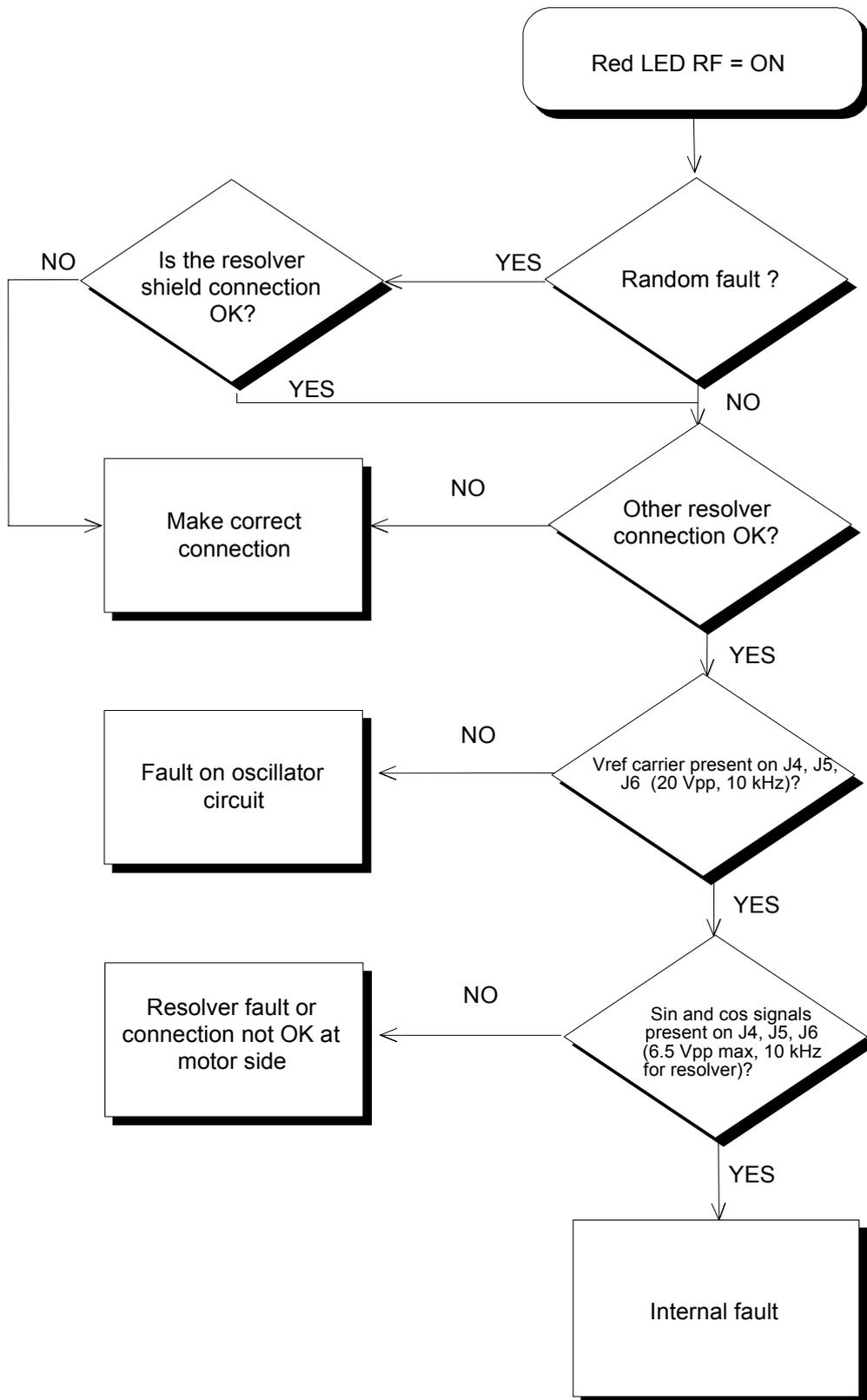
**FIG. 6.12 - IDBM Module - WTD red LED on Watch Dog**
