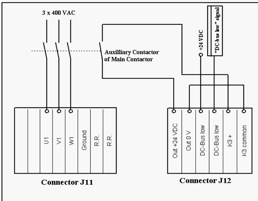
Fig. 1: Wiring Sample to discharge the DC-bus when powercontactor is disengaged
