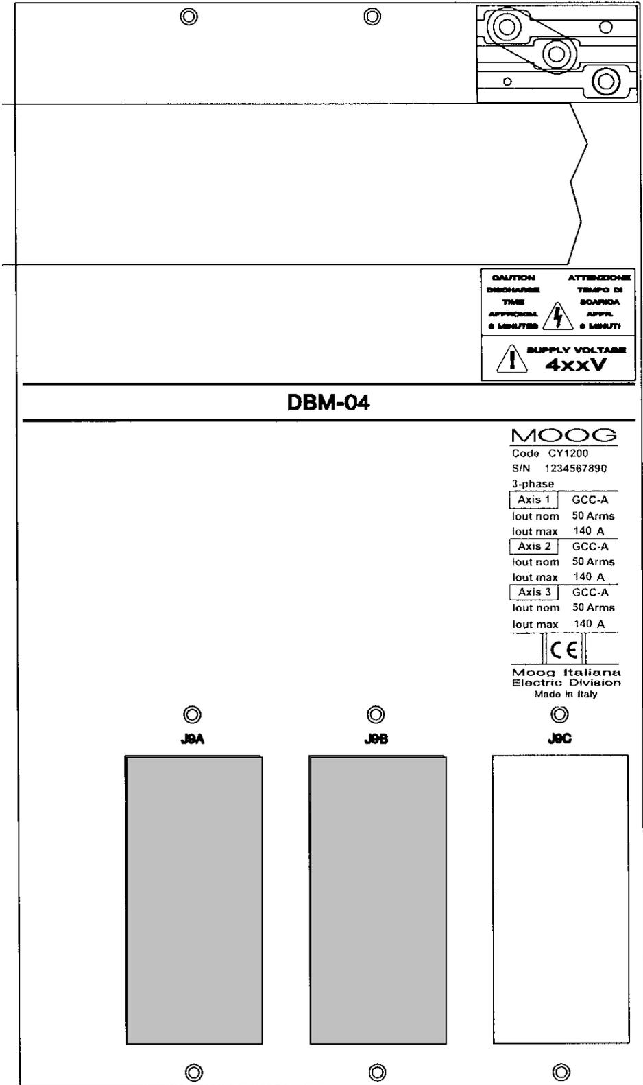
Note: the grey connectors are mounted only in some configurations (see tab.2.22)
