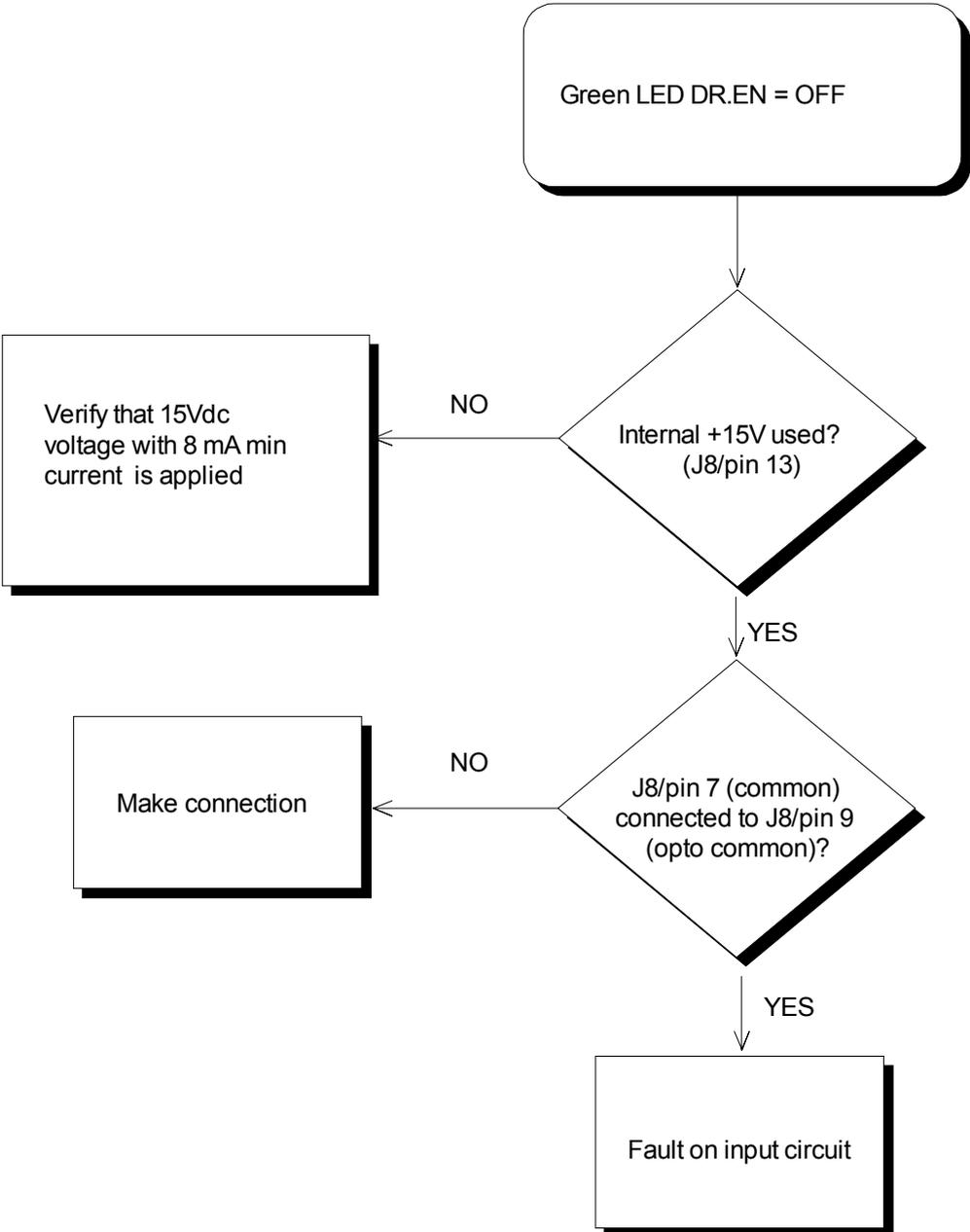
**FIG. 6.7 - IDBM Module - REF.EN green LED off
