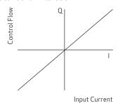
Minimal change in gain through null region. Best overall preformance for most closed loop systems.
