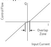
Null region flow gain is lower than normal. Spool types can range from minimal overlap to completely blocked flow.
