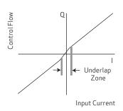
Null region flow gain is higher than normal. Always allows some small amount of flow past the spool.
