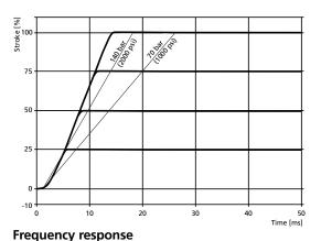
D674 with two-stage ServoJet<sup>®</sup> Pilot Valve D670
