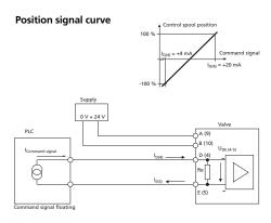
Conversion of the actual value output  ${\rm I}_{\rm outF}$  (Position of the spool) for valves with 6-pole + PE connector
