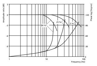
Typical characteristic curves at 210 bar (3000 psi) control or operating pressure, fluid viscosity of 32 mm<sup>2</sup>/s (cSt), oil temperature of 40 °C (104 °F)
