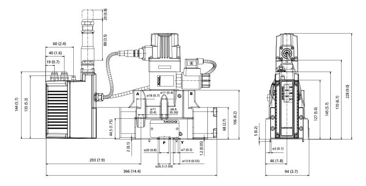
For space requirements of mating connector for various fieldbus systems see section "Electronics". The mounting surface must conform to ISO 4401-07-07-0-05 (see subsequent section "Mounting Pattern").
