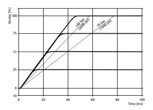
Frequency response D672 with ServoJet<sup>®</sup> Pilot Valve, Standard
