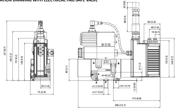
For space requirements of mating connector for various fieldbus systems see section "Electronics". The mounting surface must conform to ISO 4401-05-05-0-05 (see subsequent section "Mounting Pattern").
