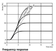
D671 with Direct Drive Pilot Valve D633, Offset
