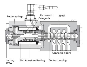
When returning to the center position, the spring force and the drive force act in the same direction. In the center position defined by the centering spring the linear force motor does not consume any current.
