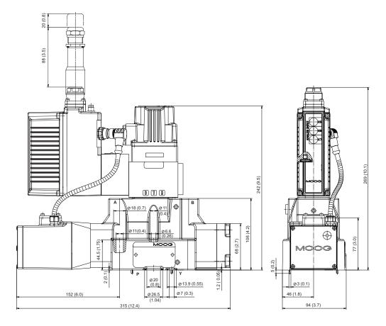
For space requirements of mating connector for various fieldbus systems see section "Electronics". The mounting surface must conform to ISO 4401-07-07-0-05 subsequent section "Mounting Pattern").
