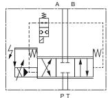
Hydraulics symbol: Presented with control pressure applied and electronics connected, supply of 2/2-way valve switched off.
