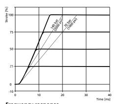
Frequency response D673 with Direct Drive Pilot Valve D633, Standard
