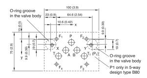
Ρ В т T<sub>1</sub> х Υ F<sub>1</sub> F4 [mm] Α F<sub>2</sub>  $F_3$ ([in]) Ø6.3 (0.25) Ø11.5 Ø11.5 Ø11.5 Ø11.5 Ø11.5 Ø6.3 M6 M6 M6 M6 (0.45) (0.45)(0.45)(0.45) (0.45)(0.25)37.3 16.7 50.8 54 54 27 3.2 -8 62 0 0 х (-0.31) (2.44) (2.13)(1.06) (0.66) (1.47) (0.13) (2.00) (2.13) 21.4 (0.84) 21.4 (0.84) 6.3 32.5 32.5 11 (0.43) 11 (0.43) 46 46 0 у 0 (0.25) (1.28)(1.81) (1.28)(1.81)
