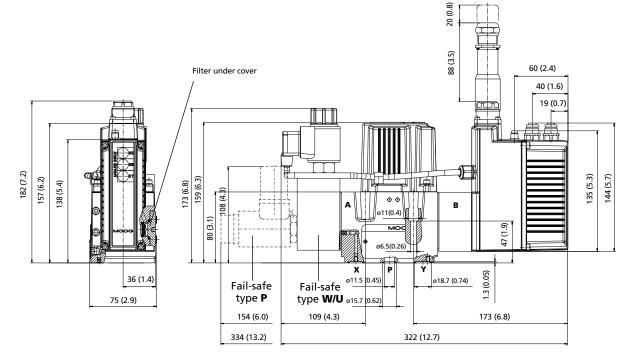
For space requirements of mating connector for various fieldbus systems see section "Electronics". The mounting surface must conform to ISO 4401-05-05-0-05 (see subsequent section "Mounting Pattern").
