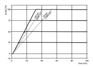
Frequency response D673 with ServoJet<sup>®</sup> Pilot Valve, High Flow
