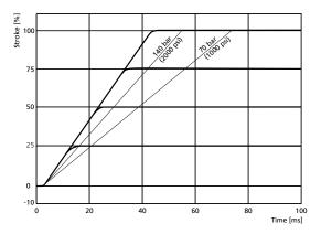
Frequency response D675 with Direct Drive Pilot Valve D633, Offset, standard spool P15
