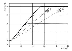
Frequency response D671 with ServoJet<sup>®</sup> Pilot Valve, Standard
