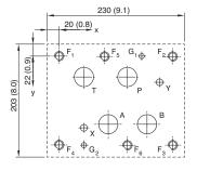
\* Dimension not according to ISO but EN 24340. The position of the mounted safety pin is according to EN. Hole G1 according to ISO is 138.6 mm (5.46 in) and it is drilled in the valve body in line with ISO.
