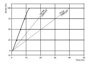
Frequency response D675 with two-stage ServoJet<sup>®</sup> Pilot Valve D671, stub shaft spool K15
