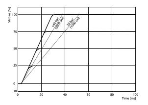
Frequency response D675 with Direct Drive Pilot Valve D633, Standard, standard spool P10
