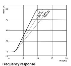
D672 with two-stage ServoJet<sup>®</sup> Pilot Valve D670
