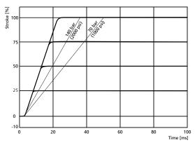
Frequency response D675 with two-stage ServoJet<sup>®</sup> Pilot Valve D671, standard spool P10
