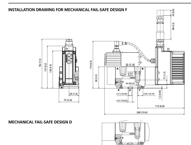
For space requirements of mating connector for various fieldbus systems see section "Electronics". The mounting surface must conform to ISO 4401-05-05-0-05 (see subsequent section "Mounting Pattern").
