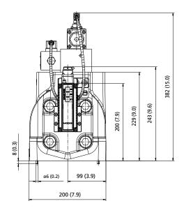
For space requirements of mating connector for various fieldbus systems see section "Electronics". The mounting surface must conform to ISO 4401-10-09-0-05 (see subsequent section "Mounting Pattern").
