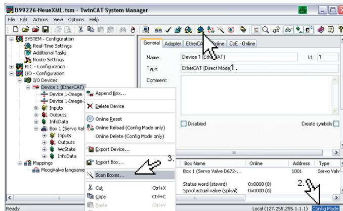
Figure 32: Scanning the network
