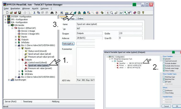
Figure 37: Linking the process data to the slave device/valves setpoint and actual values
