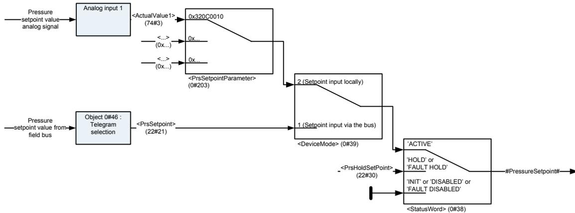
Figure 15: Pressure setpoint value path
