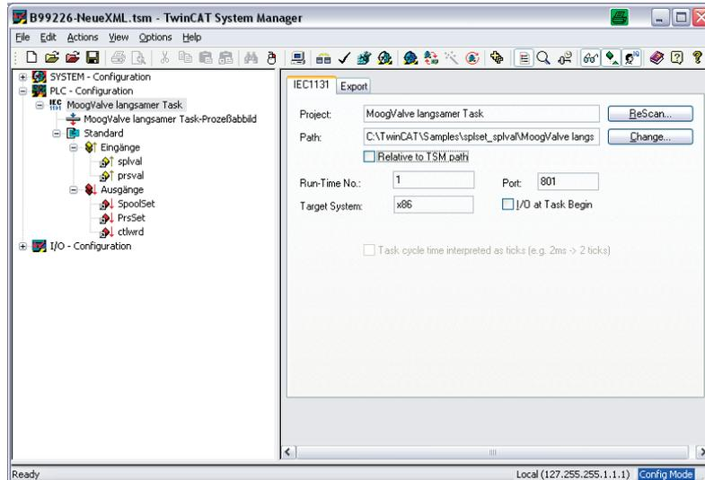
Figure 36: PLC configuration with PLC application parameters
