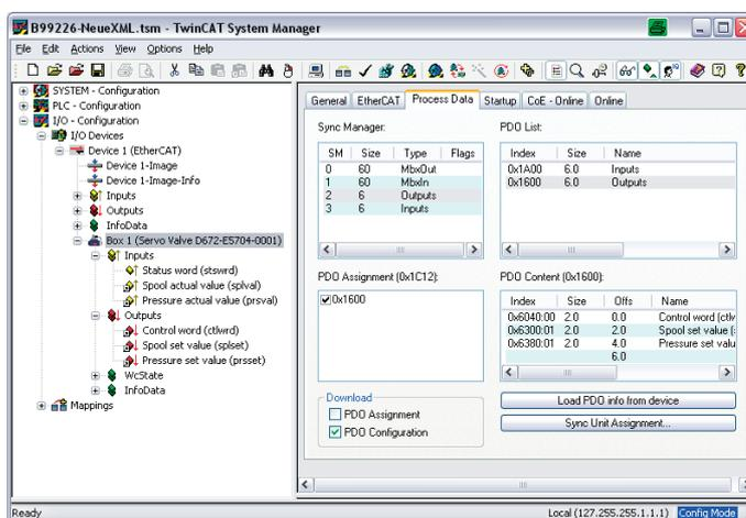
Figure 33: Process Data Objects (PDO) mapping
