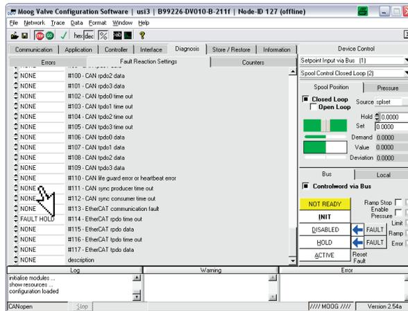
Figure 45: Configuring the fault reaction
