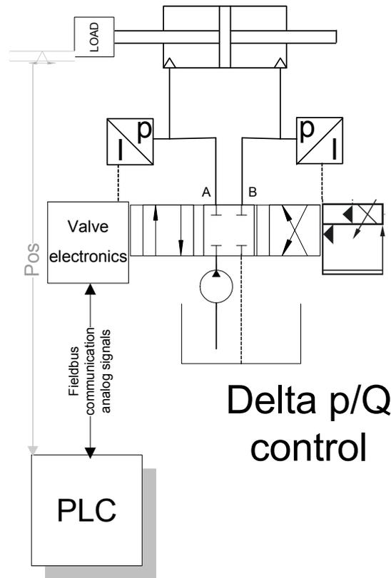
Figure 18:  $\Delta p$  control principle
