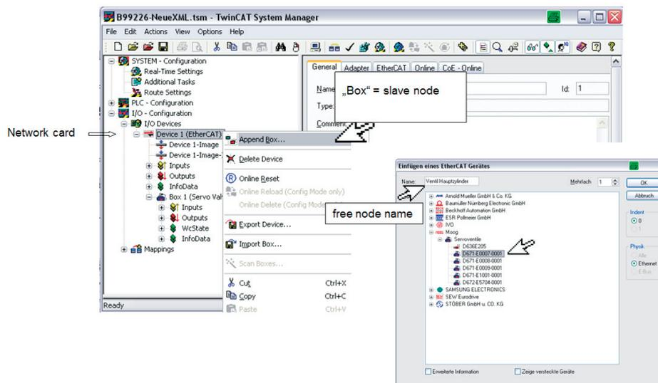
Figure 31: Inserting a network card
