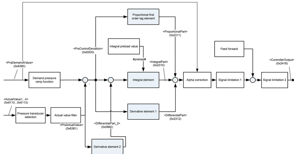
Figure 19: Pressure controller
