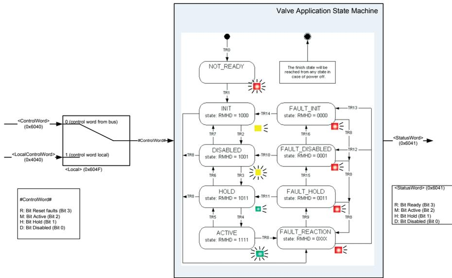
Figure 23: Device State Machine fault states
