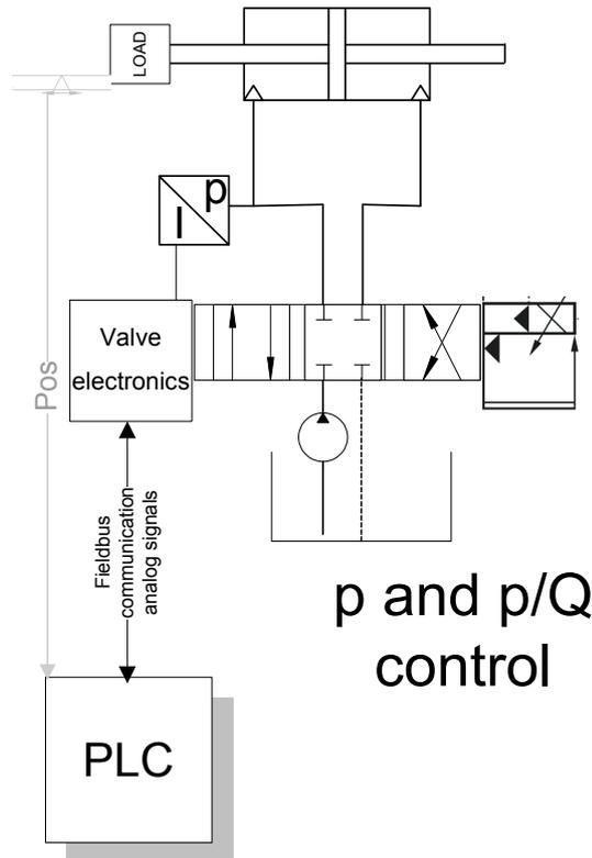
Figure 17: p and p/Q control
