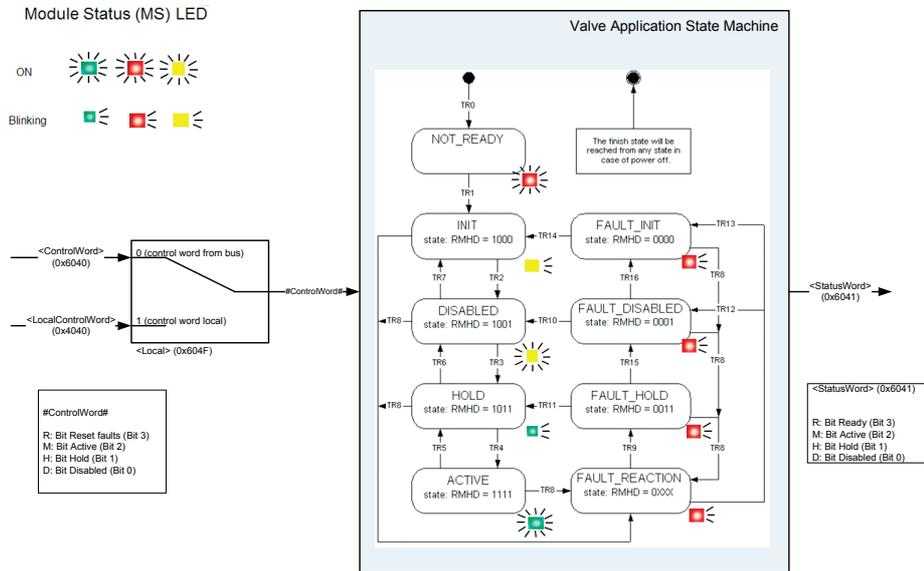
Figure 7: Device State Machine (DSM)
