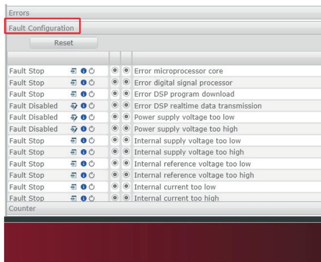
Figure 22: MoVaPuCo fault configuration
