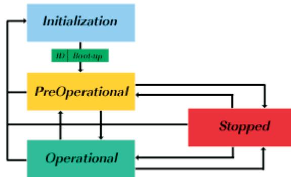
Figure 6: Network State Machine (NMT)
