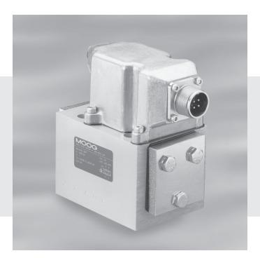
The flapper of the first stage hydraulic amplifier is rigidly attached to the midpoint of the armature. The flapper extends through the flexure tube and passes between two nozzles, creating two variable orifices between the nozzle tips and the flapper. The pressure controlled by the flapper and nozzle variable orifice is fed to the end areas of the second stage spool.
