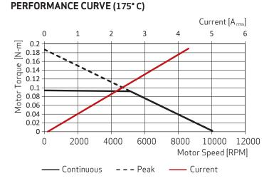
Operating Environment: Motor fully immersed in synthetic lubrication oil at 25,000 PSI (1,723 Bar) pressure and up to ambient temperature of 175° C (347° F).
