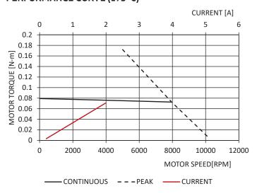
Operating Environment: Motor fully immersed in synthetic lubrication oil at 25,000 PSI (1,723 Bar) pressure and up to ambient temperature of 175° C (347° F).
