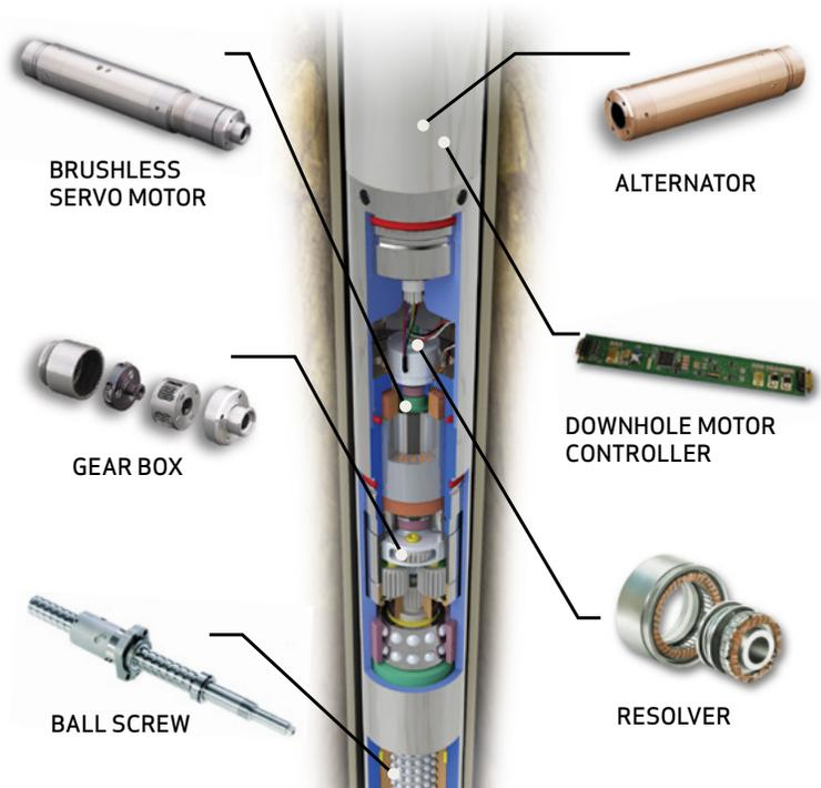
*Example of typical components designed and engineered specifically to create an optimal solution for extreme downhole environments*
