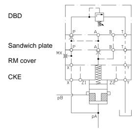
Valve configurations using a flow control sandwich plate, regardless of pilot valve; do not require any special sandwich plates.
