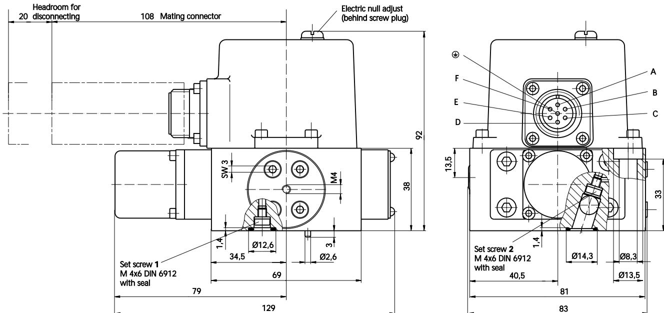
The mounting manifold must conform to ISO 10372-04-04-0-92.
