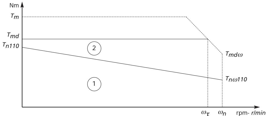
**T<sub>n110</sub>:** nominal torque, continuous duty, locked rotor
