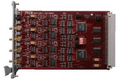
The Video 3 board supports four 10-bit digitized video channels. Unlike the earlier Video 1 and Video 2 Video boards, there are NO data channels physically on this board and thus there are no ribbon cable connectors. Also, unlike the Video 1 and Video 2 boards, the Video 3 board does not require a video sync in the signal to operate, thus it can be configured for passing analog data. There
