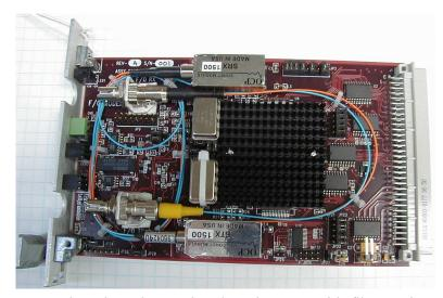
The Fiber Optic Modem board sends and receives digital data streams via fiber links optic from an opposing Fiber Optic Modem board. The Modem provides all of the timing and control functions, the high-speed link interface, data formatting transmission, clock and clock recovery for reception, and parallel bus interface for the rest of the
