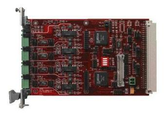
The Prizm RS-422 board provides six independent RS-422 channels that can support at least 10Megabits per second (Mbps). Each channel uses its own Prizm high-speed serial data channel and is not multiplexed with the other channels. The first four channels support only RS-422 (4-wire fullduplex connection) while channels 5 and 6 can be configured for either RS-422 or RS-485 (2-wire half-duplex connection) operation.
