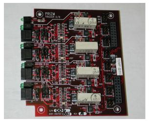
The Prizm Trigger Interface Daughtercard provides four channels of Input or Output selectable interface for use with most Acoustic Responder channels. This board is meant for use as a daughter-card on the standard PRIZM Submux1 or Submux2 motherboard. Refer to the Submux1 or Submux II manual for a description of those particular cards and the standard data daughtercards.
