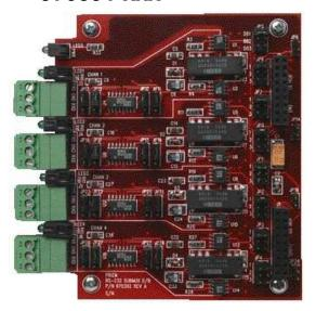
The Prizm 4-channel RS-232 Daughter board supports 4 independent, optically isolated RS-232 serial data channels, when plugged onto a Submux motherboard. Up to a total of 3 daughter boards may be stacked on one motherboard. The maximum data rate that this board supports is 115Kbaud. This board can be intermixed with the 4-channel RS-485/ 2 channel RS-422 Daughter board.
