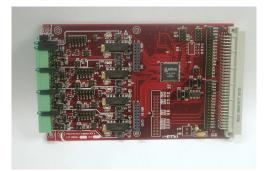
The Prizm RS-422 / 485 Sub-multiplexer (Submux2) motherboard provides four RS-422 or RS-485 channels that are multiplexed onto a single Prizm high-speed serial data channel. Motherboard channel selection of RS-422 or RS-485 can be simply done by selecting a few jumpers and can be accomplished on a channel-by-channel basis for mixed data applications. With the addition of up to three additional pluggable daughter boards, a total
