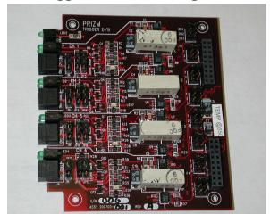
The Prizm Trigger Interface Daughterboard provides four channels of electrically-isolated digital Input or Output for use with most Acoustic Responder channels. This board is meant for use as a daughterboard on the standard PRIZM Submux or Submux2 motherboard. Refer to the Submux or Submux2 manual for a description of those particular boards and the standard data daughterboards.
