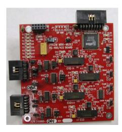
The Mini-Mux 2 RS-422/485 daughterboard provides the user with an additional four independent RS-422 or RS-485 serial data channels. Each channel can also be independently configured for either RS-422 (4-wire) or RS-485 (2-wire) communications. Each channel is optically isolated, self-powered and transient protected.
